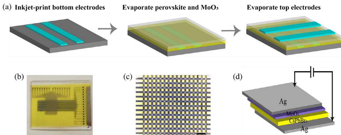
**Figure 1.** a) The schematic fabrication process of the inorganic perovskite memory array through all-vacuum-deposited processes. b) The photograph of the as-fabricated memory array on glass. c) The optical microscopy image of the memory cells (scale bar, 1 mm). d) The schematic structure of a single memory cell.
