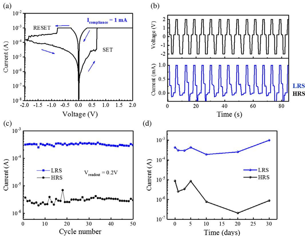
**Figure 2.** a) The current–voltage ( $I$ – $V$ ) curve of the perovskite memory devices. b) Current responses during write-read-erase pulse cycles (specifically, 2 V to write, 0.2 V to read, 2 V to erase, and 0.2 V to read). c) The cycle endurance test result. d) The stability of fabricated memory devices stored in an ambient condition.
