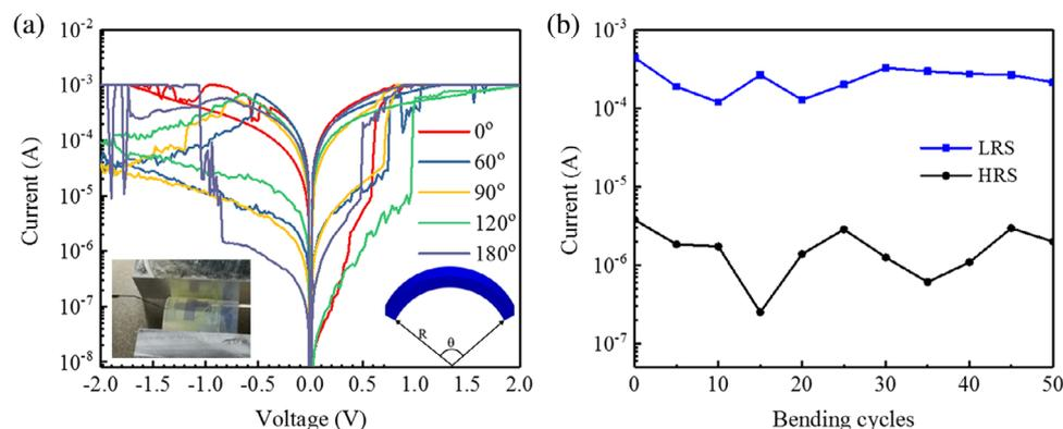
**Figure 4.** The bending performance of flexible perovskite memory devices. a)  $I$ - $V$  curves measured at various bending angles. The inset photographs show the measurement setup and the schematic illustration of the central angle ( $\theta$ ) for the flexible device under bending. b) The currents of flexible devices in LRS and HRS after different bending cycles.
