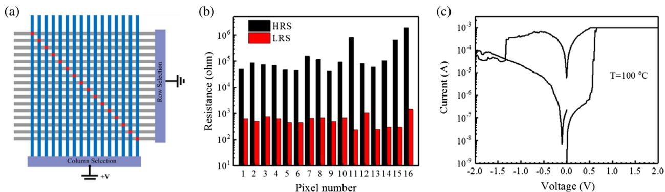
**Figure 5.** Reliable RS properties of the perovskite memory array. a) The schematic illustration of testing 16 memory cells on the diagonal line. b) The resistances of 16 memory cells in HRS and LRS. c) The  $I$ - $V$  curve of one memory cell measured at an elevated temperature of 100 °C.
