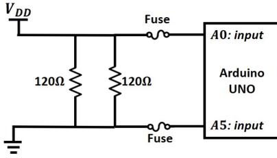
Fig. 14: Test circuits for checking that the Arduino board can measure the voltage with the fuses.
