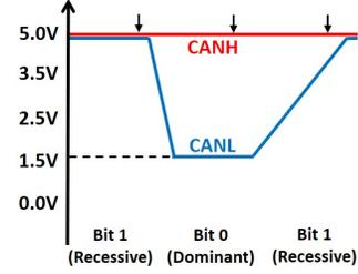
Fig. 9: Voltages of CAN bus under the forced retransmission attack when  $V_{attack,H}$  is set to 5.0V. When a recessive bit is transmitted right after a dominant bit, the transition time of the CANL's voltage level increases. Hence, a receiving ECU may determine a dominant bit since  $V_{Diff}$  is greater than 0.9V when it samples the CAN bus at the instances indicated with the black arrows facing downward.
