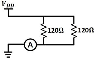
Fig. 16: Test circuit to emulate the voltages of the CAN bus under the overcurrent attacks. We measure the current that flows to the ground, and  $V_{DD}$  is set to 3.5V in the passive overcurrent attack and 5.0V in the active overcurrent attack.
