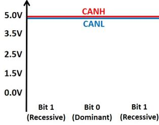
Fig. 7: Voltages of CAN bus under the DoS attack. Since  $V_{attack,L}$  is set to 5.0V, both CANH and CANL become 5.0V, which represents a recessive bit.
