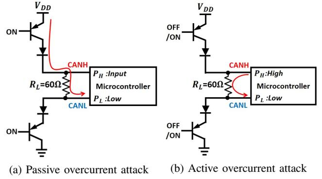
Fig. 5: Circuit diagrams under the overcurrent attacks. The red curve indicates the current in each overcurrent attack. (a) In the passive overcurrent attack, the current flows from  $V_{DD}$  to  $P_L$  when a dominant bit is transmitted. (b) In the active overcurrent attack, the current flows from  $P_H$  to  $P_L$  regardless of the bits.
