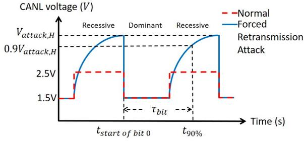
Fig. 10: Voltage of CANL under the forced retransmission attack. The bit length time  $\tau_{bit}$  is defined as the sum of duration of the dominant bit and the transition time. Compared with the voltage characteristics of the normal operation (dashed red line), the voltage of CANL needs to be pulled up to  $V_{attack,H}$  and the transition time increases (solid blue line).
