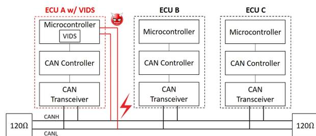
Fig. 1: General architecture of VIDS. VIDS is implemented as software code at ECU A’s microcontroller. The microcontroller of ECU A is directly connected to the CAN bus via two wires (two red lines). If ECU A is compromised, the adversary can launch voltage-based attacks using the directly connected wires.
