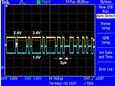
Fig. 15: Voltages of CANH (in yellow) and CANL (in blue) during the normal message transmission.
