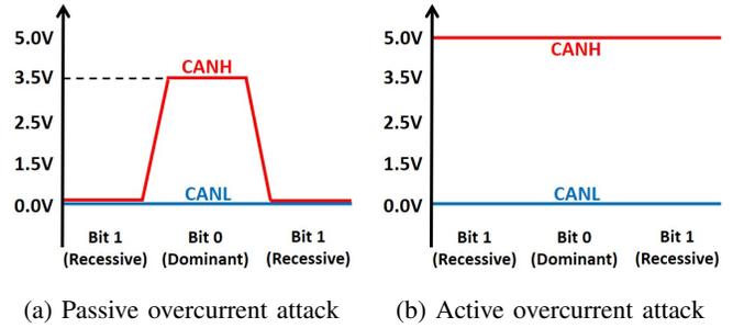
Fig. 6: Voltage behavior of CANH and CANL under the overcurrent attacks. (a) In the passive overcurrent attack, the maximum voltage difference between CANH and CANL is 3.5V when a dominant bit is transmitted. (b) In the active overcurrent attack, the voltage difference is always 5.0V.
