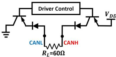
Fig. 4: The schematics of the Microchip MCP2551 CAN transceiver, which is composed of two BJTs and two diodes. The driver control turns off the BJTs when transmitting a recessive bit and turns them on when transmitting a dominant bit. The impedance  $R_L$  between CANH and CANL is  $60\Omega$  since two  $120\Omega$  termination resistors are connected in parallel.
