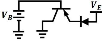
Fig. 12: Test circuits for measuring current in the DoS attack.
