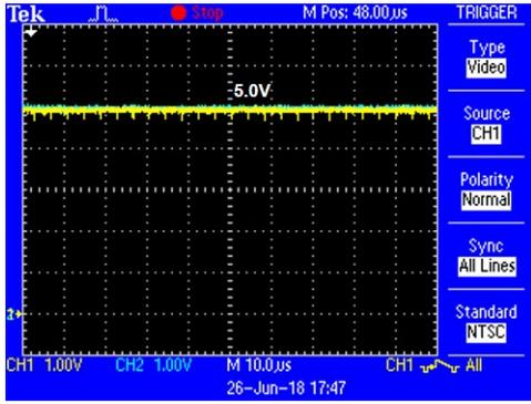
Fig. 18: Voltages of the CAN bus when the DoS attack is successfully launched by ECU A.  $P_L$  is set to the high voltage output mode that can generate 5.0V.
