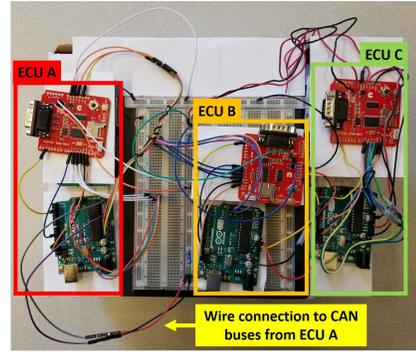
Fig. 13: The CAN bus testbed. The microcontroller of ECU A is connected to CANH and CANL via two wires. ECU A is compromised and launches the proposed voltage-based attacks. ECU C transmits messages every 1 second, and ECU B logs the received messages.
