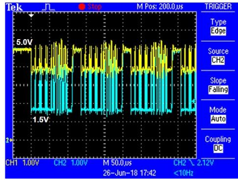
Fig. 22: Voltages of the CAN bus for  $V_{attack,H}=5.0V$ . The forced retransmission is successfully launched by ECU A. The same voltage waveform is repeated every  $132\mu s$  which indicates the message retransmission.
