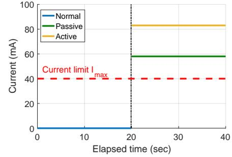
Fig. 17: Current measured in the test circuit under the overcurrent attacks. Before the attacks occur, the current is 0mA. However, after the attacks, the current greater than  $I_{max}$  (i.e., 40mA.) flows to the ground in both attacks which may damage the microcontroller.
