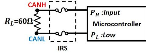
Fig. 11: Structure of the proposed hardware-based IRS that comprises two fuses connected to each analog pin of the microcontroller.
