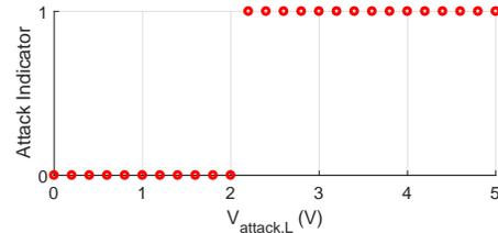
Fig. 20: The minimum value of  $V_{attack,L}$  that leads to a successful DoS attack. The attack indicator is either 0 meaning a failure of the attack or 1 meaning a success of the attack. The DoS attack becomes successful from  $V_{attack,L}=2.2V$ .
