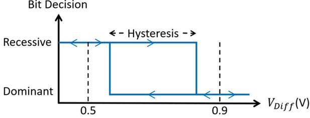
Fig. 8: Bit decision criteria of the Microchip MCP2551 CAN transceiver. The differential input hysteresis may not be identical among the CAN transceivers. A CAN transceiver can determine a dominant bit if  $V_{Diff}$  is typically larger than 0.9V and a recessive bit if  $V_{Diff}$  is less than 0.5V.
