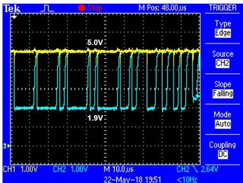
Fig. 24: Voltages of the CAN bus for  $V_{attack,H} = 5.0V$  at which the forced retransmission attack becomes successful using the power supply.
