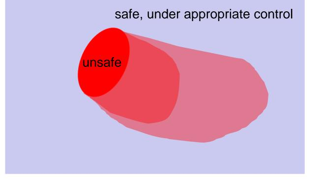
Safety Property can be encoded as a condition on the system's reachable set of states
