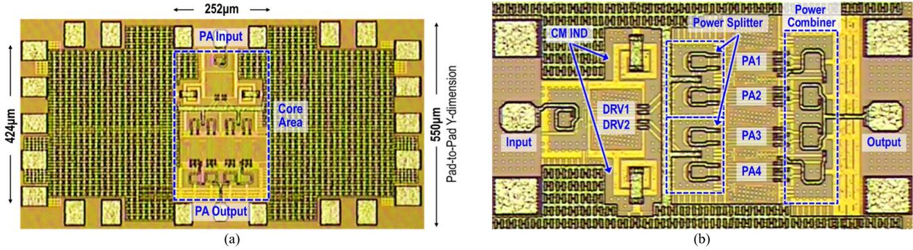
Fig. 11. Die photographs of the PA in 16-nm FF CMOS. (a) PA test chip including pads. (b) Zoomed-in view of PA core (with 90° counter-clockwise rotation).
