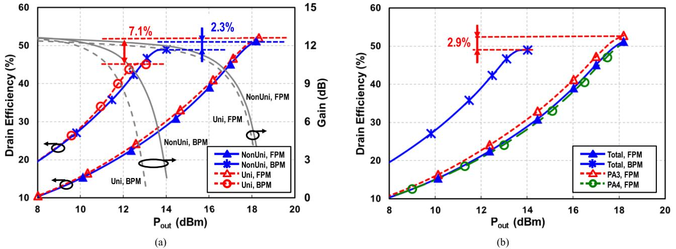
Fig. 6. Large-signal simulation results. (a) DE (and gain) comparison between non-uniform and uniform power combining in FPM and BPM. (b) Further breakdown in DE for non-uniform power combining.
