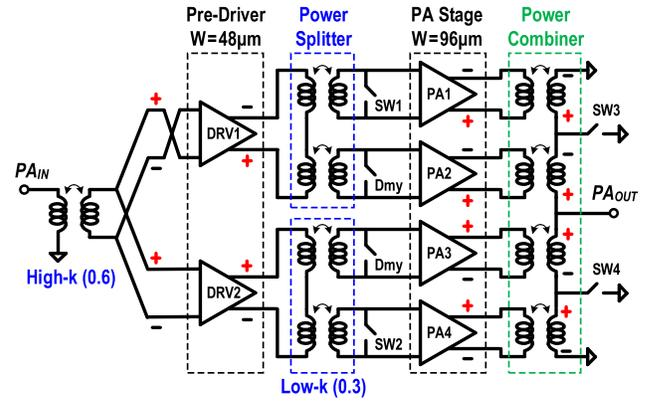
Fig. 2. Two-stage PA architecture with a reconfigurable two-/four-way series-parallel power combiner. Polarity of each gain stage is shown.
