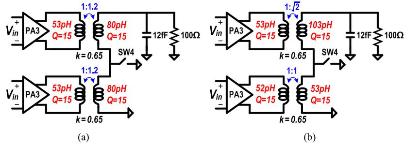
Fig. 5. Simplified half-circuit schematic with a two-way series combiner for comparison between (a) uniform and (b) non-uniform power combining.
