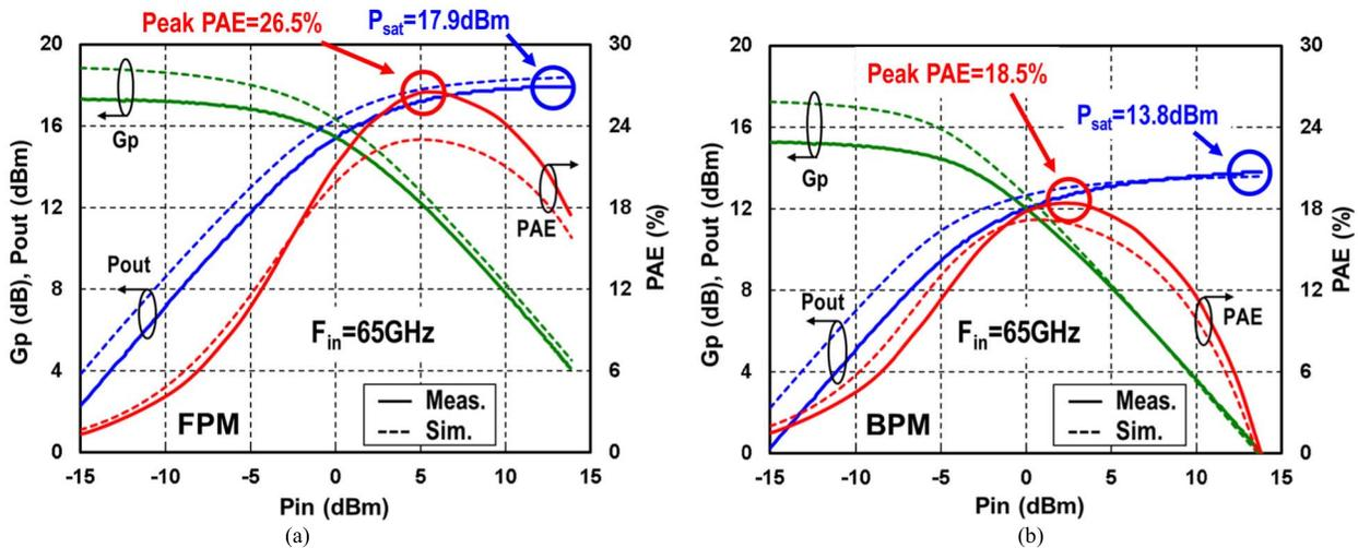
Fig. 13. Measured versus simulated large-signal performance ( $G_p$ ,  $P_{out}$ , and PAE) versus  $P_{in}$  in (a) FPM and (b) BPM at 65 GHz.
