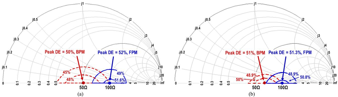
Fig. 7. Load-pull simulations of DE show how  $r_{opt}$  shifts between two modes for (a) uniform and (b) non-uniform power combining.
