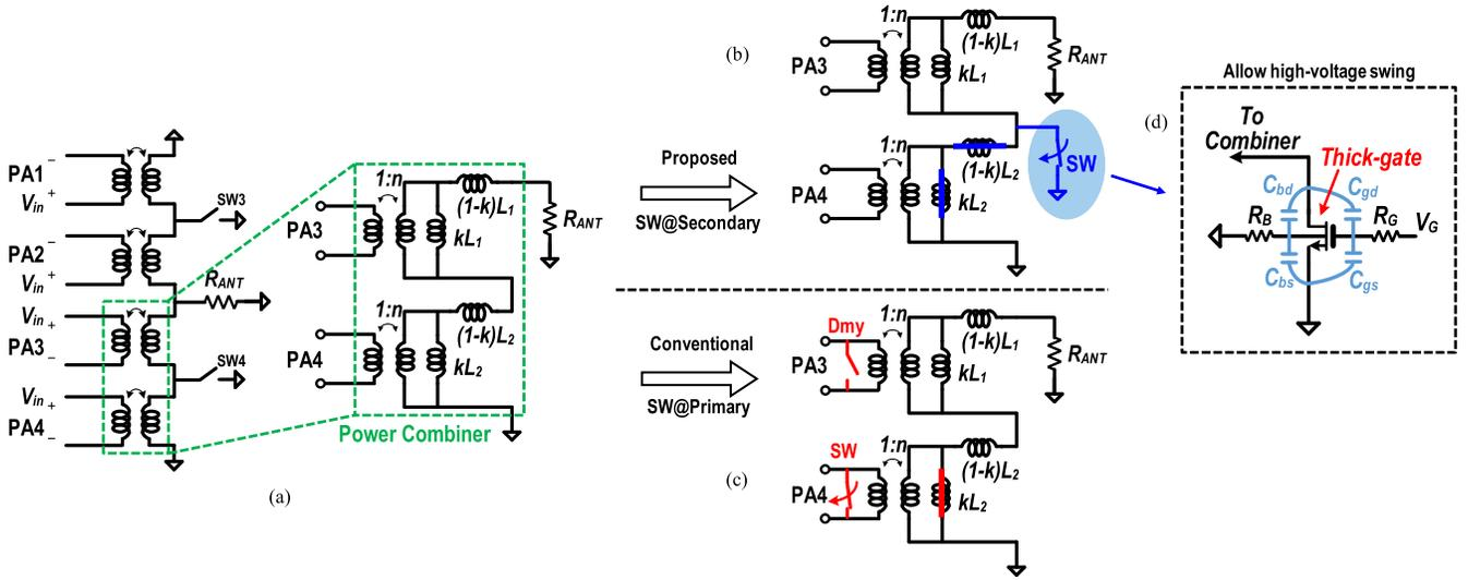
Fig. 8. Comparison of implementing the switching scheme. (a) Power combiner model. (b) Proposed switch placement at secondary side. (c) Conventional switch placement at transformer's primary. (d) Thick-oxide switch architecture which accommodates a high-voltage swing.
