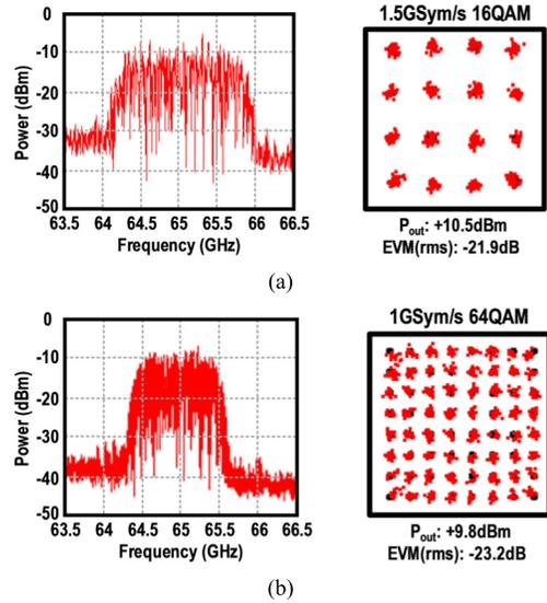
Fig. 16. Measured spectrums and constellations for (a) 1.5 GSym/s 16-QAM and (b) 1 GSym/s 64-QAM at 65 GHz.
