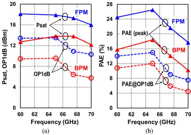
Fig. 15. Large-signal measurements in FPM and BPM across 60–70 GHz. (a)  $P_{sat}$  and  $OP_{1dB}$ . (b) Peak PAE and PAE at  $OP_{1dB}$ .
