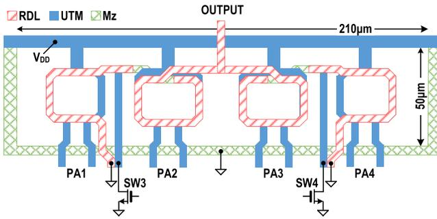
Fig. 9. Two-/four-way series-parallel power combiner with non-uniform turns ratios of (from left to right) 1:1, 1:  $\sqrt{2}$ , 1:  $\sqrt{2}$ , and 1:1.
