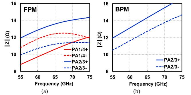
Fig. 10. Magnitude of impedances seen from the two single-ended outputs (+/-) of PA1-4 in (a) FPM and (b) BPM.
