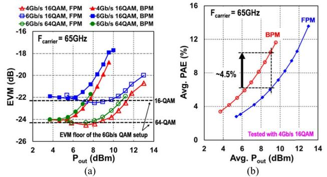
Fig. 17. Measurements of modulated signals. (a)  $EVM_{rms}$  versus  $P_{out}$  for various modulations. (b) PAE versus  $P_{out}$  with 4 Gb/s 16-QAM modulation in FPM and BPM.
