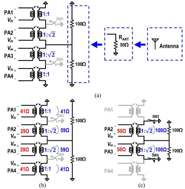
Fig. 4. Conceptual diagram of non-uniform power combining. (a) Combiner model. The impedances seen from each PA stage in (b) FPM and (c) BPM.
