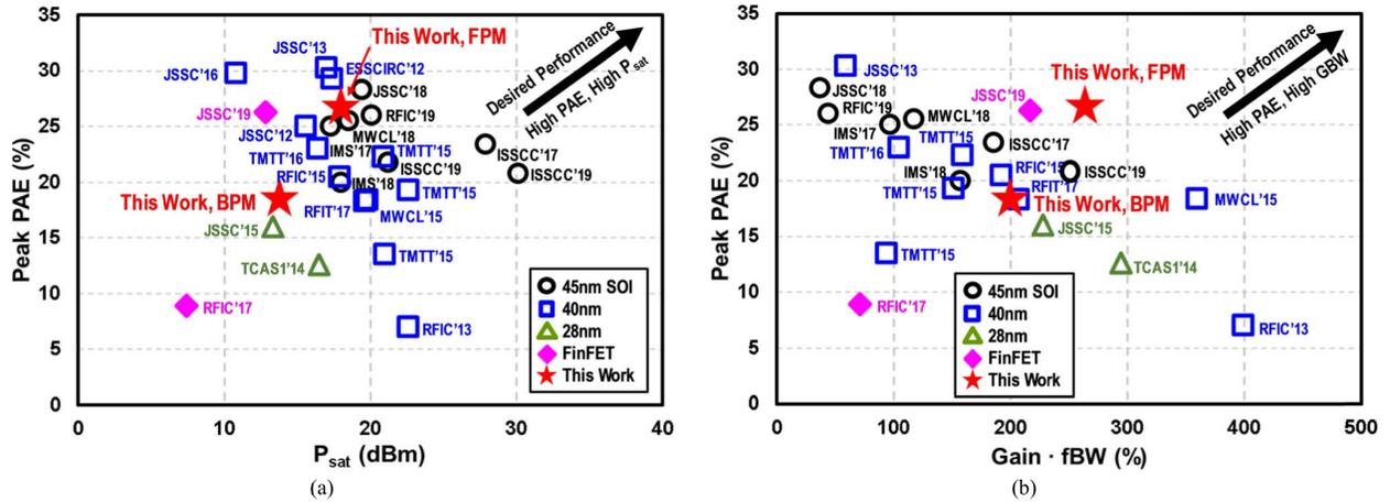
Fig. 18. Performance comparison of mm-wave (50–75 GHz) PA prior art. (a) Peak PAE versus PA  $P_{\text{sat}}$ . (b) Peak PAE versus gain-fBW product [38].
