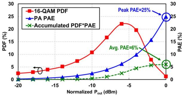
Fig. 1. Conceptual diagram illustrating PA average efficiency. The 16-QAM PDF and PA PAE curves are depicted as functions of normalized PA  $P_{out}$ .
