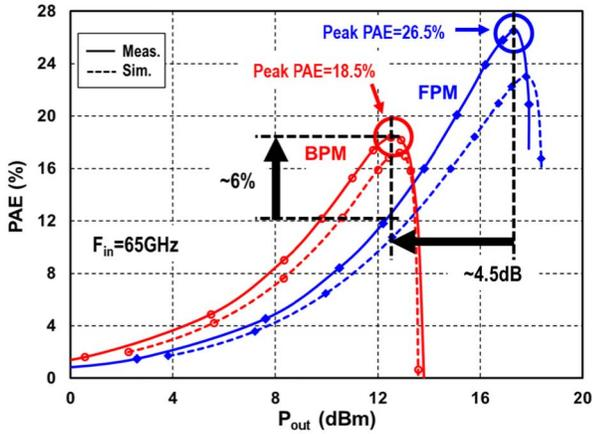
Fig. 14. Measured versus simulated PAE versus  $P_{out}$  in FPM and BPM at 65 GHz.
