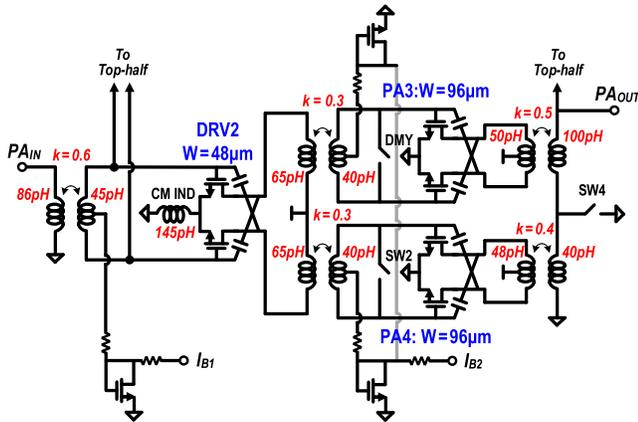
Fig. 3. Detailed transistor-level schematic for the bottom-half of the PA.
