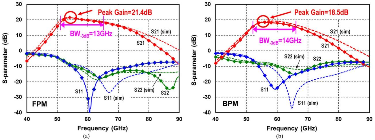
Fig. 12. Measured versus simulated S-parameters in (a) FPM and (b) BPM.
