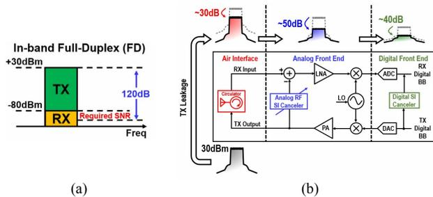
Fig. 10. SI cancellation in FD communication (a) SI cancellation requirement in a FD radio with TX output power of 27dBm and RX required sensitivity of -80dBm, (b) SI cancellation distributed in the RX chain.
