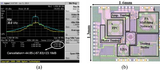
Fig. 3. (a) 4-port canceler (FPC) achieves -23dB cancellation using WCDMA modulated signal, (b) Die photo of TSMC 40nm CMOS chip, FPC shown center-left.
