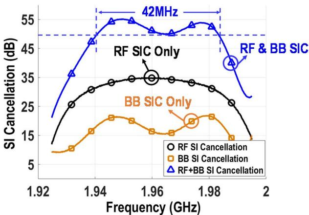
Fig. 12. Dual-injection path FD canceler block diagram (top), die photo (center), and measured SI suppression (bottom).
