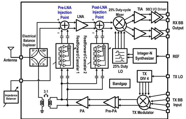
Fig. 14. Improved Dual-Injection Path Canceler with Electrical Balance Duplexer to allow both FD and FDD operation.
