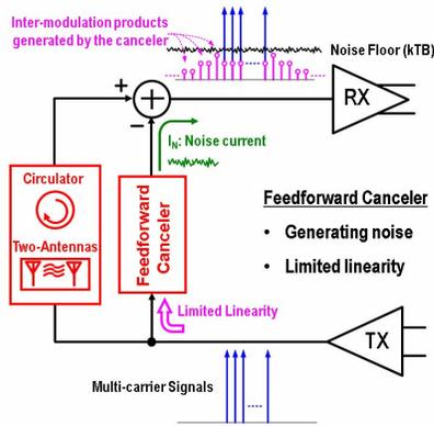
Fig. 1. Components used to improve TX-to-RX isolation. These include dedicated TX/RX antennas, a circulator with shared TX/RX antenna and feedforward cancellation paths.
