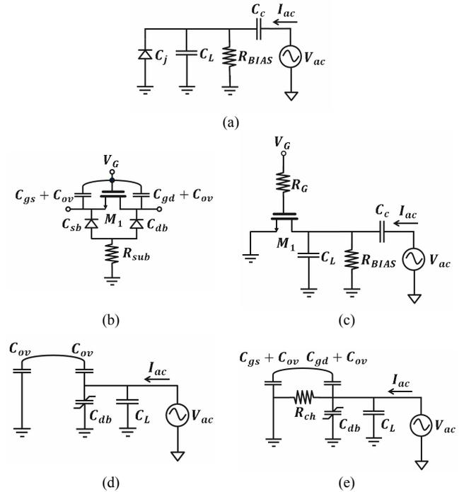
Fig. 7. (a) A test circuit for a simple diode; (b) Capacitances in a NMOS transistor; (c) A test circuit for a NMOS transistor as a switch; (d) The equivalent circuit when the switch is OFF; (e) The equivalent circuit when the switch is ON.
