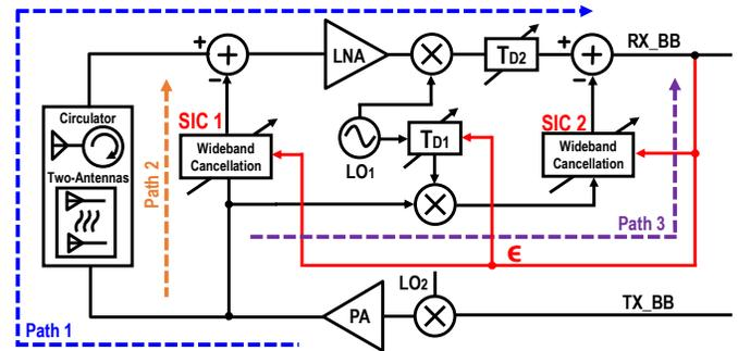
Fig. 11. Dual-injection path self-interference canceling architecture.
