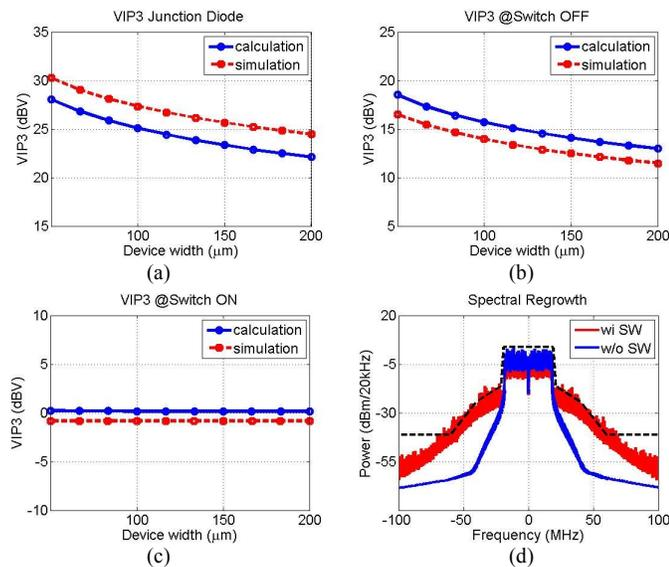
Fig. 8. The calculation and Spice simulation results of IP3: (a) Diode junction capacitance, (b) NMOS switch is OFF, (c) NMOS switch is ON; and (d) The spectral regrowth due to limited switch linearity.
