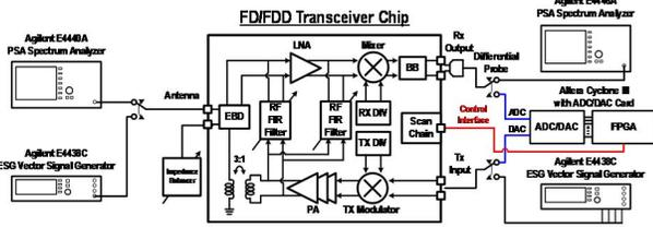
Fig. 15. Test setup which includes a FPGA board to emulate the digital baseband and perform real-time calibration.
