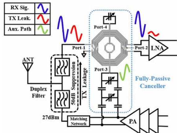
Fig. 2. An early implementation of an all-passive feedforward SI cancellation network.
