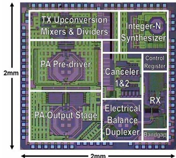
Fig. 13. Die photo of improved dual-injection path radio with EBD implemented in a 40nm TSMC CMOS process.
