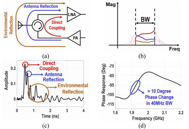
Fig. 9. Channel response of the leakage path (a) Multiple time delay paths of the leakage signal coupled from PA output to LNA input, (b) Frequency response for each time delay versions of the leakage signal, (c) Impulse response of a discrete circulator from Meca Electronics, (d) Phase response of the measured discrete circulator.
