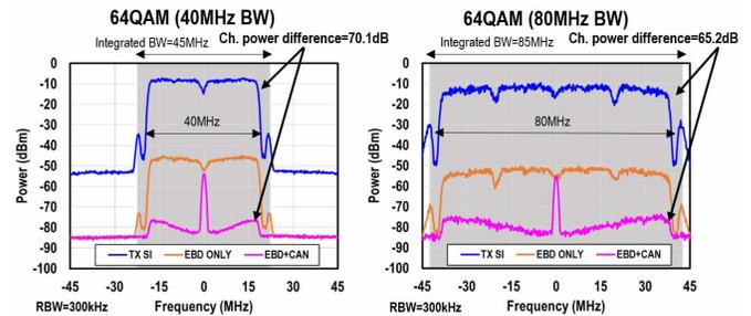
Fig. 16. Measured SI cancellation using IEEE 802.11 (OFDM multicarrier) sample packets with different bandwidths.
