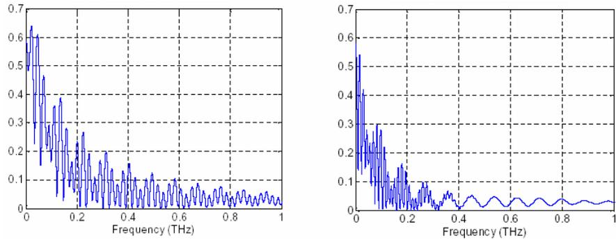
Fig. 3: Reflection in terahertz range. Left: no explosive, Right: explosive present
