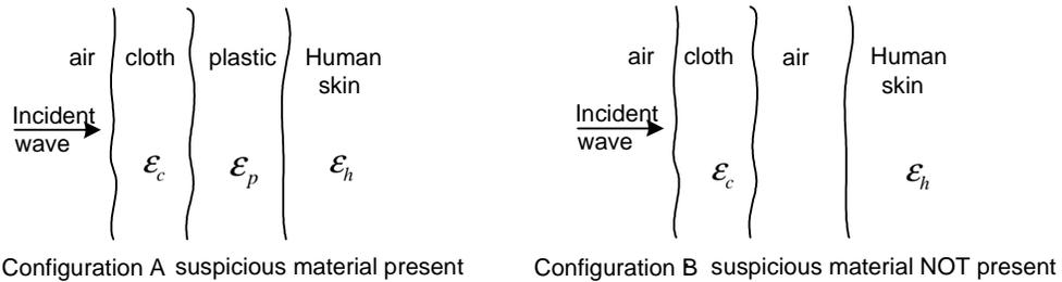
Fig. 1: Multi-layer media model for hidden object underneath clothing
