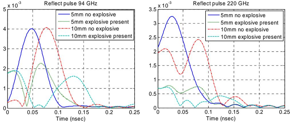
Fig. 5: Effect of thickness of the bomb layer.
