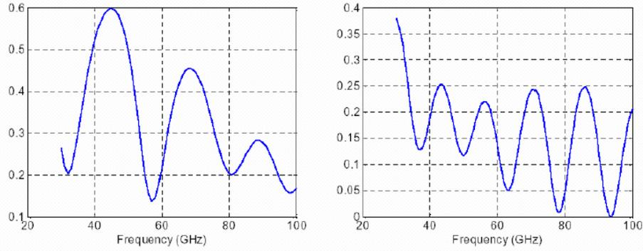
Fig. 2: Reflection in MMW range. Left: no explosive, Right: explosive present
