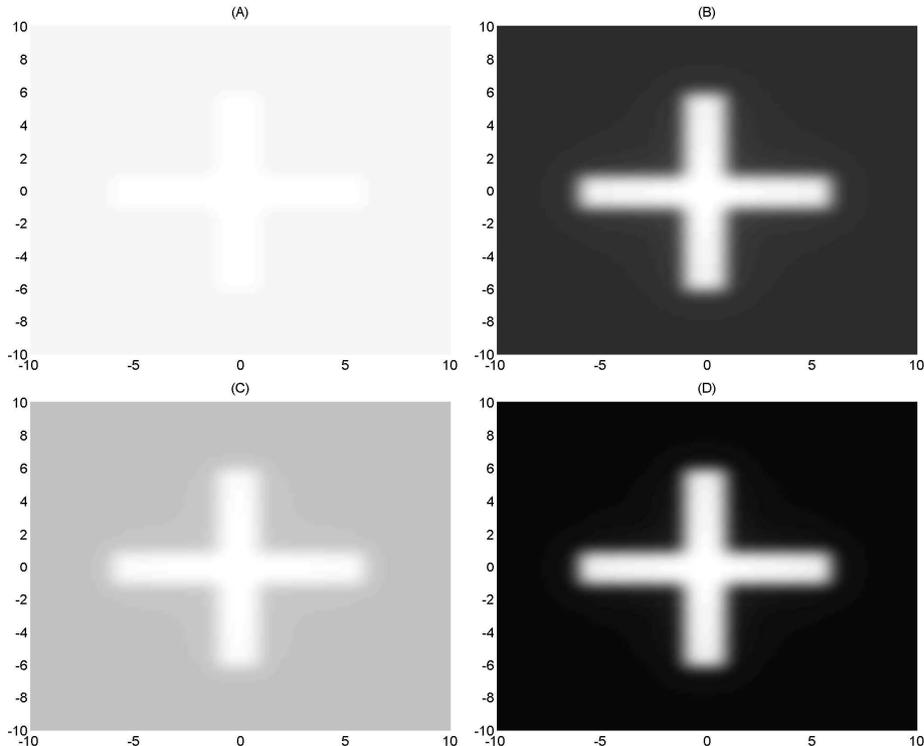
**Figure 6.** The linear polarized cross images through random media of optical depth 30 using (A) co-polarized wave, (B) CPIS, (C)OAIS, and (D) 1 MHz photon density waves. The angular sizes are in microradians.
