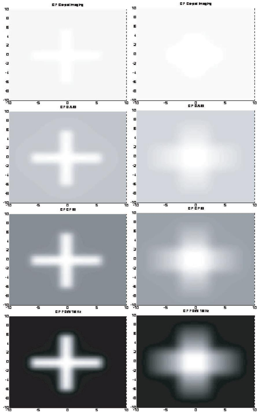
**Figure 7.** Field of view effect to CW imaging. Left column shows FOV of 1 microradian and right column shows FOV of 5 microradians. Top row is co-polarized imaging, second row is OAIS, third row is CPIS, and bottom row is photon density waves
