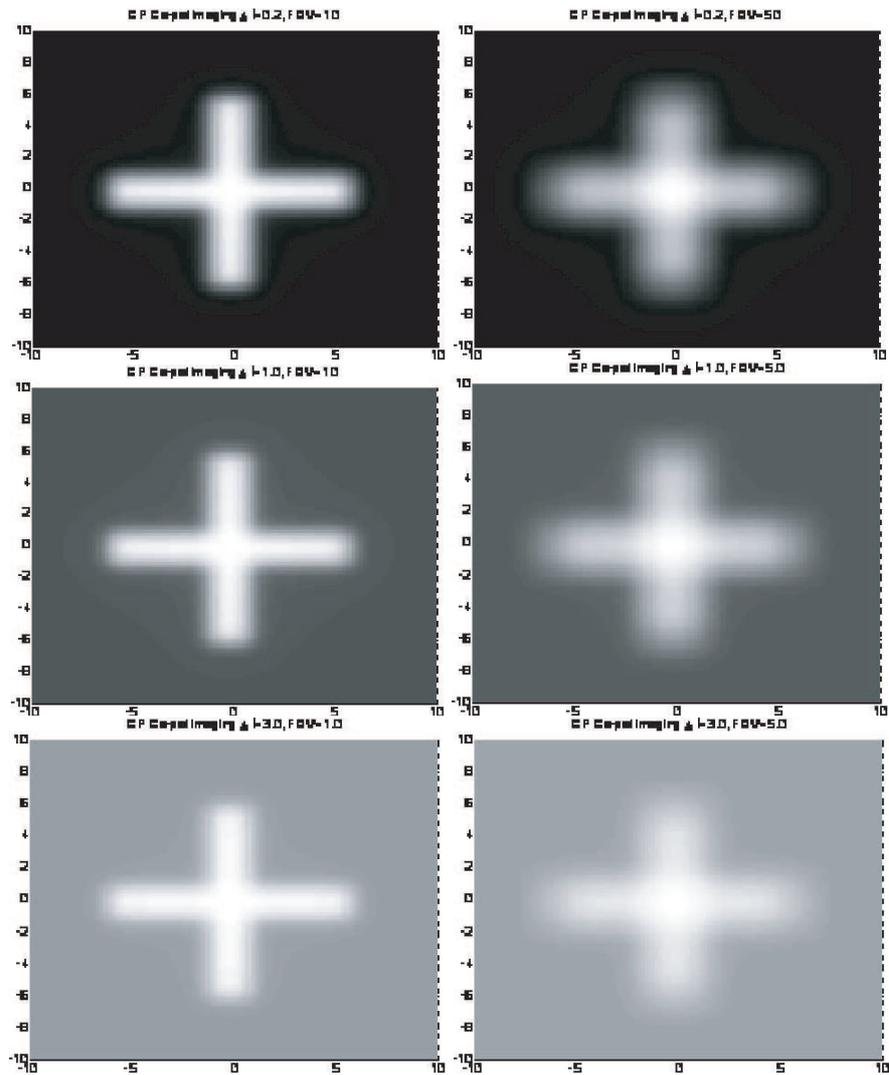
**Figure 8.** Field of view effect to CW imaging. Left column shows FOV of 1 microradian and right column shows FOV of 5 microradians. Top row is time-gating is 0.2, second row is time-gating of 1, and the bottom row is time-gating of 3. The time unit is normalized to  $L/c$
