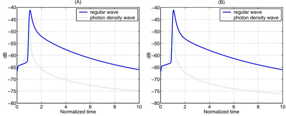
**Figure 2.** Forward pulse CW wave and 10 MHz photon density wave ( $0.68^\circ$ ) as a function of time (A) Circular polarization and (B) Linear polarization.
