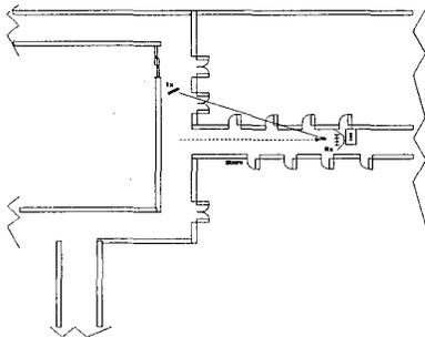
**Figure 3:** Plan view of the area of the EE building used for the tests. The transmitter is positioned at about  $18^\circ$  the antenna boresight. The distance from Tx to Rx is 21 m.
