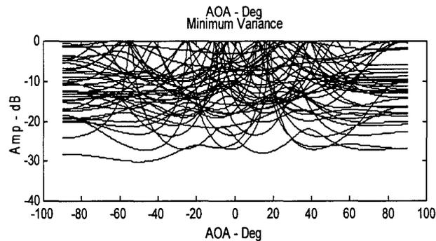
**Figure 4:** Superposed angular spectra for each individual frequency in the hallway experiment. Note the apparently random AOA for each incident temporal frequency. Each spectrum is obtained using 40 points in the frequency range 0.9-1 GHz. The plot is meant to show the difficulty in obtaining an AOA estimate from individual estimates alone.
