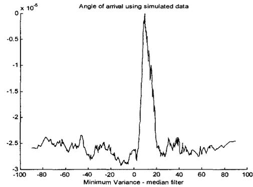
**Figure 2:** Using data obtained from the simulated EE building, we show the AOA estimation results. In this case there is no problem discerning the correct AOA at 18 degrees.
