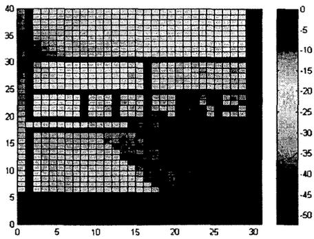
**Figure 1.** Simulation of EM wave propagation inside a building. One Transmitter is located at the top left. Black lines are dielectric walls.
