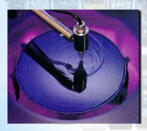
The photoresist is the chemical that is spun on top of the substrate ... and determines whether the process is:
