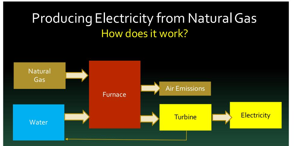
In the Boiler Power Plant, natural gas is converted to electricity through the Rankine cycle:
