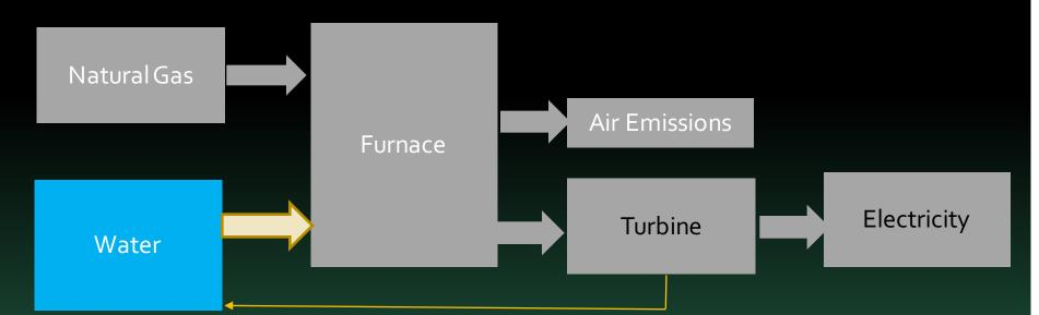
Water is fundamental to burning natural gas for power in a boiler style power plant as it is heated into steam and used to turn the turbines that generate electricity. Water is withdrawn to support the electricity production cycle and consumed through evaporation.
