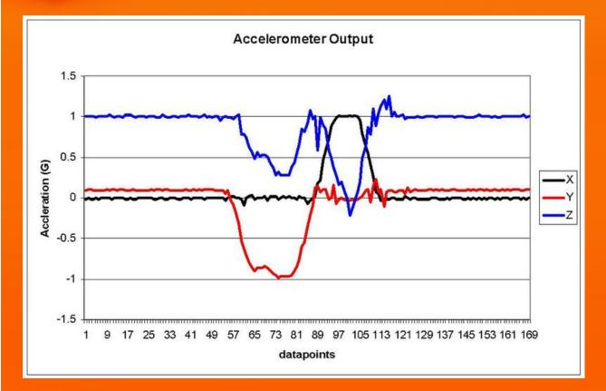
The three axes of an accelerometer may be used to detect the orientation of a tennis racquet (to which they are attached) within a certain # of degrees of accuracy.
