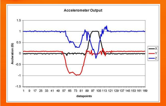
Alternatively, the three axes of an accelerometer may be used to detect whether or not the tennis racquet is in the proper posture for a successful swing.
