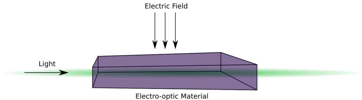
*Figure 6.1 - Light traveling through an electro-optic material.*
