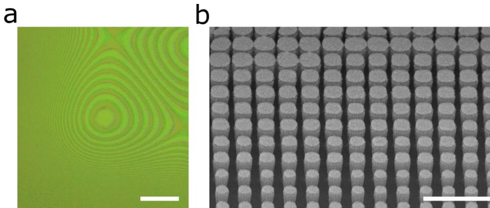
*Fig. 4.2. Images of the fabricated meta-optics. The meta-optics was sputter coated with gold-palladium alloy to ensure charge dissipation a) Optical image (Scale bar is  $150\ \mu\text{m}$ ). b) Scanning electron micrograph; scale bar of  $1\ \mu\text{m}$  taken at  $45^\circ$  to the normal.*
