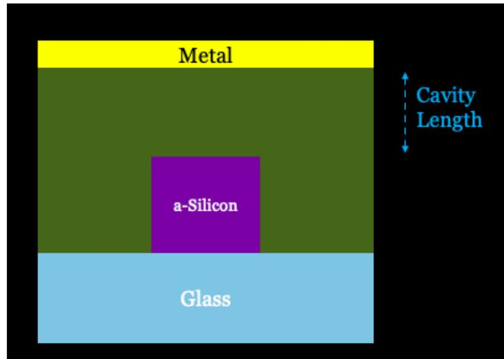
Figure 6.5 – Geometry cross section of a single grating
