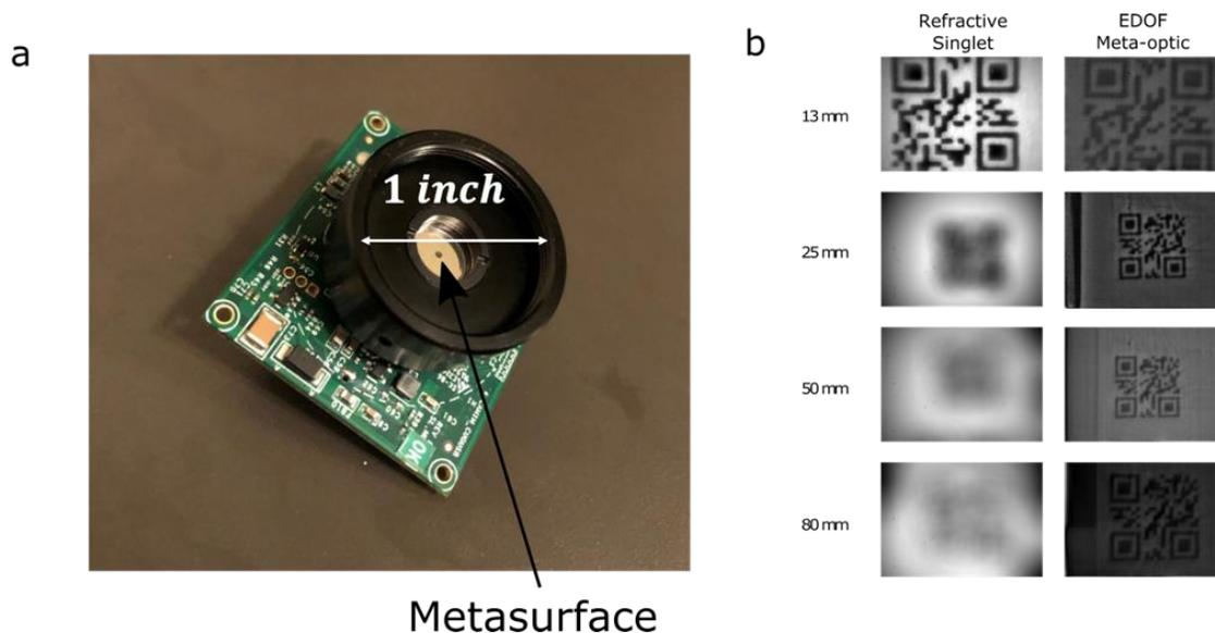
*Fig. 4.5. a) Metasurface optic integrated with E-consystems camera module. b) Pictures of QR code object at differing object lengths taken by a singlet refractive lens with focal length 6mm at F/2 (left) and by a singlet EDOF meta-optic with nominal focal length 5.6mm at F/2.8 (right). The 13mm and 25mm object distances used a 5mm × 5mm QR code. The 50mm object distance used a 10mm × 10mm QR code, and the 80mm object distance used a 30mm × 30mm barcode.*
