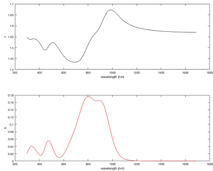
*Figure 6.4 EO polymer refractive index. Real (top) and imaginary (bottom) versus wavelength. Measured using ellipsometry*
