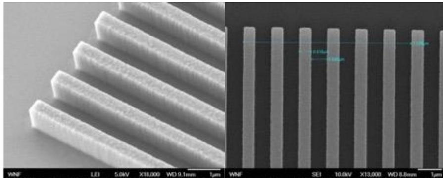
*Figure 6.8 - Si deposited on substrate post etch.*
