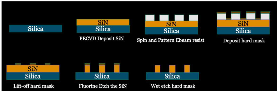
*Figure 3.1. Fabrication process flow for silicon nitride metasurface*
