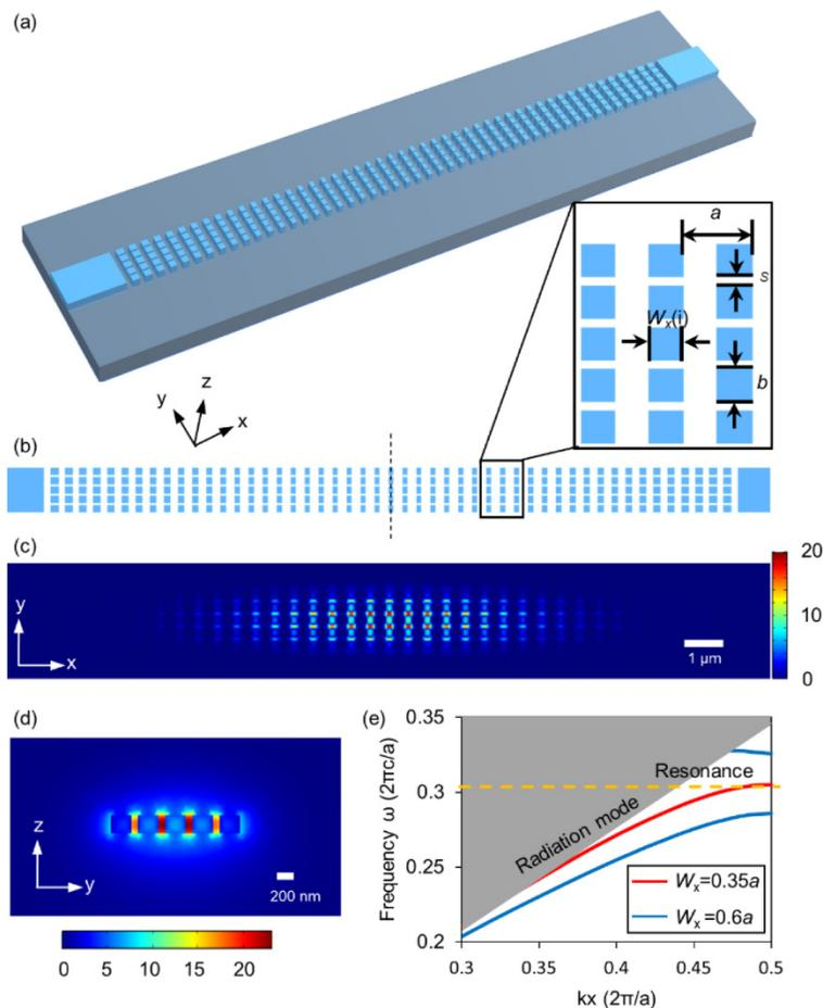
Fig. 1. (a) Schematics of the proposed Si MSPhC device; (b) Top view of the MSPhC device. Inset: zoom-in view of the framed part. (c)-(d) The electric field ( $|E|$ ) distribution from (c) top and (d) side taken at the center of the cavity simulated by 3D FDTD. (e) Simulated band structure of periodic multi-slot post cell (shown in the inset) with  $W_x = 0.35a$  (red lines) and  $W_x$
