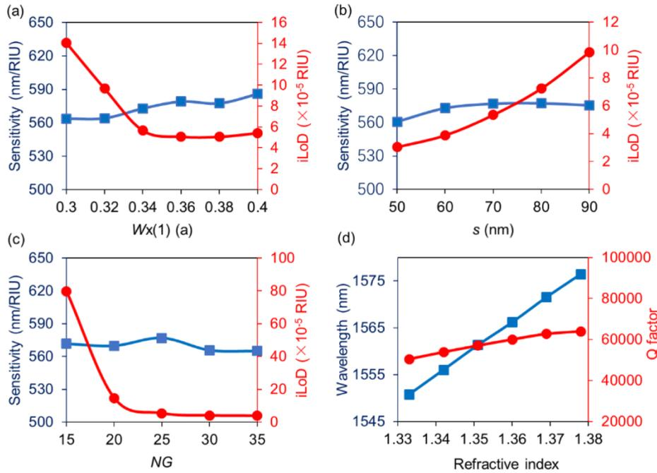
Fig. 2. Influence of (a)  $W_x(0)$ , (b)  $s$  and (c) number of Gaussian mirror segments ( $NG$ ) on the sensitivity and  $iLoD$  of multi-slot PhC cavity sensors; (d) Wavelength shift and variance of  $Q$ -factor over different background refractive indices. The sensitivity calculated in (a)-(c) is derived from the  $S = \Delta\lambda/\Delta n$  with the background refractive index around 1.333.
