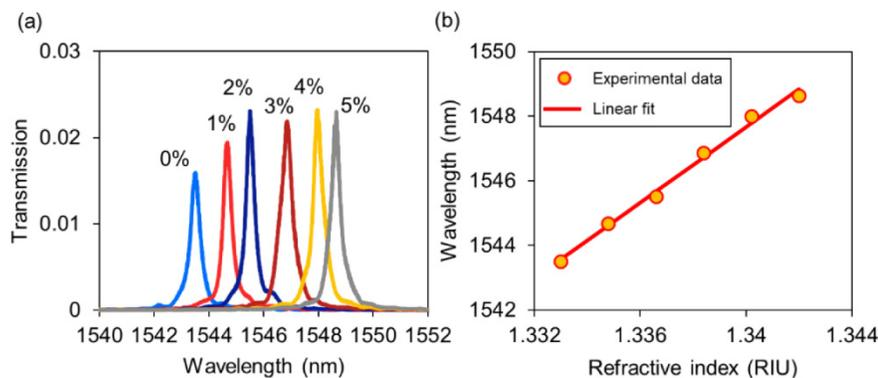
Fig. 4. (a) Measured transmission responses of the multi-slot PhC cavity immersed in the aqueous NaCl solution with different concentrations. (b) The resonant wavelength of the PhC cavity sensor as a function of the background refractive index. The sensitivity of the PhC cavity sensor is 586 nm/RIU by linear fitting.
