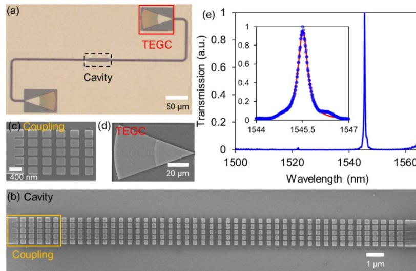
Fig. 3. (a) Optical image of the fabricated multi-slot photonic crystal nanobeam cavity. (b), (c) SEM of the device and the enlarged view of the coupling region connecting the strip/slot waveguides. (d) SEM of the GC. (e) Measured transmission spectrum of the MSPhC cavity in 2% NaCl solution. The inset shows the fit to Lorentzian lineshape for the resonance ( $Q \sim 4200$ ).
