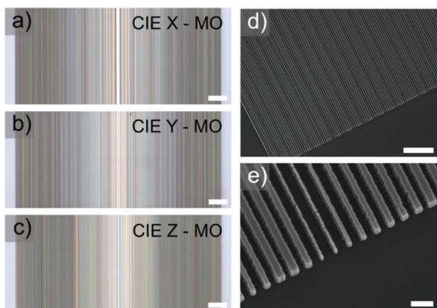
**Figure 3.** Design and fabrication of the CIE meta-optics (MO). Optical images of the CIE X, Y, and Z meta-optics are shown in (a), (b), and (c), respectively. The scale bars correspond to 100  $\mu\text{m}$ . Magnified SEM images of the Y meta-optic at an oblique angle are shown in (d) and (e). The scale bars in (d) and (e) correspond to 5  $\mu\text{m}$  and 500 nm, respectively.
