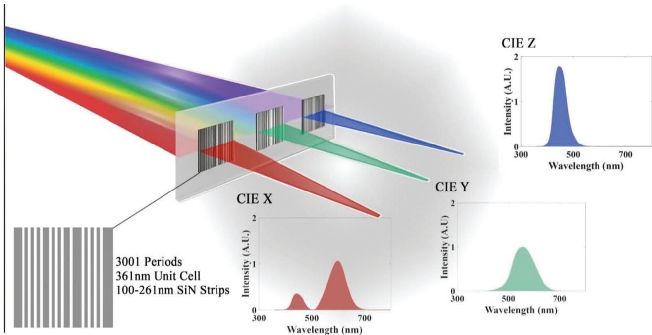
**Figure 1.** Schematic of the CIE XYZ meta-optics. Three separate 1D meta-optics focus light with a spectral response equivalent to the color matching functions of the CIE 1931 XYZ color space from left to right, respectively. The spectral responses are depicted for the respective color space functions.
