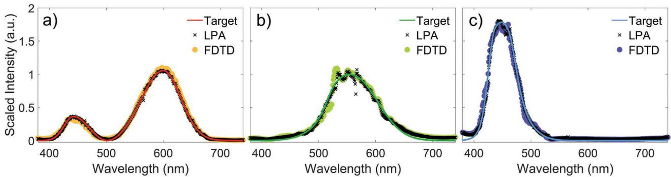
**Figure 2.** Verification of the optimization based on LPA for the a) CIE X, b) CIE Y, and c) CIE Z meta-optics. The design results under LPA are the first terms in the brackets of Equation (2) multiplied by  $f(\lambda_0)/c$ .
