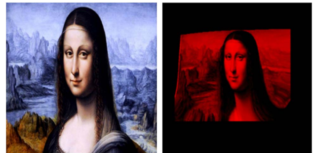
Fig. 3. Image simulation of the Mona Lisa in the NEV using Zemax. The left figure is the original image projected in the display. The right figure is the simulated image as seen by the person using the NEV.
