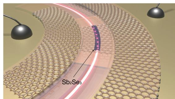
Schematics for electrically controlled phase-change-material integrated-photonic devices. Left: Tunable beam splitters using doped silicon PIN heaters. Center and right: Amplitude- and phase-programmable units with graphene heaters.
