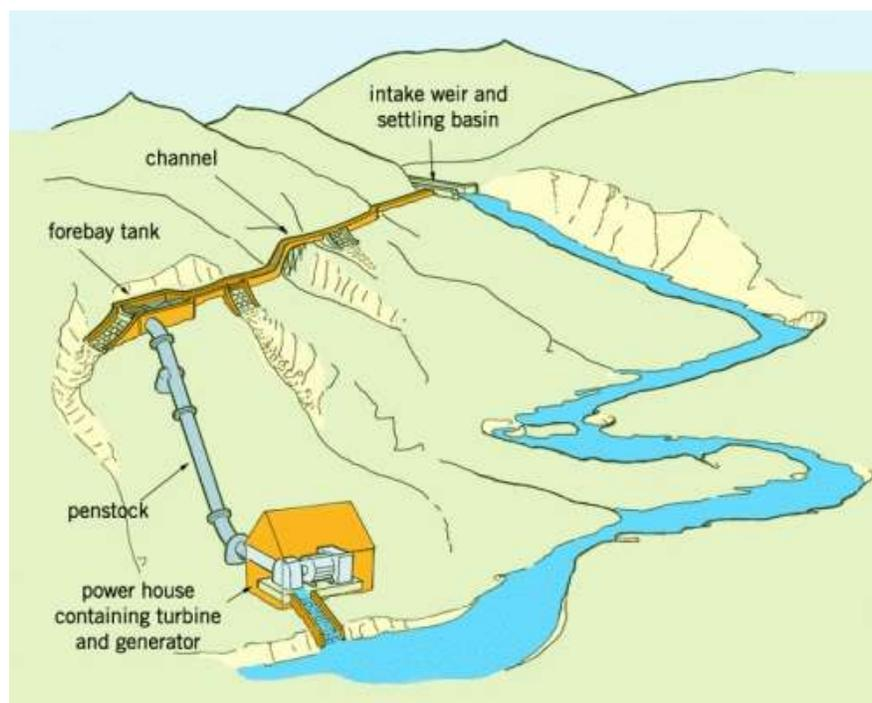
**Figure 3: Example small-scale run-of-river hydroelectric system [5]**
