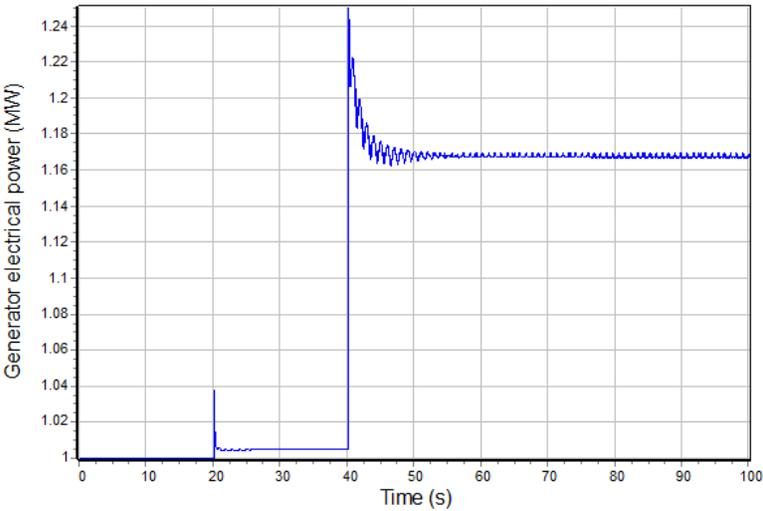
Figure 22: Generator electrical power output, 25% load increase (simulation 2)
