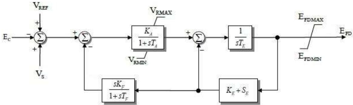
Figure 9: IEEE1A block diagram [20]
