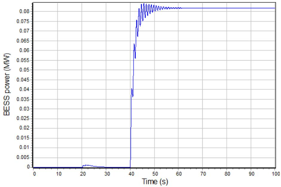
**Figure B4: BESS power, 25% load increase (simulation 2)**
