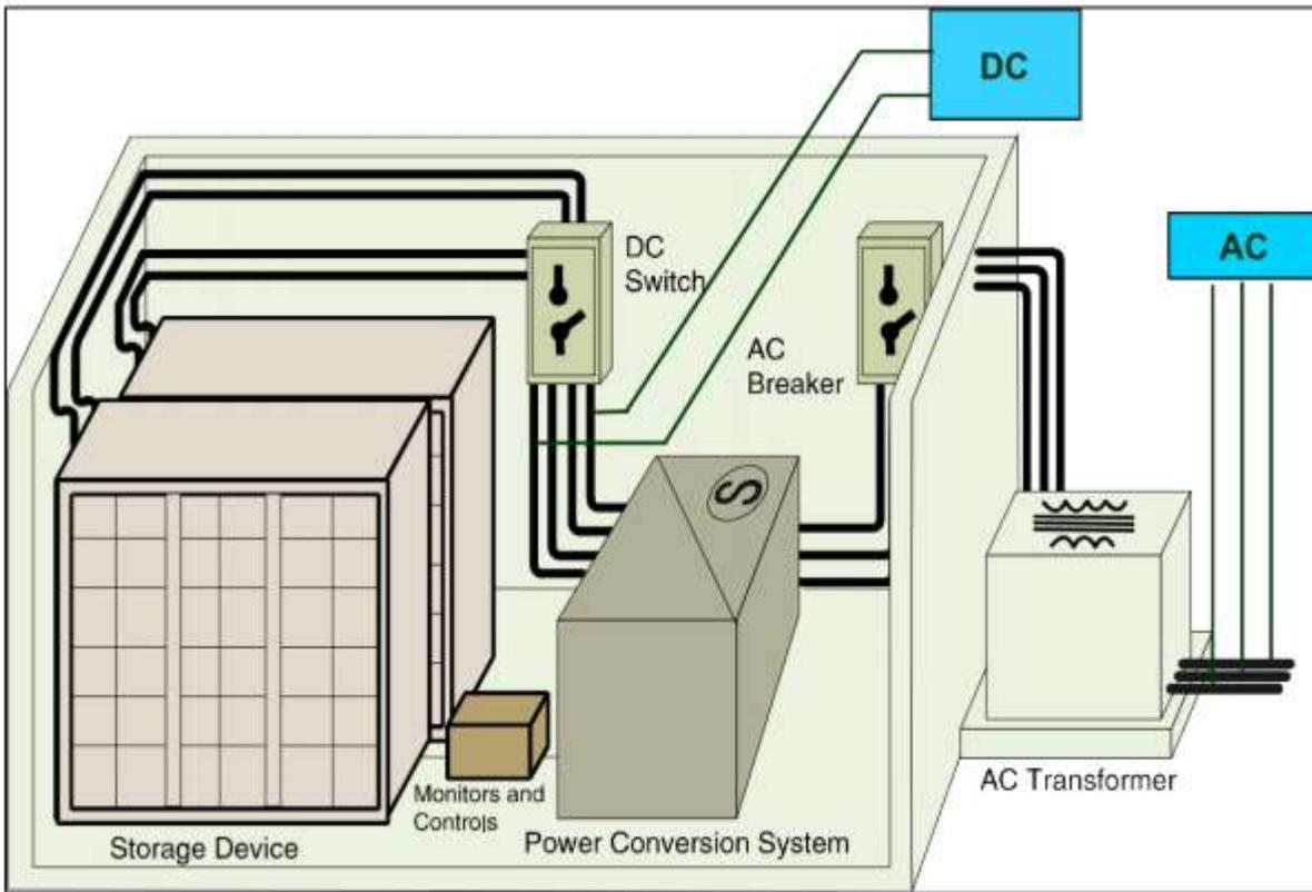
**Figure 2: Battery energy storage system schematic [1]**
