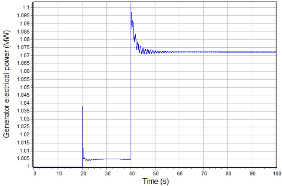
**Figure 18: Generator electrical power output with BESS  $K_{pg} = 1$**
