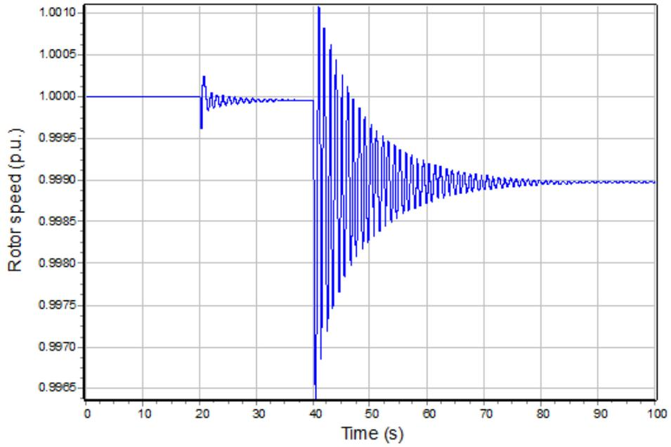
**Figure 26: Generator rotor speed, 0.5 MW base load (simulation 4)**
