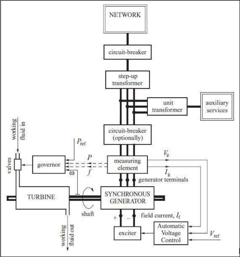
**Figure 8: Power generation system block diagram [11]**
