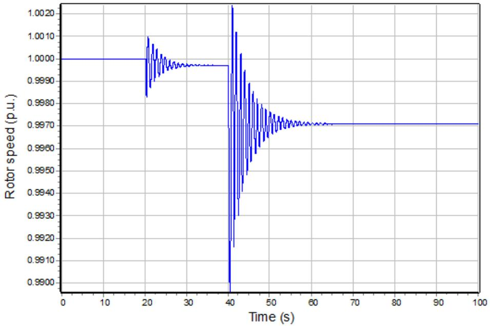
**Figure 27: Generator rotor speed, 1.5 MW base load (simulation 5)**
