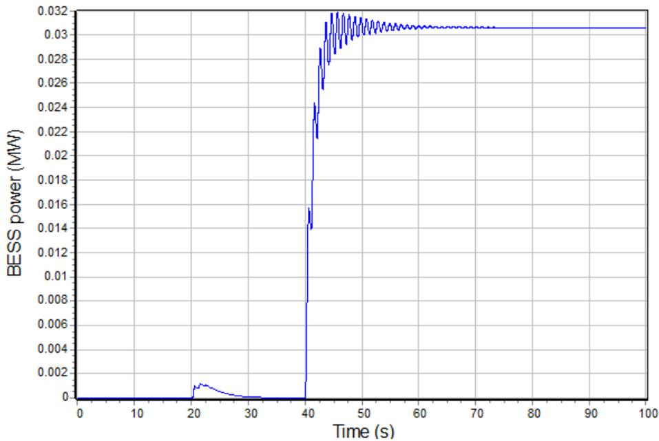
**Figure 20: BESS output with BESS  $K_{pg} = 1$**
