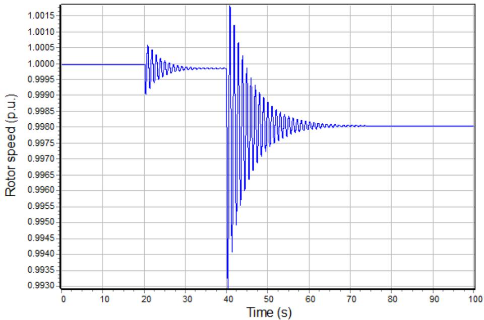
**Figure 19: Generator rotor speed with BESS  $K_{pg} = 1$**
