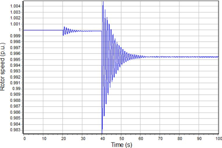
**Figure 23: Generator rotor speed, 25% load increase (simulation 2)**
