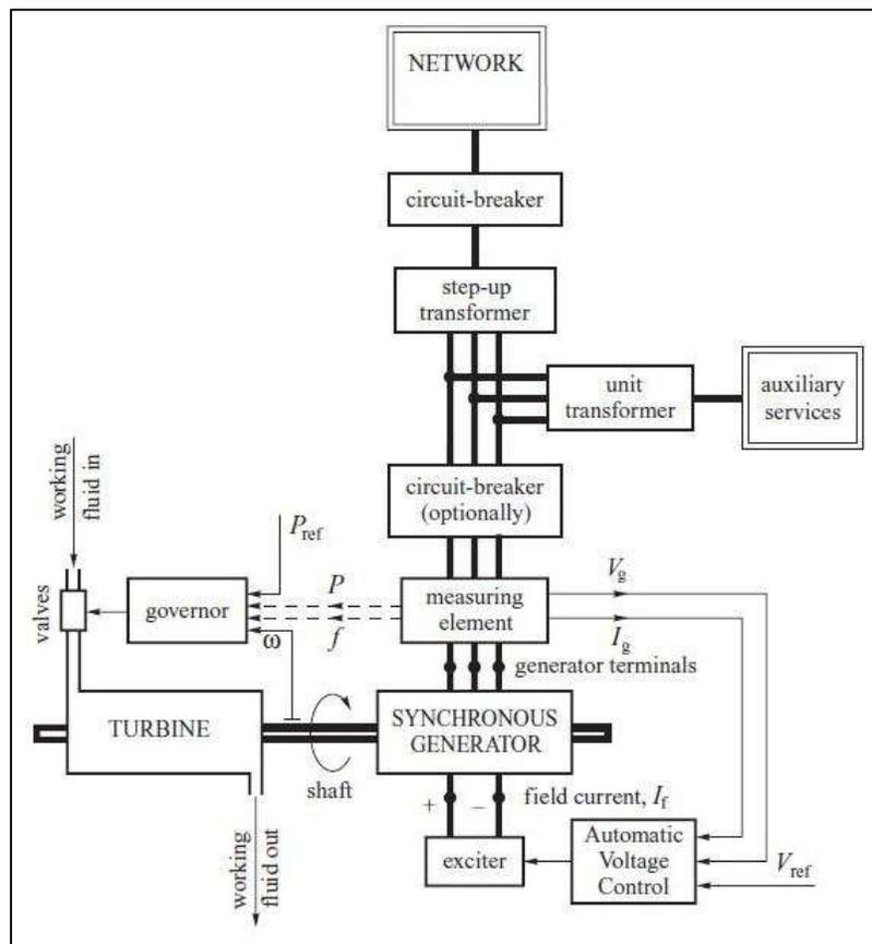
**Figure 8: Power generation system block diagram [11]**
