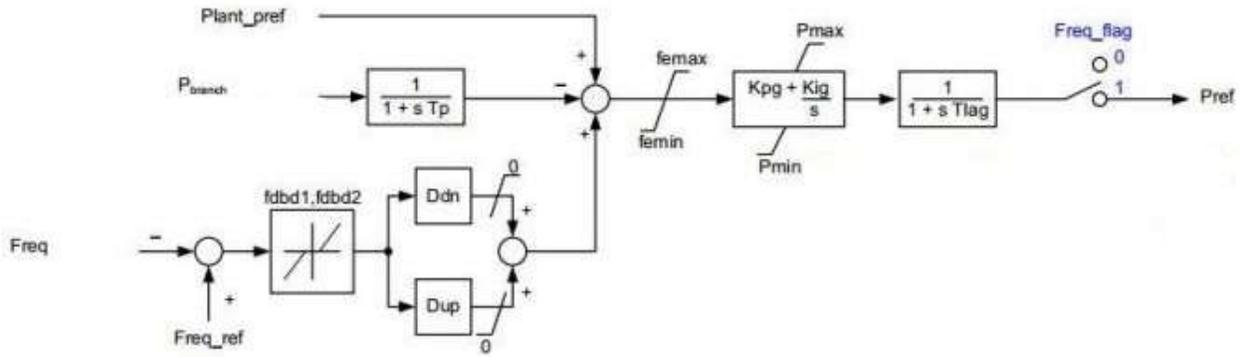
**Figure 13: REPC\_A active power control block diagram [20]**
