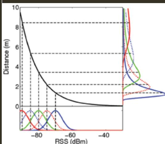
The mapping from RSS measurements to distance estimates can be used to map the Gaussian distribution of RSS measurement error to a distribution of the beacon distance. Note that RSS measurements from distant beacons have high estimation variance illustrated by the wide distribution whereas RSS measurements from nearby beacons have low estimation variance as illustrated by the narrow distribution.
