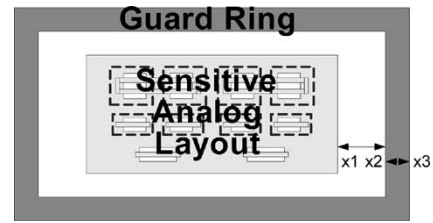
Fig. 11. Guard ring around a sensitive analog circuit. Constraints on the guard ring are: 1) minimum distance from the boundary of the sensitive analog section to the edge of the guard ring: x_2 - x_1 > d ; and 2) width of the guard ring: x_3 - x_2 > w .
