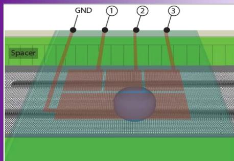
A schematic of the EWOD plate alignment above the surface ratchet, with a droplet sandwiched in between.
