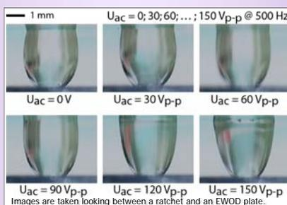
As voltage is increased the contact angles with the EWOD plate are reduced, lifting the droplet's center of gravity further from the ratchet.
