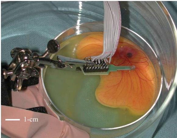
Fig. 7. Device positioned with biosensor implanted into chick chorio-allantoic membrane at day 7.
