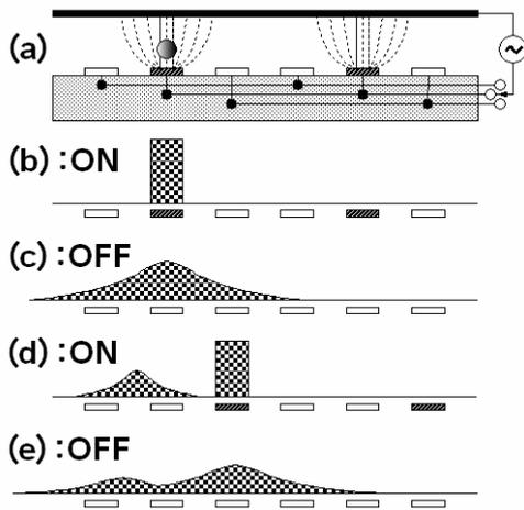
Figure 2. Principle of Brownian motor. 3-phase electrostatic rectification of Brownian motion provides net motion. (a-b) Trapping of the bead. (c) Probability distribution after Brownian motion. (d) Next phase and trapping. (e) Next probability distribution after further Brownian motion.
