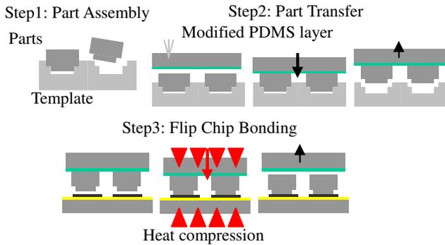
**Fig. 3:** Process flow schematic: (Step 1) The parts are first assembled using a coil shaker; (Step 2) they are then transferred to rubber surface with high van der Waals forces; (Step 3) the parts are then transferred to the final destination substrate (silicon die with patterned solder) by flip chip bonding.
