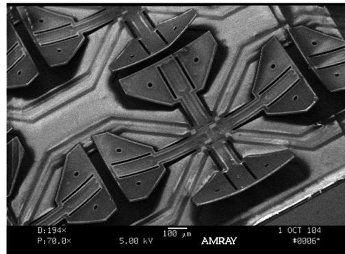
**Figure 2.** Zoomed-in view of cilia chip fabricated by J. Suh [6] in its unheated state. Resistive heating of a thermo-bimorph cilium decreases its curvature. A “motion pixel” consisting of a group of 4 orthogonal cilia is in the center of the image; independent control of the cilia can generate force or motion in 4 orthogonal directions.
