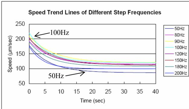
**Figure 6.** Robot for different step frequencies (experimental data). The absolute values depend on the step frequency and reach a maximum near 90 - 100Hz. The slow-down trend over time is similar in all experiments and reflects the reduced step size as the robot is heating up.
