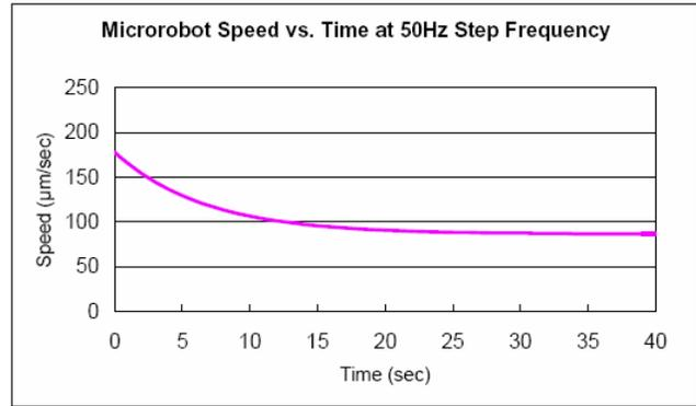
**Figure 4.** Robot speed at 50Hz step frequency (12.5Hz gait frequency). Experimental data (>200 sample points) and curve fitting coincide.  $v(0)=178.3\mu\text{m/sec}$ ,  $v(\infty)=86.6\mu\text{m/sec}$ .
