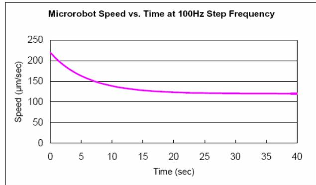
**Figure 5.** Robot speed at 100Hz step frequency (25Hz gait frequency). Experimental data (>200 sample points) and curve fitting coincide.  $v(0)=224.4\mu\text{m/s}$ ,  $v(\infty)=124.5\mu\text{m/s}$ .
