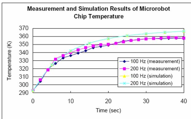
**Figure 10.** Simulated and measured robot temperatures during operation at 100Hz and 200Hz step frequency. A "macroscopic" ANSYS FEM model was used to simulate robot body, cilia, walking surface, and air layer in between.
