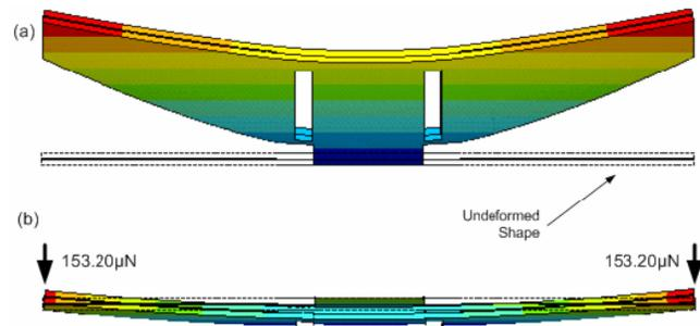
**Figure 9.** ANSYS FEM simulation of cilium (a) with curvature due to thermal stress, (b) with mechanical load of  $153.2\mu\text{N}$  applied to each corner, corresponding to a mass load of approximately 4g distributed over 128 cilia.
