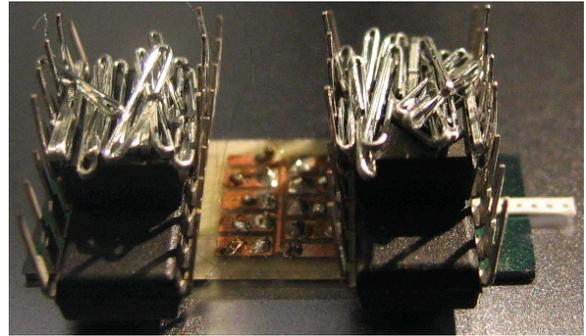
**Figure 8.** Microrobot walking under maximal load, carrying 3.524g in addition to its own mass of 0.478g. 128 cilia lift this load during a 4-phase gait, which implies an average of 31mg per cilium (more than 1000 times the cilium mass). Note: the small white strip extending over the right edge of the robot holds the patterns that are recognized by the motion tracking system.
