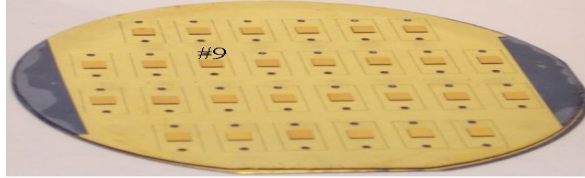
Fig. 7: 28 PZT actuators self-assembled on a 4-inch pump substrate.
