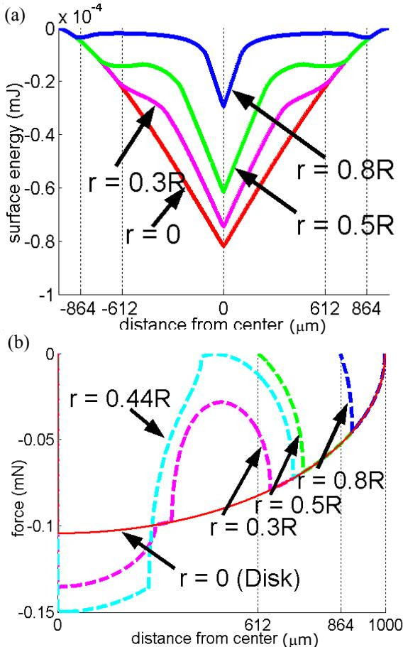
Figure 3. (a) Energy profiles: For ratios of  $r/R = 0.5$  and 0.8 local minima exist at distance  $\pm 610\mu\text{m}$  and  $\pm 860\mu\text{m}$ , respectively. (b) The corresponding force profiles show that when  $r/R \geq 0.45$ , the force vanishes before the part reaches alignment, and it can get stuck without reaching correct alignment.
