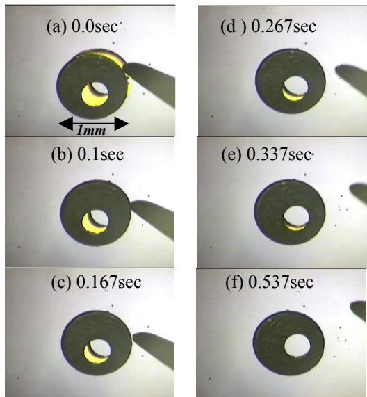
*Figure 6. This sequence of video frames shows how the part was able to shift and rotate back from the misalignment situation. Tweezers were used to force the part away from the binding site to observe the process of self-alignment.*
