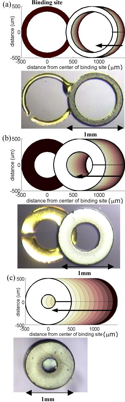
**Figure 1.** Simulation and experimental results agree on the locations of local energy minima during self-assembly of ring-shaped parts. They get stuck at those positions for cutout ratios (a)  $r/R = 0.8$  and (b)  $r/R = 0.5$ . With further decreased cutout ratio (c)  $r/R = 0.3$ , only one global minimum remains, where part and binding site exactly align.
