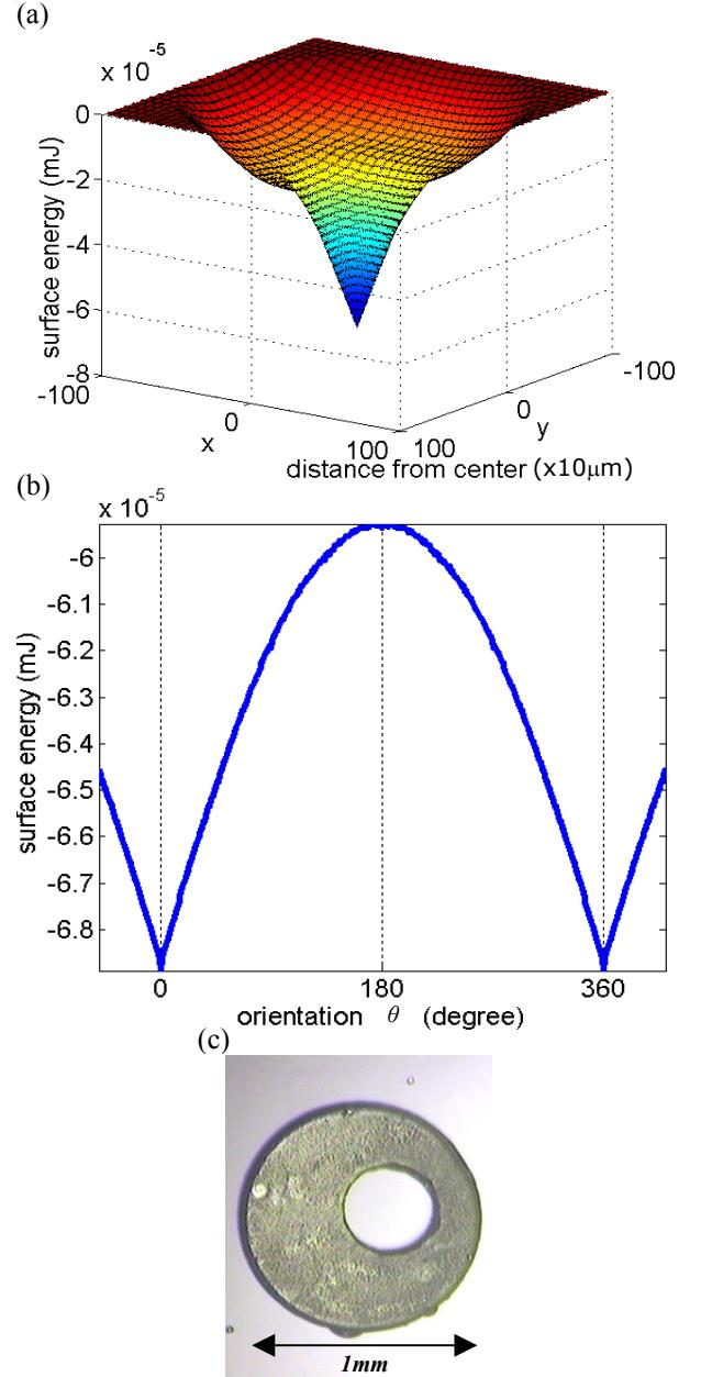
Figure 4. Energy profiles for offset ring design with  $(R, r/R, d/R) = (500\mu\text{m}, 0.4, 0.24)$ . (a) A global minimum of surface energy is found at  $(x,y)=(0,0)$  while translating the part over the binding site. (b) The global minimum also appears when part orients with the binding site for  $(x,y)=(0,0)$ . (c) Experimental result shows exact alignment of the silicon part over the SAM-coated gold binding site in water.
