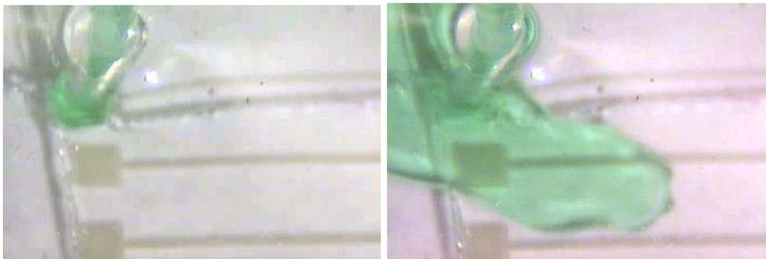
Figure 19: PDMS-sapphire bond leaked
