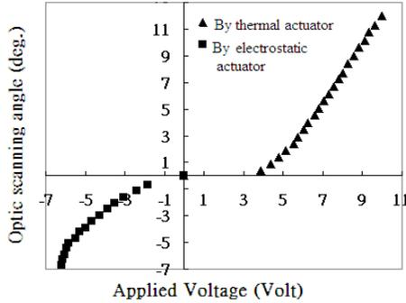
Figure 3: The DC switch characteristics
