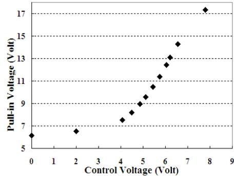
Figure 6: Control (thermal) voltage vs. pull-in voltage
