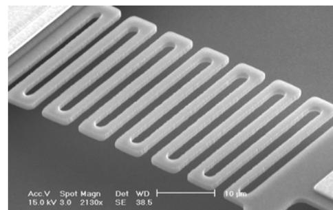
Figure 2: The extended torsion spring
