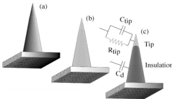
**Figure 1.3-7.** Schematic drawing of the MEMS intracellular electrodes used in this study. (a) The electrodes are made of sharp, bare, silicon needles; (b) the bare silicon is then coated with a metal; (c) finally, a dielectric passivation layer is deposited on the metal layer and the tip of the metal is exposed. The simplified electric model for the tip and the insulation are also presented. The justification to this simplified model is detailed in the text.
