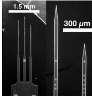
**Figure 1.3-6.** Silicon-based planar microelectrode arrays (MEAs) for cortical recording. D. Kewley and G.T.A. Kovacs. By permission.
