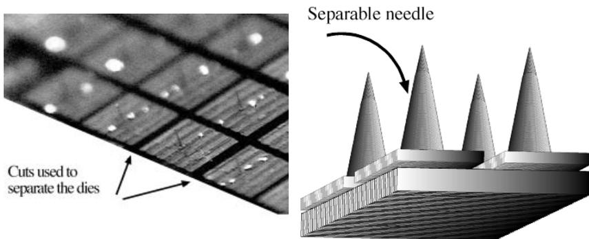
**Figure 1.3-10.** (a) An optical microscope image of an array of diced electrodes. The electrodes are glued to a substrate with an adhesive (photoresist). By soaking the sample in acetone the dies can be separated and used as individual probes. (b) A schematic drawing of the electrodes after the sharpening process is completed.
