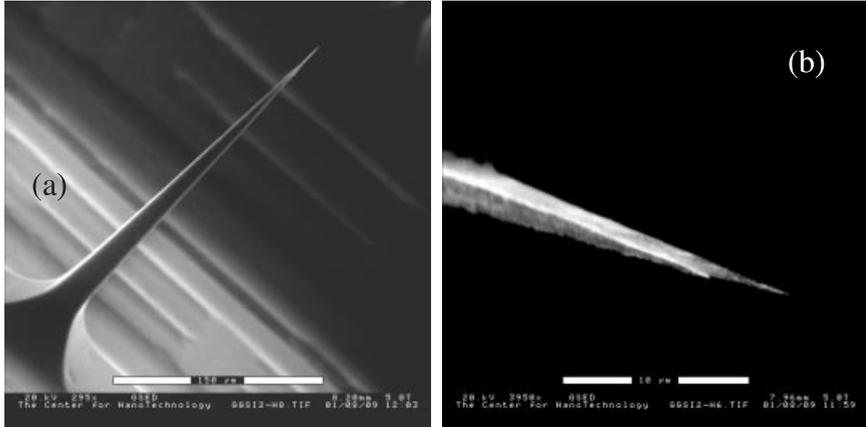
**Figure 1.3-9.** (a) A single needle after the RIE sharpening process. The scale bar is 150  $\mu\text{m}$ . (b) A tip of a sharpened silicon needle. The needle is tilted approximately  $45^\circ$  with respect to the plane of the image. The scale bar is 10  $\mu\text{m}$ .
