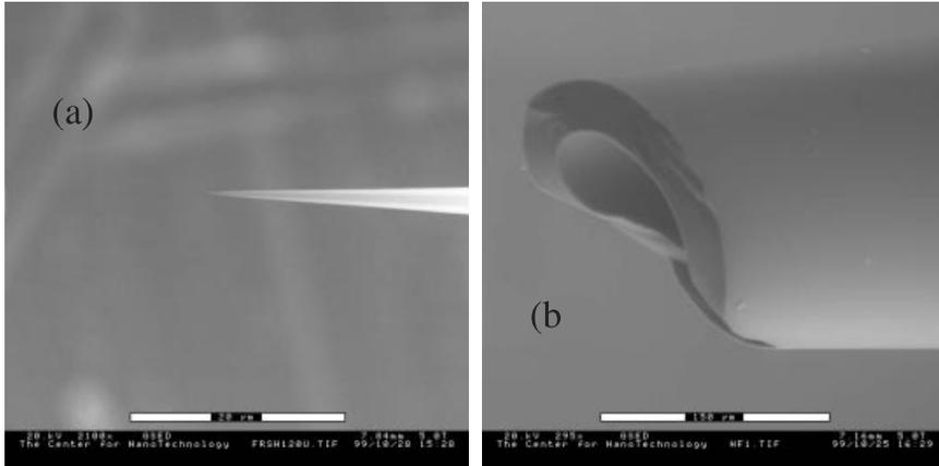
**Figure 1.3-4.** Glass micropipettes. **(a)** An Environmental scanning electron microscope (ESEM) image of the tip of a pulled glass capillary. The scale bar is 20  $\mu\text{m}$ . Similar tips are commonly used for intracellular neuronal recording. **(b)** An ESEM image of a broken glass capillary. The glass provides superb insulation between the inner and the outer sides of the probe. The scale bar is 150  $\mu\text{m}$ .
