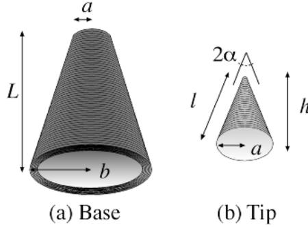
**Figure 1.3-8.** Schematic drawing of the MEMS intracellular electrodes. (a) Geometry of the base, (b) geometry of the tip.
