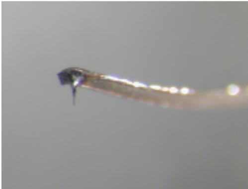
Fig. 7. Released, flexible silicon devices ready for implantation. (Top). The same batch includes both sharpened silicon pillars at the end, (one enlarged below) and devices with bare metal patch electrode.
