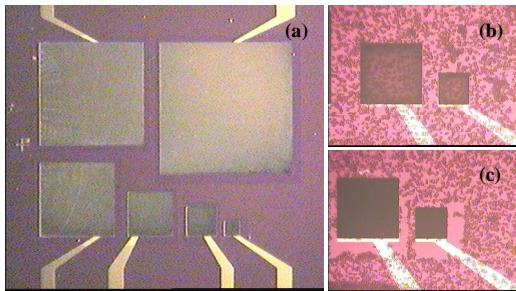
**Figure 6.** (a) Electroplated platinum electrodes (dark squares) with pp4G coating on silicon nitride surface. The two smallest electrodes ((b) bare and (c) coated) after 24 hours in a medium with bovine aortic endothelial cells.
