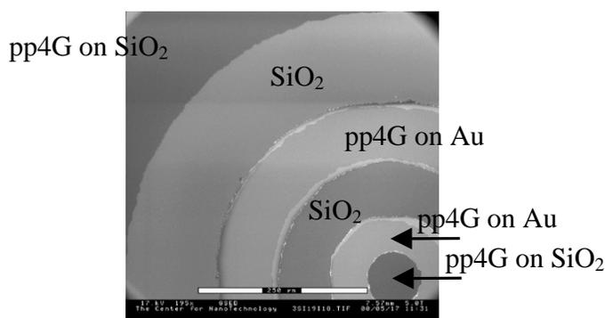
**Figure 2.** ESEM image of pp4G features after lift-off. The pp4G structures are aligned to predefined CrAu structures. Similar results were obtained for structures as small as 10  $\mu\text{m}$ . While current results were produced with low-cost printed masks (features > 10 $\mu\text{m}$ ), we expect minimum feature size and alignment precision for these protein-resistant coatings to be limited only by the lithographic resolution.
