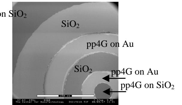
**Figure 2.** ESEM image of pp4G features after lift-off. The pp4G structures are aligned to predefined CrAu structures. Similar results were obtained for structures as small as 10  $\mu\text{m}$ . While current results were produced with low-cost printed masks (features > 10  $\mu\text{m}$ ), we expect minimum feature size and alignment precision for these protein-resistant coatings to be limited only by the lithographic resolution.
