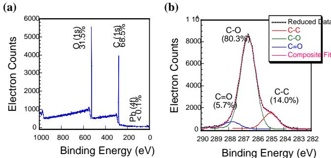
**Figure 3.** ESCA data of a pp4G coating after the photoresist lift-off process: (a) survey scan and (b) carbon 1s high-resolution scan from a patterned pp4G coating on thermal oxide.
