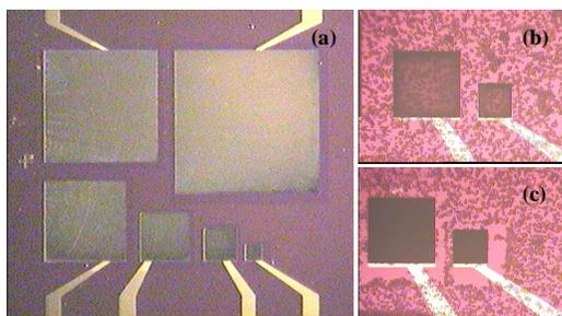
**Figure 6.** (a) Electroplated platinum electrodes (dark squares) with pp4G coating on silicon nitride surface. The two smallest electrodes ((b) bare and (c) coated) after 24 hours in a medium with bovine aortic endothelial cells.
