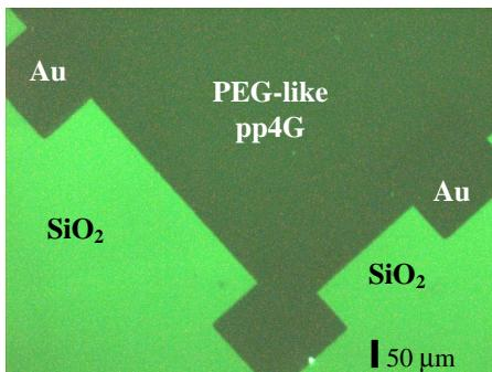
**Figure 4.** A fluorescence microscope image from a fluorescently labeled protein adsorption experiment on a patterned pp4G and SiO<sub>2</sub> surface. Adsorbed proteins covered exposed SiO<sub>2</sub> areas while pp4G coated domains resisted protein adsorption.
