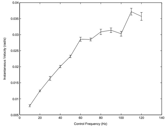
Figure 8. Counter clockwise instantaneous angular velocity, calculated from best fit curve, versus the control frequency.
