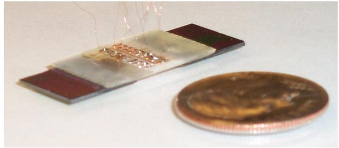
Figure 1. Microrobot in relation to a US Dime. Note the two dark green (grey) cilia chips bonded to the white PCB board. Wire bonds on the bottom side connect the 5 channels of each chip to pads on the PCB board. Nine wires (two sets of four directions plus a common ground) soldered to the top side pads connect the robot to the control box.
