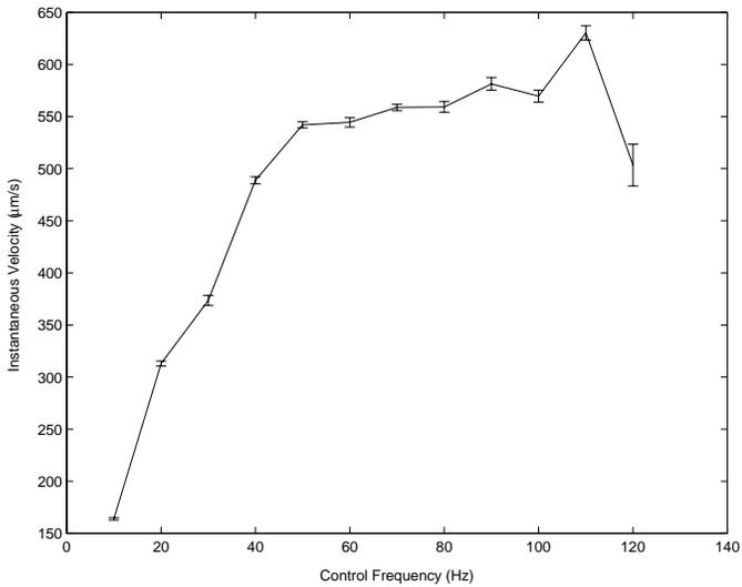
Figure 6. Northwest instantaneous velocity, calculated from best fit curve, versus the control frequency.
