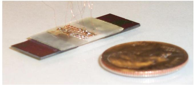
Figure 1. Microrobot in relation to a US Dime. Note the two dark green (grey) cilia chips bonded to the white PCB board. Wire bonds on the bottom side connect the 5 channels of each chip to pads on the PCB board. Nine wires (two sets of four directions plus a common ground) soldered to the top side pads connect the robot to the control box.
