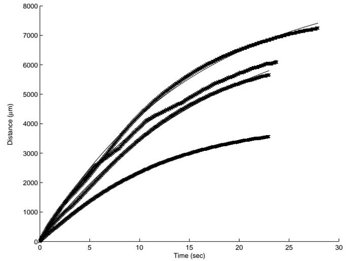
Figure 4. South motion translational displacements, plotted as “x”, and the best fit curve. Plots represent, from bottom up, 30, 60, 120, and 90Hz control frequencies. The highest velocity for these frequencies is achieved at 90Hz.
