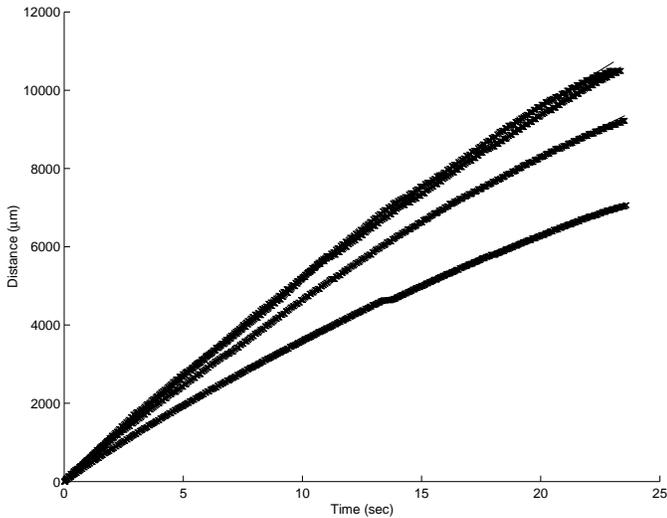
Figure 3. Northwest motion translational displacements, plotted as “x”, and the best fit curve. Plots represent, from bottom up, 30, 60, 120 and 90Hz control frequencies. The highest velocity for these frequencies is achieved at 90Hz.
