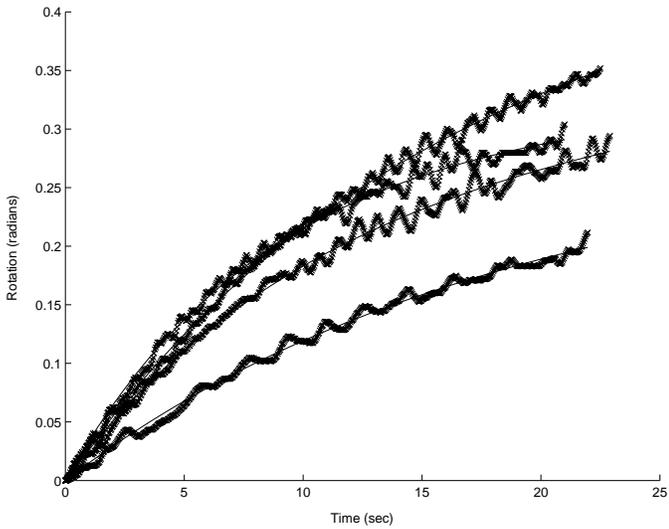
Figure 5. Counter clockwise rotational displacements, plotted as “x”, and the best fit curve. Plots represent, from bottom up, 30, 60, 90 and 120Hz control frequencies. The highest velocity for these frequencies is achieved at 120Hz.
