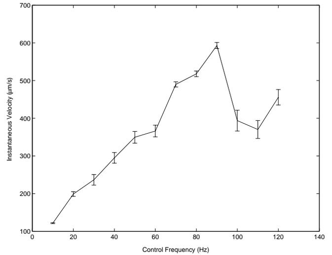
Figure 7. South instantaneous velocity, calculated from best fit curve, versus the control frequency.
