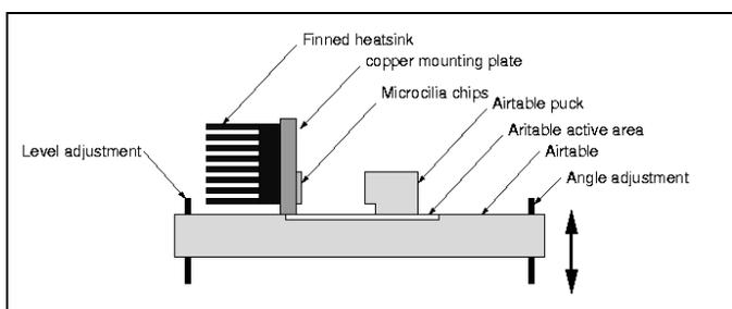
Figure 6. Side view of the airtable.
