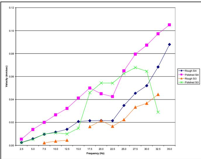
**Figure 11. Comparison of all interface materials for both three- and four-phase gaits.**
