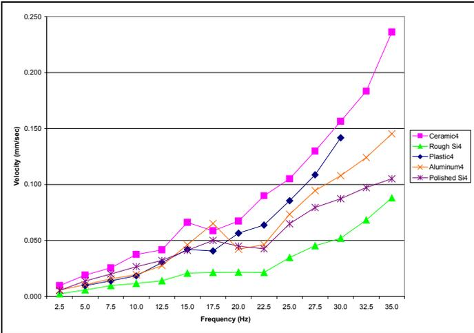
**Figure 10 . Influence of interface material on puck velocity (four phase gait).**
