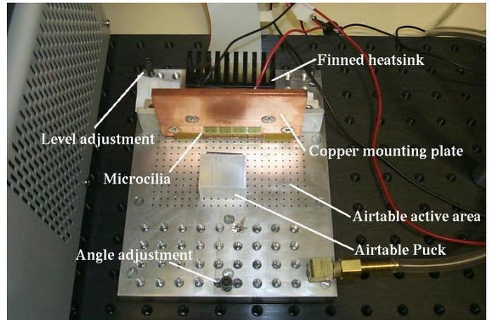
**Figure 2.** Airtable experimental setup to simulate microsatellite docking. A 8”x6” inch perforated aluminum plate with 3 adjustable support screws provides levitation support for an aluminum puck (“pico-sat”). Microcilia chips are mounted on a vertical copper plate with heat sink. The cilia are controlled by a PC and exert a lateral force on the puck during the docking procedure.
