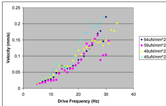
Figure 8. The velocity of the airtable puck (using the beveled plastic bumper) against different drive frequencies and normal forces.
