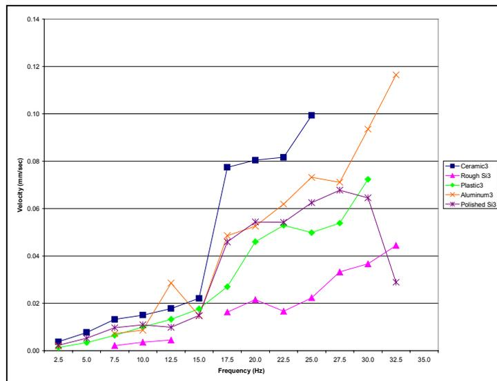
Figure 9. Influence of interface material on puck velocity (three phase gait).
