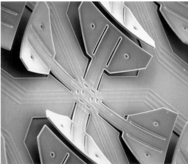
**Figure 1.** Scanning electron microscope (SEM) view of a single microcilia motion cell. The cell is approximately 1mm long and wide. (Image by John Suh, 1997)
