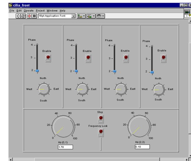
Figure 7. Labview interface for the microcilia. The four controls at the top of the screen dictate the direction and gait of the individual cilia chips. The two large controls at the bottom control the driving frequency of the two leftmost and rightmost chips.
