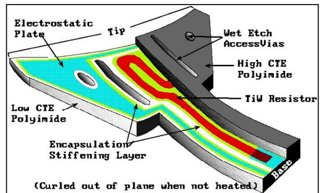
**Figure 4.** Cross sectional view of the microcilia with two layers of polyimide, titanium-tungsten heater loop, and aluminum electrostatic plate. (Image by John Suh, 1997).
