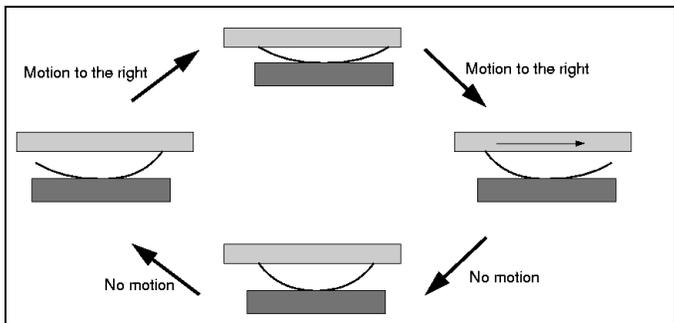
Figure 5. The four phase microcilia motion gait. A three phase gait can be achieved by omitting the top phase.
