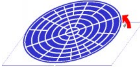
Figure 9 Conceptual design of an actuator array that implements a combined radial-gravity field. Individual actuators are tiled in a circular array pattern. The array is tilted by an angle \phi to add a gravity component \delta g . Under some simplifying assumptions \delta = \tan \phi .
