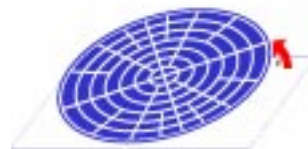
Figure 9: Conceptual design of an actuator array that implements a combined radial-gravity field. Individual actuators are tiled in a circular array pattern. The array is tilted between \phi = 0^\circ and 45^\circ to add a gravity component \delta g with \delta = \tan \phi .
