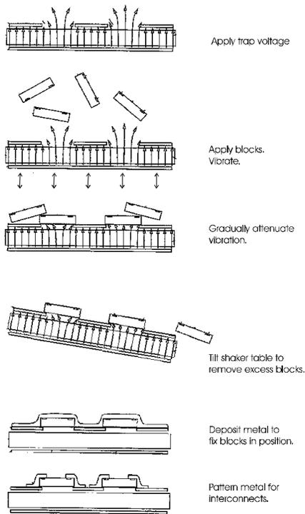
**Figure 9. Process flow for dry electrostatic self-assembly.**<sup>51</sup>
