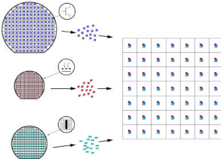
**Figure 1: Conceptual description of parallel microassembly, with the upper wafer being standard CMOS electronics, the middle wafer photonic devices, and the lower wafer microstructures.<sup>1</sup>**
