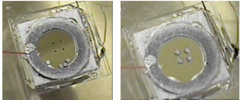
**Figure 10: Dry stochastic assembly with electrostatic force fields: Left: Parts are placed on patterned electrode. Friction is overcome by ultrasonic vibration. Right: Voltage is applied to the electrode; parts are attracted to the apertures (dark squares) and trapped there.**
