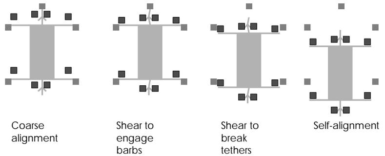
**Figure 14. Shear-lock mechanism.**
