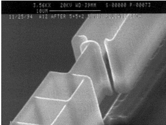
**Figure 13: Single-crystal silicon snap fastener.**<sup>105</sup>
