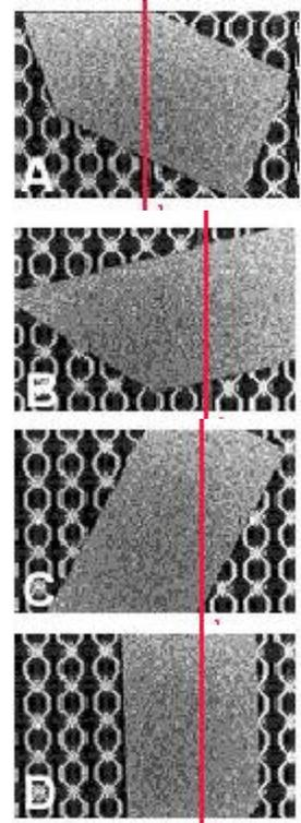
**Figure 12: Open-loop positioning and orienting of a silicon chip on a MEMS cilia array. The chip is centered and aligned with  $\mu\text{m}$  accuracy.<sup>63</sup>**
