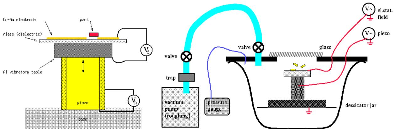
**Figure 11: Experimental apparatus for self-assembly with electrostatic traps. (a) A vibratory table with a gold-coated dielectric is attached to a piezoelectric actuator. The aperture in the upper electrode creates a fringing field that causes polarization in the part. The part is attracted to the aperture. (b) Self-assembly experiments in vacuum. The vacuum provides a controlled environment that minimizes surface sticking effects due to capillary forces and reduces squeeze-film effects.**
