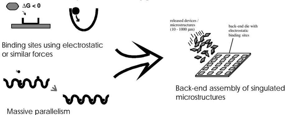
Figure 6. Self-assembly concept<sup>36</sup>.
