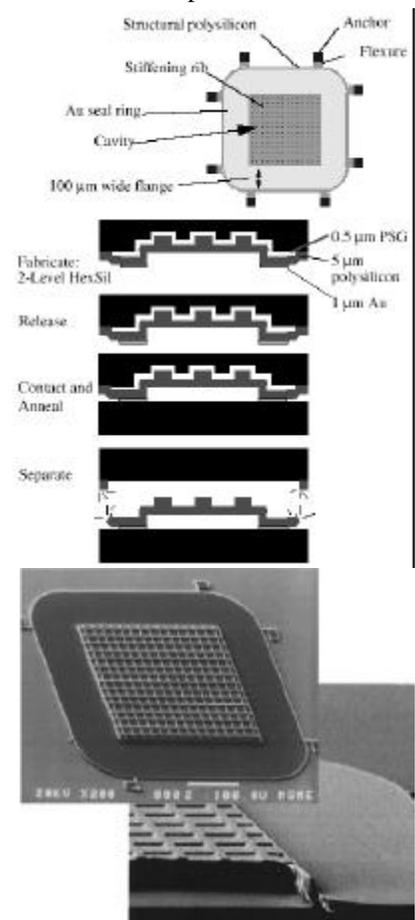
**Figure 3. Process flow for wafer-wafer transfer of vacuum lids (above). Seal formed by Au/Si eutectic weld. SEM of transferred structure, cleaved cross-section (below).**
