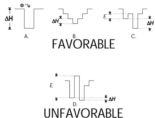
Figure 7. Comparison of favorable and unfavorable potential energy functions for self-assembling systems.<sup>64,106</sup>
