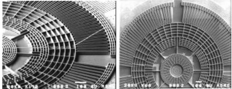
Figure 4. Two-piece HexSil microactuator transferred onto glass substrate using indium solder bonding.
