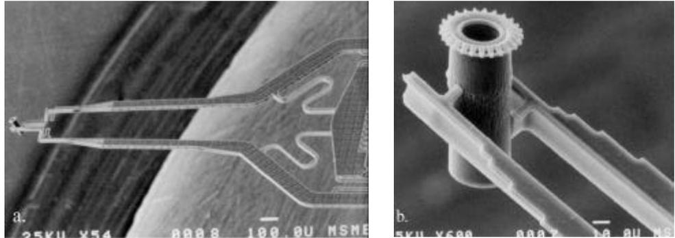
**Figure 2: SEMs of Hexsil molded polysilicon microtweezers gripping a Hexsil gear.<sup>19</sup> (a) the overall structure is 5 mm in length, but the gripper contains features that are smaller than 10  $\mu\text{m}$ .**
