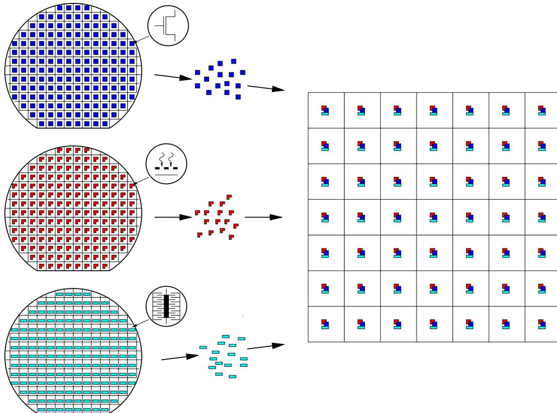
Figure 2: Parallel microassembly: Multiple micro-scale components (e.g. electronics, photonics, and MEMS) are built in parallel using standard fabrication processes. They are positioned and combined with other components on a hybrid “pallet.” Note that the fabrication density is very high, while the pallets may have a larger size and lower density.
