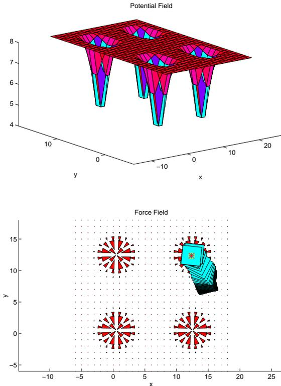
Figure 7: (a) Potential field created by an electrode with four small square-shaped apertures, as shown in the experimental setup in Figure 1. The four potential traps correspond to the four apertures. (b) Simulation of a square part moving in the corresponding force field (denoted by force vectors) The part translates and rotates until it reaches a local minimum in the potential field.
