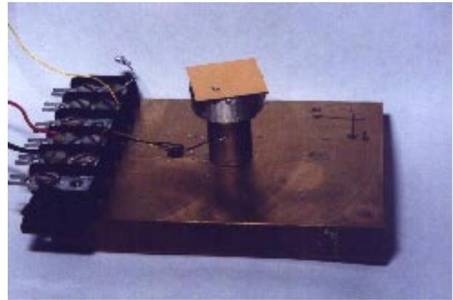
Figure 4: Experimental apparatus for self assembly experiments. A lithographically patterned electrode is attached to a piezoelectric actuator (vertical cylinder). Some parts can be seen in the lower left quadrant of the substrate.
