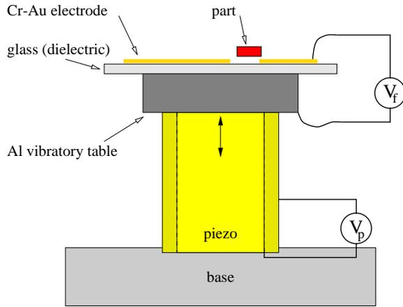
Figure 3: Experimental apparatus for self assembly with electrostatic traps. A vibratory table with a gold-covered dielectric is attached to a piezoelectric actuator. The aperture in the upper electrode creates a fringing field that causes polarization in the part. The part is attracted to the aperture.
