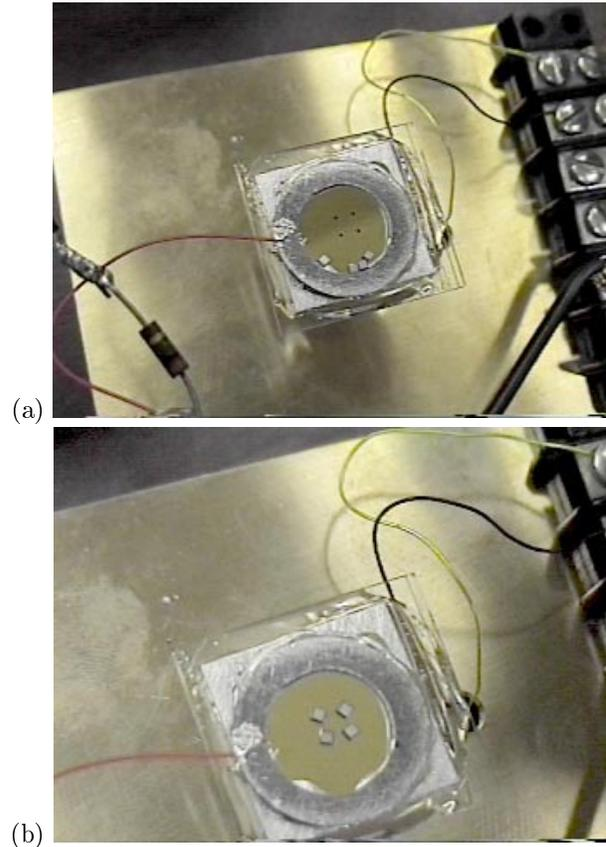
Figure 1: Parallel microassembly with electrostatic force fields: (a) Surface-mount capacitors are placed onto a glass substrate with a 100 nm thin patterned Cr-Au electrode. Frictional and adhesive forces are overcome by ultrasonic vibration. (b) Voltage applied to the electrode creates an electrostatic field. The parts are attracted to the apertures in the electrode (dark squares) and are trapped there.
