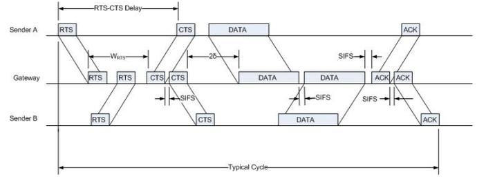
**Figure 6: Common timing of hypothetical single channel protocol**
