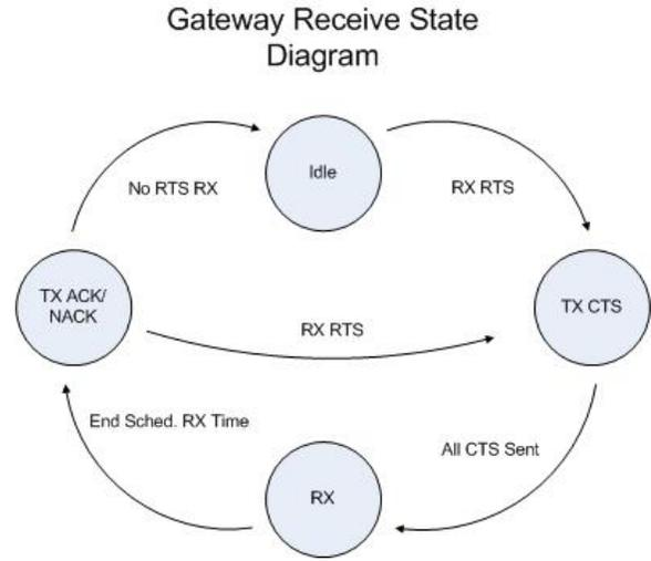
Figure 3: Gateway node RX process
