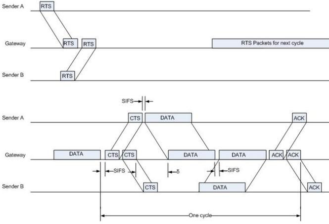
**Figure 5: Typical cycle using dedicated control channel. *Top: Control channel, Bottom: Main channel***
