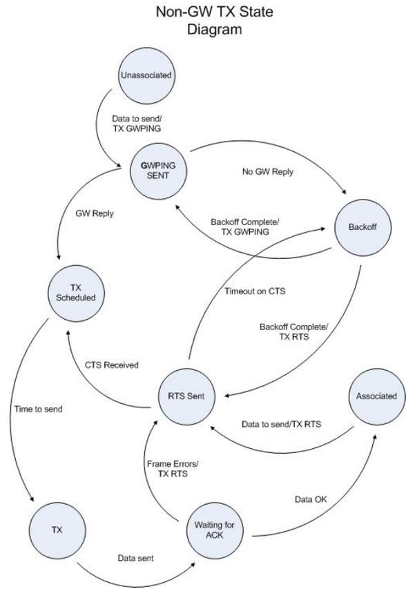
Figure 4: Non-Gateway node TX process
