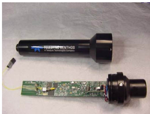
Fig. 5. Smart Marker, essentially a reduced size, lower power modem used as an object marker in underwater environments.
