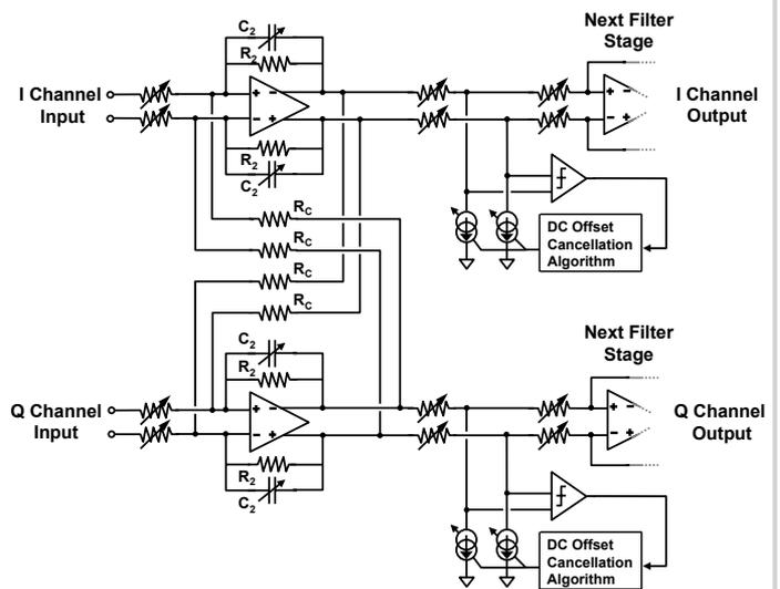
Figure 17.6.2: One complex pole stage of 5<sup>th</sup>-order filter.
