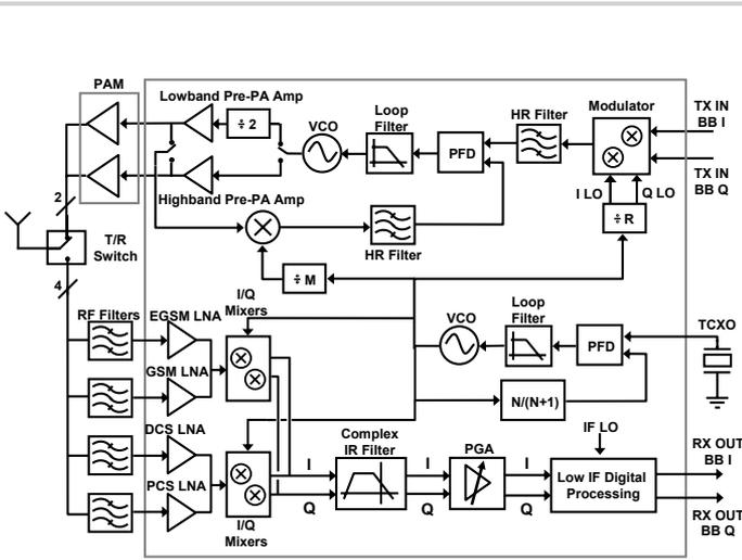
Figure 17.6.1: Quad-band transceiver block diagram.
