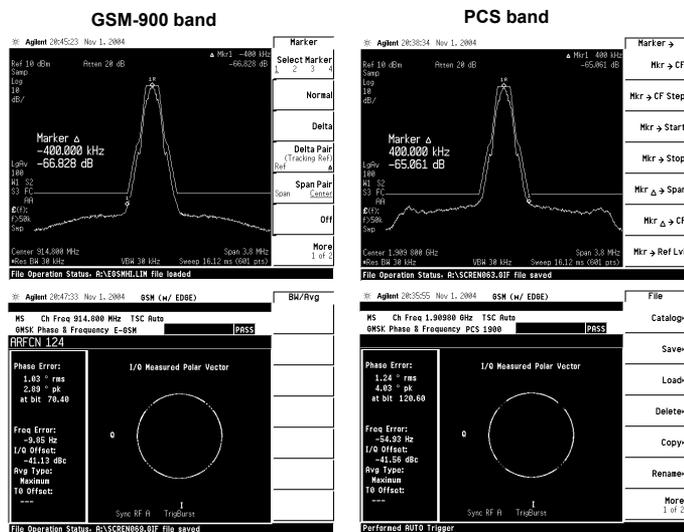
Figure 17.6.3: TX rms phase error and modulation mask.
