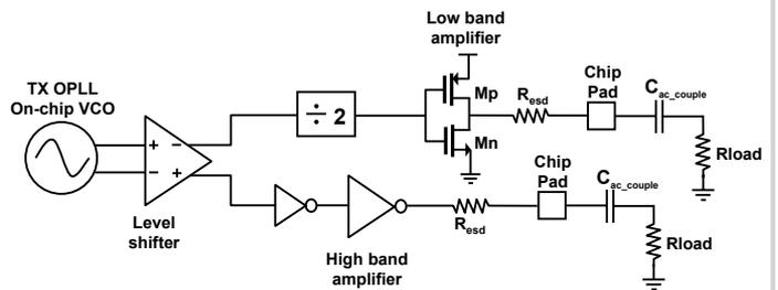
Figure 17.6.4: High and low band pre-PA drivers.
