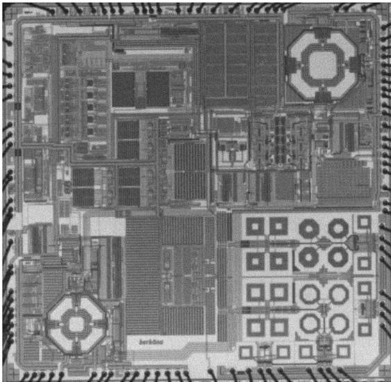
Figure 17.6.7: Single chip quad-band transceiver die micrograph.
