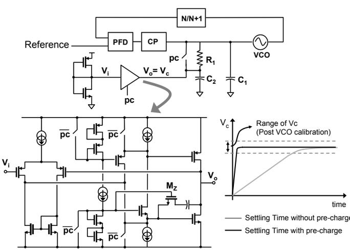
Figure 17.6.5: Fractional-N synthesizer with pre-charger.
