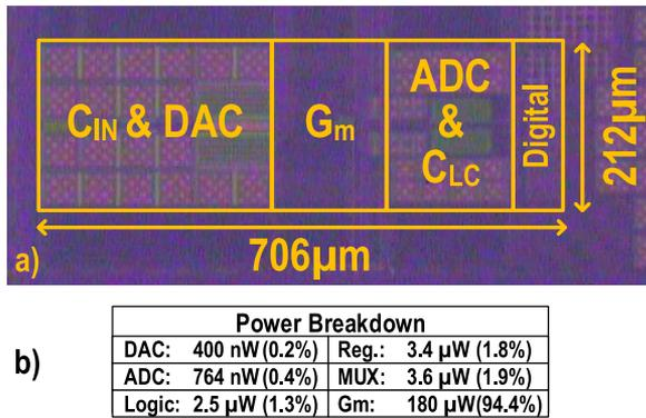
Fig. 13. (a) Die photomicrograph of 65 nm 1p9m TSMC CMOS 64-channel multiplexed recording prototype and (b) system power breakdown.
