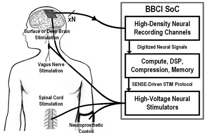
Fig. 1. Conceptual diagram of a closed-loop Bidirectional-Brain Computer Interface (BBCI) which includes neural recording, real-time digital computation, and stimulation.
