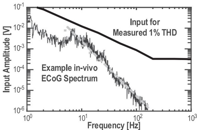
Fig. 17. RMS input amplitudes causing 1% Total Harmonic Distortion, measured with single-tone sinusoids across frequency for ECoG recording. Overlaid with a typical ECoG PSD (2kS/s) adapted from [27].
