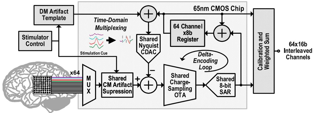
Fig. 2. Functional block diagram of the highly-multiplexed, digitally-delta-encoded ECoG signal chain with common- and differential-mode artifact suppression that is selectively enabled when cued by the stimulator.
