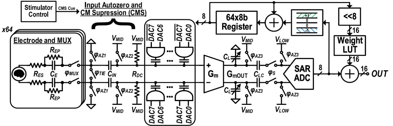
Fig. 4. Detailed schematic of the analog front end, including delta-encoded feedback loop with 8-bit DAC and 8-bit ADC, CMS system, autozero technique, and interpolation.
