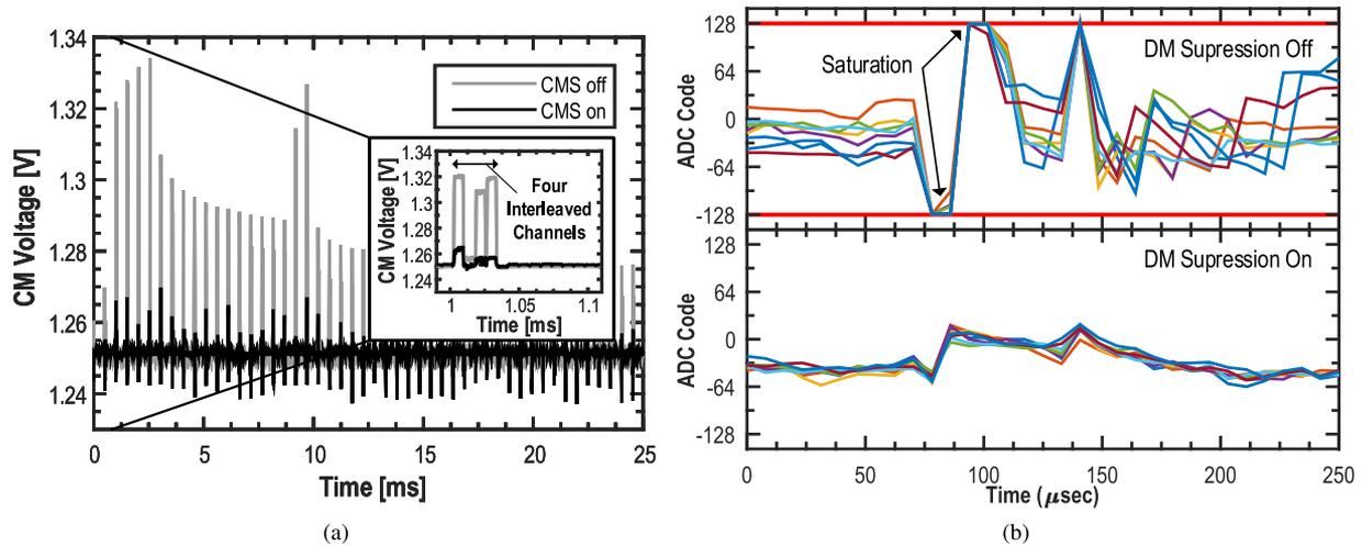
Fig. 21. In-vivo recordings in the presence of artifacts for common- (a) and differential-mode (b). (a) shows the voltage at the input to the amplifier with and without common-mode suppression. (b) shows the reconstructed output waveform with and without front-end suppression. Measurements were performed with 300  $\mu$ A biphasic stimulation in PtIr microwire electrodes adjacent to recording electrodes, creating 100 mV Pk-Pk stimulus artifact at the recording inputs.
