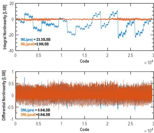
Fig. 16. INL and DNL measurements of the prototype both before and after calibration obtained using the histogram method over 16777216 samples. The DNL is dominated by the noise floor of the amplifier, while the INL shows 2.90LSB linearity after calibration, demonstrating very strong linear performance across the entire input range.
