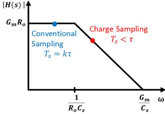
Fig. 9. Qualitative frequency-domain description of charge sampling with respect to conventional sampling. Charge sampling occurs above the 3 dB bandwidth of a single-pole amplifier and sacrifices some gain for faster settling response.
