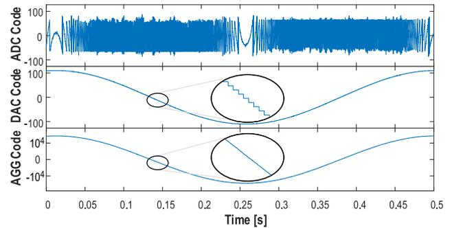
Fig. 14. Demonstration of the ADC+DAC aggregation for a 2 Hz, 35 mV rms sinusoidal input demonstrating the DC offset cancellation range of the system and basic operation. The ADC residue interpolates the coarsely quantized DAC signal to create a 14-bit aggregated output.
