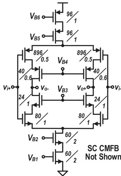
Fig. 8. Transistor level implementation of the charge-sampling OTA, similar to [28].
