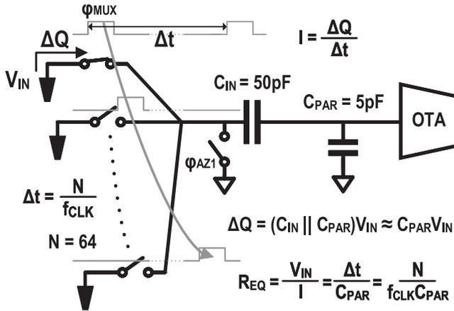
Fig. 5. Conceptual diagram of input network charging and resulting equivalent input resistance, as seen from the perspective of each recording electrode.
