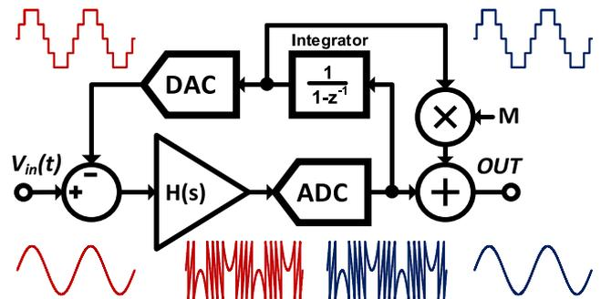
Fig. 3. Delta encoding using an accumulating digital feedback loop. The aggregate count in the accumulator tracks the coarse voltage level that is fed back to the DAC, while the ADC output is the delta between the accumulated value and input voltage. Summing the ADC residue with the DAC interpolates the coarsely quantized DAC output to reconstruct the full signal waveform.
