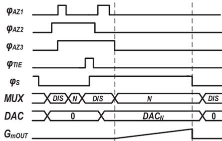
Fig. 7. Autozero and sampling operation timing diagram for CMS operation.
