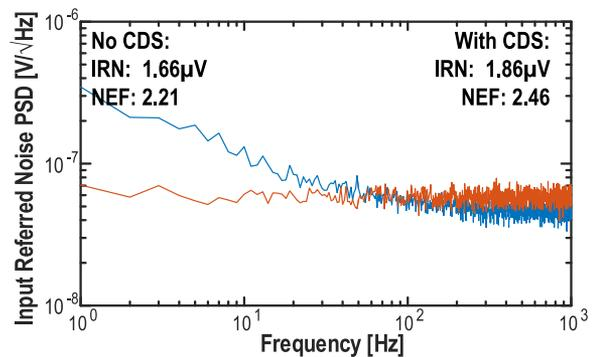
Fig. 15. Input-referred noise measurements for ECoG recording configurations operating with time-domain multiplexing. Noise measurements are shown for one of the 64 operational time-interleaved channels. Switching noise is below the amplifier noise floor by design. Correlated-double sampling (CDS) operation is also shown (in orange).
