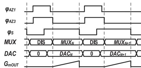
Fig. 6. Autozero and sampling operation timing diagram for normal recording mode. Note: Switch AZ2 remains open during normal operation.
