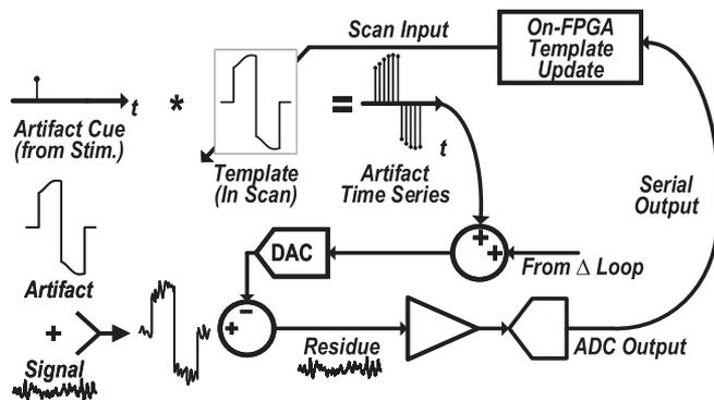
Fig. 12. Template-subtraction based architecture. A cue from the stimulator during a stimulation event enables look-up of the learned artifact. Samples of this template are combined with the Delta-Encoding feedback signal to cancel stimulation artifacts at the amplifier input.
