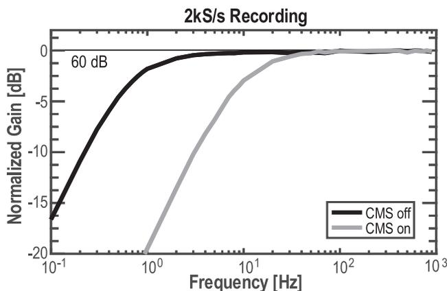
Fig. 18. Measured full signal chain transfer functions for ECoG (2kS/s).
