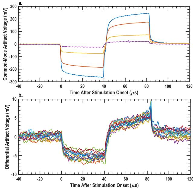
Fig. 11. Common-mode (a) and differential-mode (b) artifacts for an H-bridge type stimulator. The amplitude and shape of both artifacts can vary considerably with the stimulation current and electrode.
