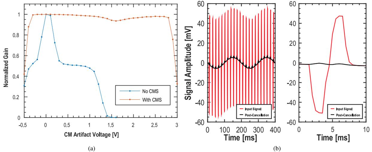
Fig. 19. Bench measurements of the CMS (a) and DMS (b) systems. (a) shows the CMS system swept over CM artifact voltage levels both with and without CMS enabled. The CMS largely mitigates gain variation compared to the nominal case. (b) shows a 10 mV sinusoidal 5 Hz signal with a  $\pm 54$  mV biphasic stimulation artifact (differential) before and after front-end suppression.
