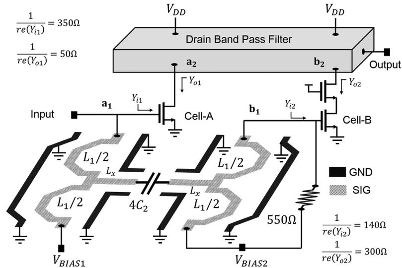
Fig. 5. Circuit diagram of the BPDA.
