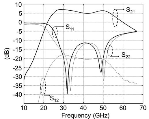
Fig. 7. BPDA measured S-parameters.
