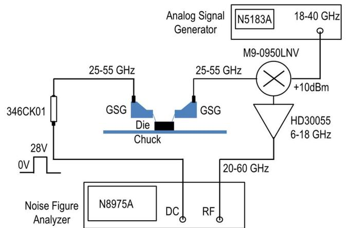
Fig. 8. Setup for BPDA noise characterization using the N8975A noise-figure analyzer.
