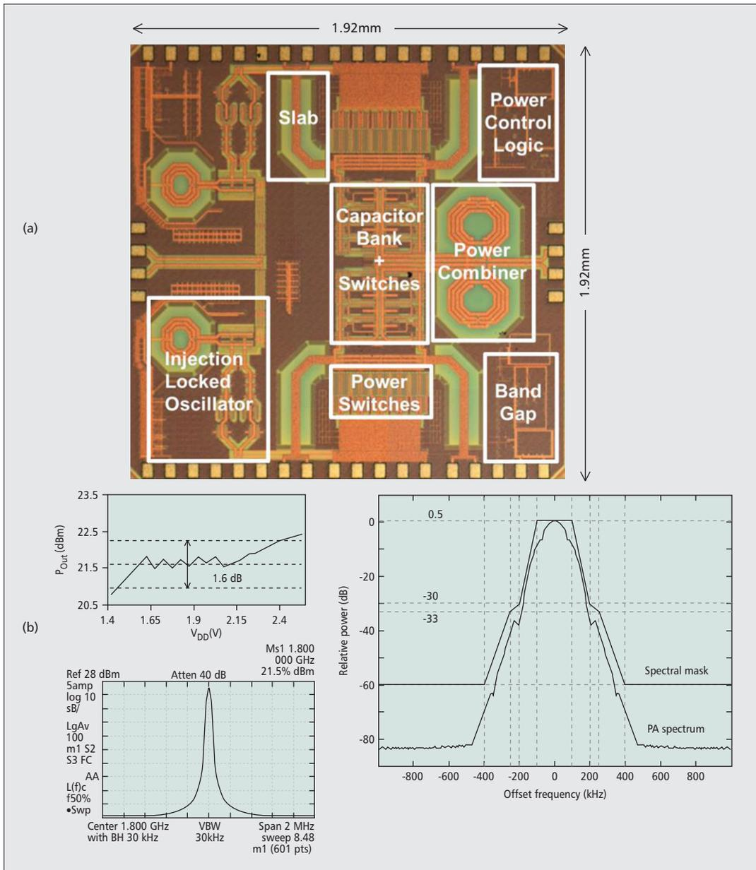
Figure 5. a) PA die photo; b) measurement results.
