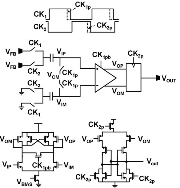
Fig. 18. Comparator schematic and timing diagram.
