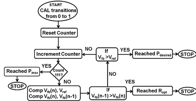
Fig. 16. Algorithm for regulatorless power control loop.
