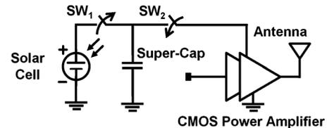
Fig. 3. CMOS power amplifier for long-range sensor TX.
