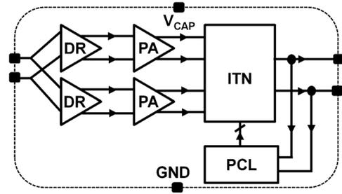
Fig. 13. Block diagrams of the long-range sensor transmitter.
