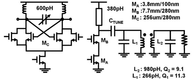
Fig. 14. Injection-locked oscillator driver and PA output stage.
