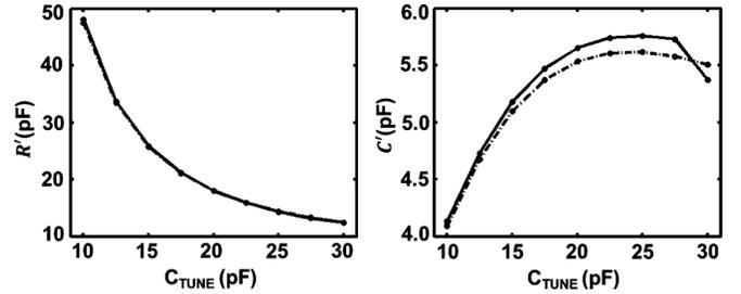
Fig. 10.  $R'$  and  $C'^{prime}$  variation as a function of the tuning capacitance.
