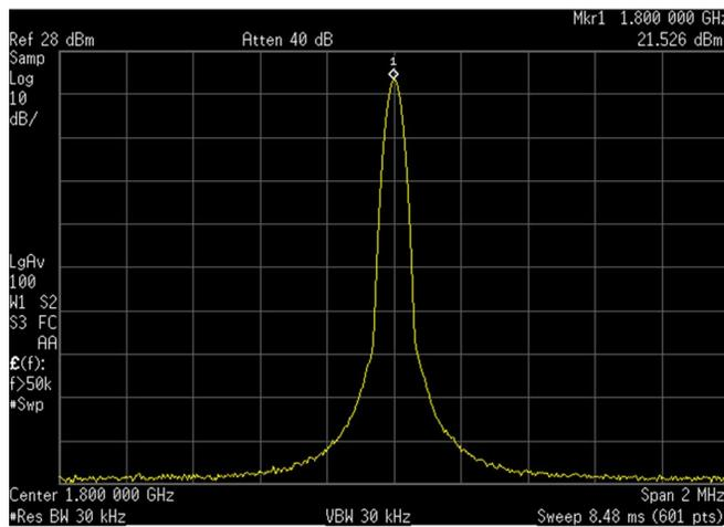
Fig. 24. Measured PA output power (including the 2.5-dB cable loss) with a 1.8-GHz single-tone input, 2.5-V supply voltage, and TMN in the maximum output-power state.
