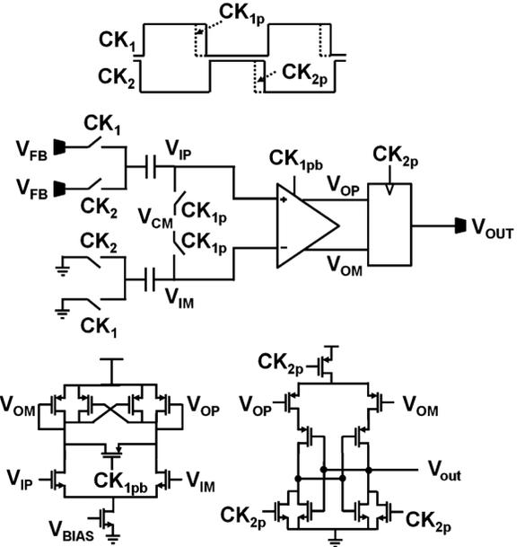
Fig. 18. Comparator schematic and timing diagram.
