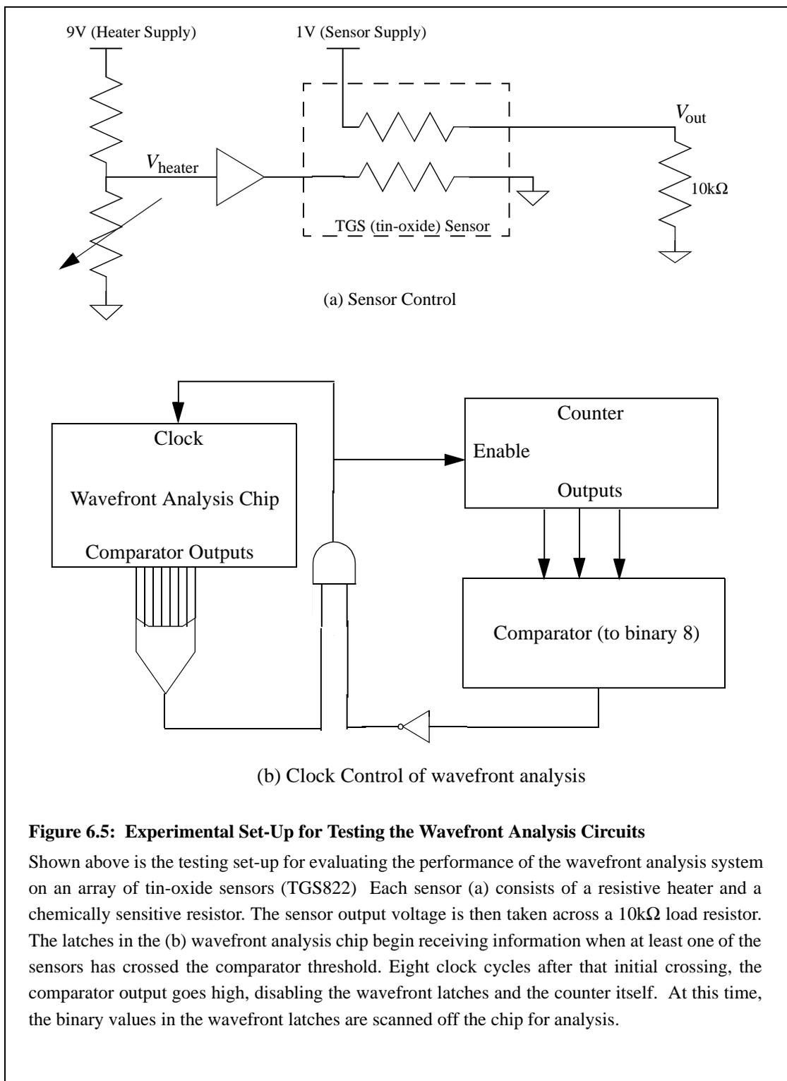
**Figure 6.5: Experimental Set-Up for Testing the Wavefront Analysis Circuits**
