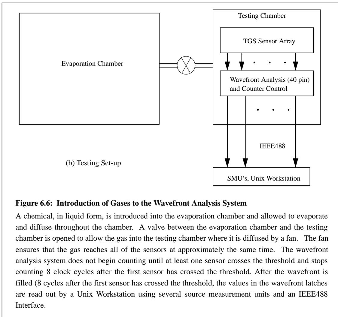
**Figure 6.6: Introduction of Gases to the Wavefront Analysis System**
