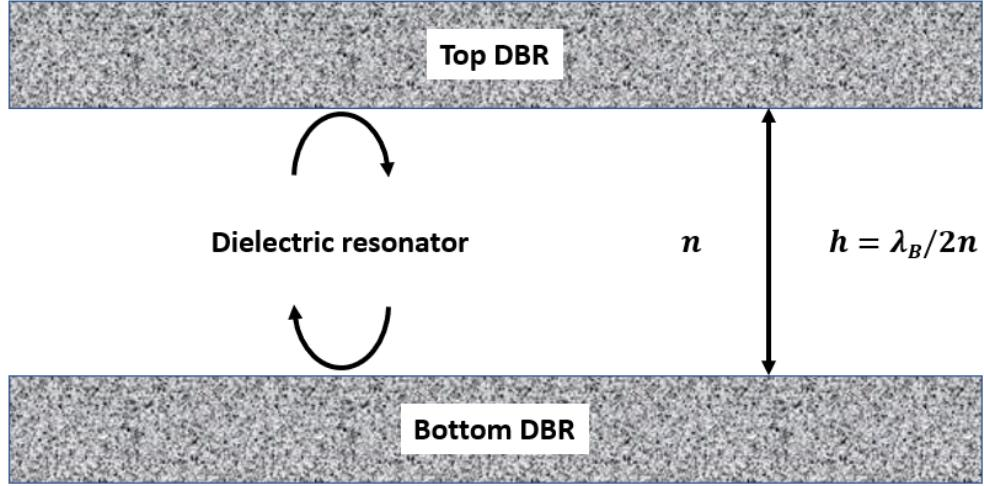
Figure 2.2: **Distributed Bragg reflector resonator.** A dielectric resonator formed by the inclusion of a  $\pi/2$  phase shift defect within a distributed Bragg reflector (DBR). Alternatively, this can be understood in terms of a resonance formed between two DBRs.
