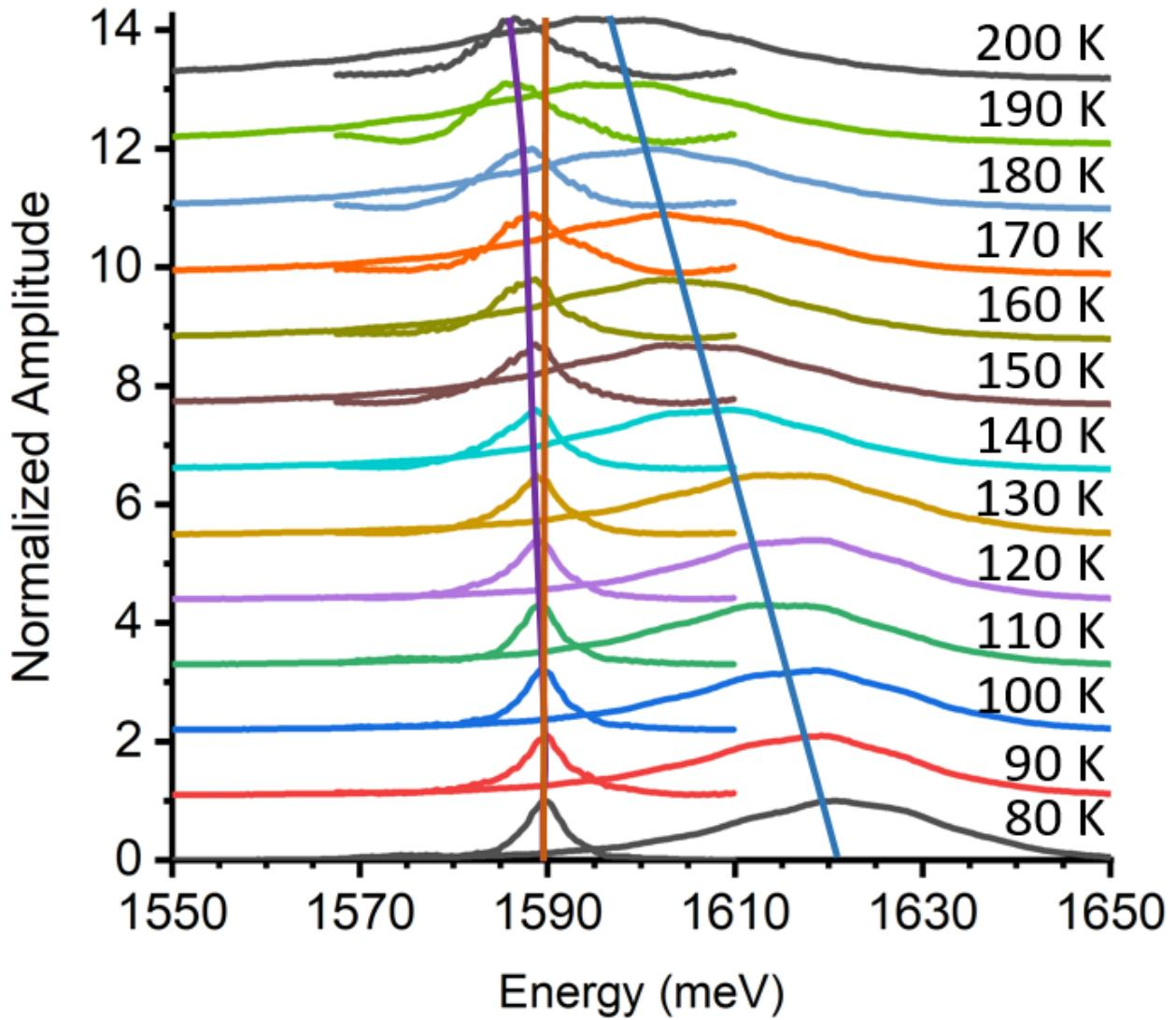
Figure 3.5: Overlayed plots of the cavity transmission (left peak) and MoSe<sub>2</sub> photoluminescence (right peak). The center frequency of the neutral exciton exhibited in the photoluminescence is plotted in Fig. 3.3a. The center frequency of the cavity resonance is plotted in Fig. 3.4c with respect to the exciton detuning from the bare cavity resonant frequency.
