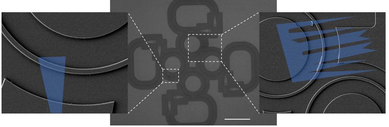
**Figure 2.6: Silicon nitride ring resonator transfer.** Optical image of exfoliated WSe<sub>2</sub> and MoSe<sub>2</sub> monolayers integrated onto the left and top ring resonators, respectively, with false-color SEM images of the integrated monolayers. Scale bar is 10  $\mu\text{m}$ .
