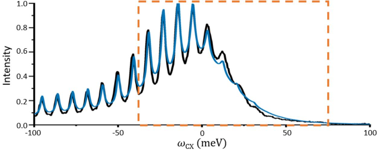
Figure 4.4: **Theoretical fit of a polaron model to cavity-coupled photoluminescence data.** Measured cavity-coupled PL (black) and simulated cavity-coupled PL (blue) at 80 K. Theoretical model fit to the windowed region of data with the Hamiltonian described in the text ( $T = 80$  K,  $\gamma = 48.4$  meV,  $\alpha_p = 0.018$  ps $^2$ ,  $\omega_b = 6.7$  meV,  $\kappa = 2.85$  meV,  $g = 4$  meV).
