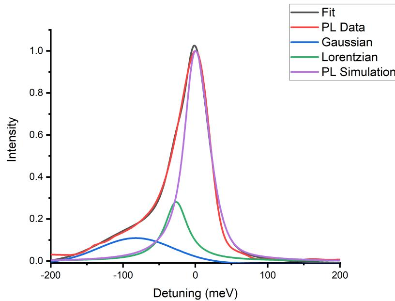
Figure 4.2: **Photoluminescence spectra and fit for an excitonic transition.** The extracted fit parameters for equation 4.19 are:  $y_0 = -0.01262$ ,  $A_D = 15.82$ ,  $\Gamma_D = 122.0$  meV,  $\Delta_D = -82.31$  meV,  $A_T = 17.02$ ,  $\Gamma_T = 38.56$  meV,  $\Delta_T = -26.55$  meV,  $f = 0.9038$ ,  $\alpha_p = 0.018$  ps<sup>2</sup>, and  $\omega_b = 6.7$  meV.
