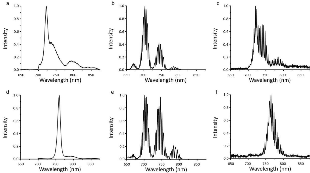
**Figure 2.7: Ring resonator spectra with integrated monolayer  $\text{WSe}_2$  and  $\text{MoSe}_2$ .**
