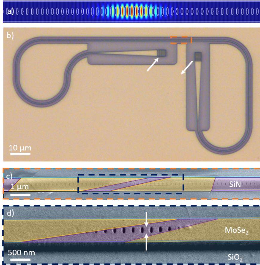
**Figure 3.1: Monolayer MoSe<sub>2</sub> integrated onto a photonic crystal defect resonator.**
