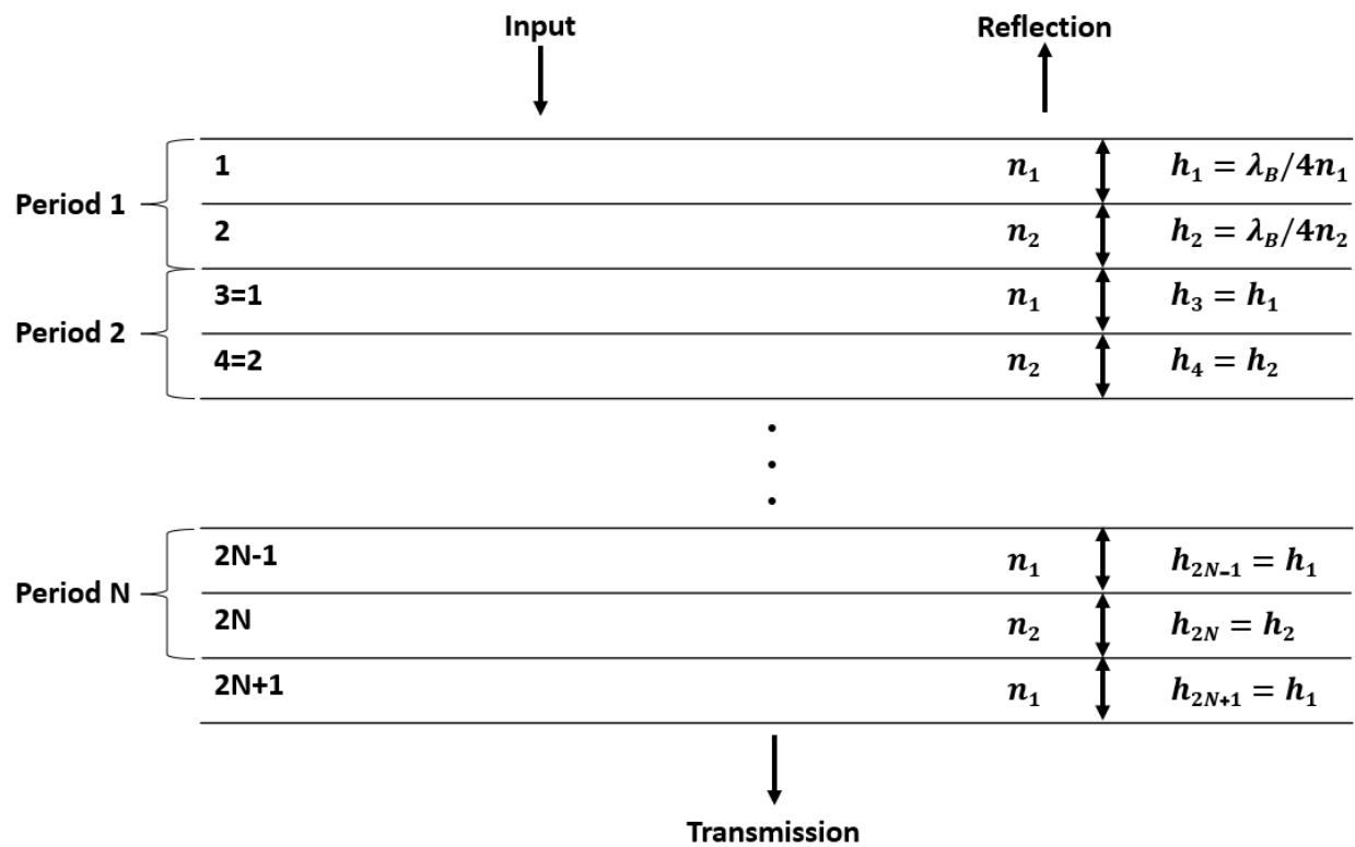
Figure 2.1: **Distributed Bragg reflector.** A distributed Bragg reflector (DBR) consisting of  $2N + 1$  layers of alternating quarter-wavelength high and low index materials [65].
