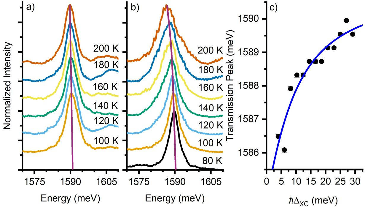
Figure 3.4: Temperature dependence of the monolayer  $\text{MoSe}_2$  integrated onto a photonic crystal defect resonator. a) Representative transmission spectra of the nanobeam cavity without an integrated flake of monolayer  $\text{MoSe}_2$  at 100 K to 200 K in 20 K increments. b) Representative transmission spectra of the nanobeam cavity with an integrated flake of monolayer  $\text{MoSe}_2$  at 80 K to 200 K in 20 K increments. c) Dispersive shift of the cavity resonance in transmission.
