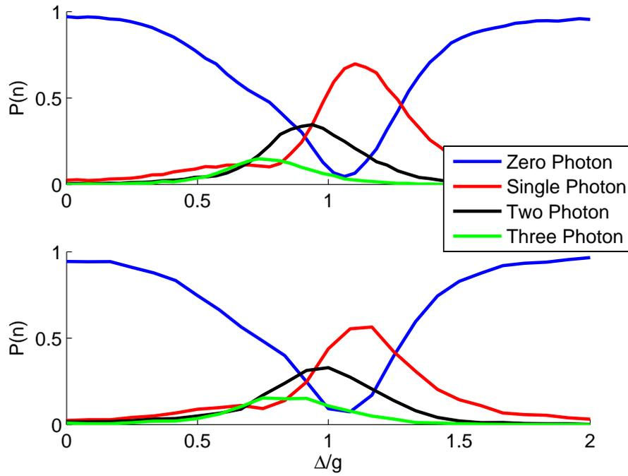
Figure 5.13: The effect of pure QD dephasing on the Fock state generation: (a) Probability  $P(n)$  of generating  $n$  photon states as a function of  $\Delta/g$ . No QD dephasing is included. (b)  $P(n)$  as a function of  $\Delta/g$ , with a pure QD dephasing rate  $\gamma_d/2\pi = 1$  GHz. For all the simulations:  $\kappa/2\pi = 4$  GHz and  $g/2\pi = 40$  GHz.
