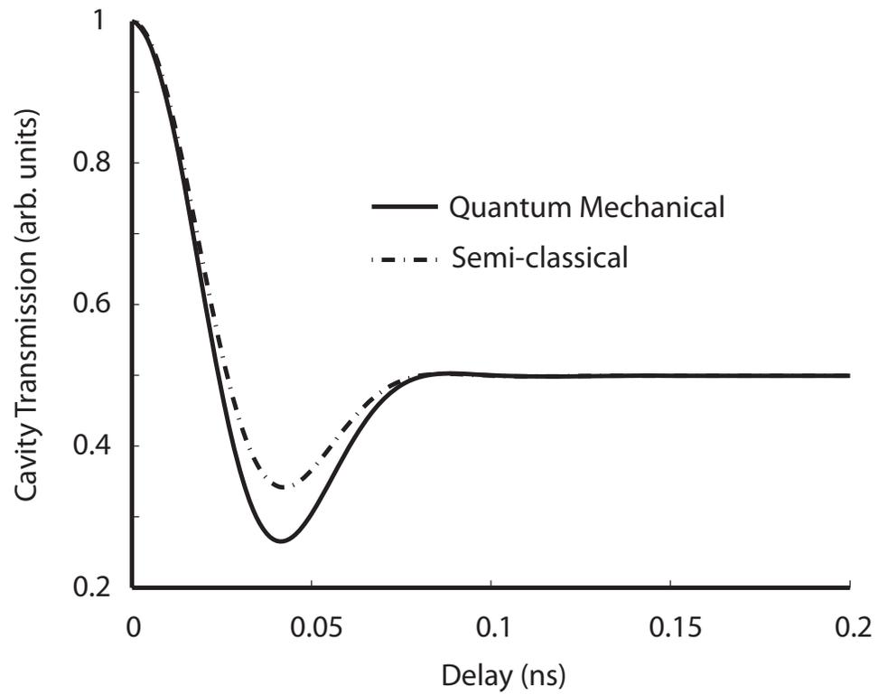
Figure 2.6: Comparison between two methods: quantum optical and semi-classical. The integrated cavity transmission is plotted as a function of the delay between two pulses. The two methods match quite well at zero and large time delay. However, they differ at the minimum transmission due to destructive interference between two pulses.
