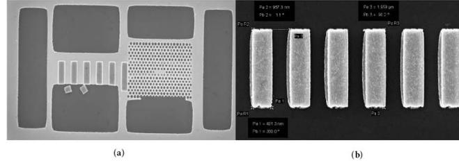
Figure 9.2: (a)SEM of a photonic crystal cavity with metallic grating on the side. (b) SEM of a metallic grating fabricated for generating surface acoustic wave.
