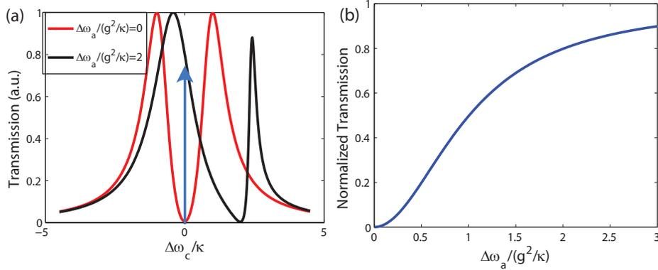
Figure 2.10: (a) Transmission spectra of coupled cavity-QD system for two different QD-cavity detunings. The blue arrow shows the wavelength of the laser whose transmission is being modified. (b) Normalized steady state transmission with different QD detunings. The laser is resonant with the cavity. We used the following parameters:  $g/2\pi = \kappa/2\pi = 20$  GHz;  $\gamma = \kappa/80$ ; the pure dephasing rate is assumed to be zero for this analysis ( $\gamma_d/2\pi = 0$ ).
