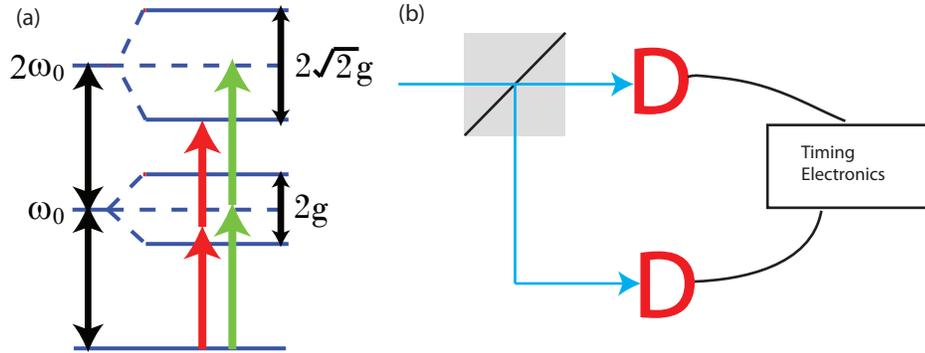
Figure 5.6: (a) The anharmonic ladder structure: when the laser is detuned from the polariton, then the coupling of the first photon is difficult, but two photons together can reach the second order manifold, and the output light will have more two photon character.
