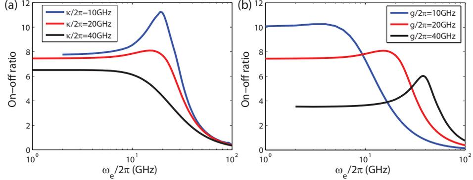
Figure 2.11: The frequency response of the switch for different (a)  $\kappa$ . ( $g/2\pi$ ) is kept constant at 20 GHz and (b)  $g$ . ( $\kappa/2\pi$ ) is kept constant at 20 GHz. For both simulations  $\Omega = 1$  GHz;  $\Delta\omega_0/2\pi = 10$  GHz;  $\gamma_d/2\pi = \gamma/2\pi = 0.1$  GHz.
