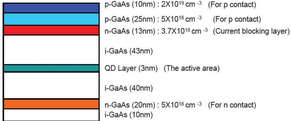
Figure 4.5: The details of the p-n-i-n wafer with doping densities.
