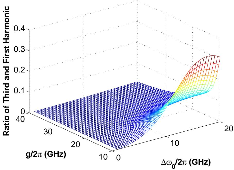
Figure 2.16: Ratio between the third and first harmonic of the modulated signal for different QD-cavity coupling  $g$  and maximum QD detuning  $\Delta\omega_0$ . The cavity decay rate  $\kappa/2\pi = 20$  GHz and the modulation frequency  $\omega_e/2\pi = 5$  GHz.
