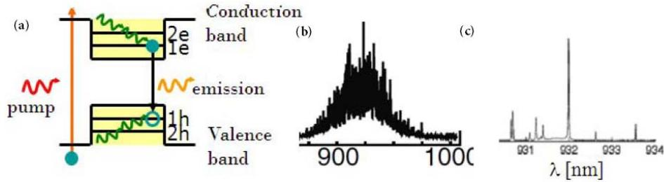
Figure 1.2: (a) The QD energy levels. Difference in bandgap between two materials give rise to the barriers for the electrons and the holes; (b) The inhomogeneous broadening of the quantum dots; (c) Single QD lines: delta function like density of states in quantum dot gives rise to very narrow spectral lines in QD photoluminescence.
