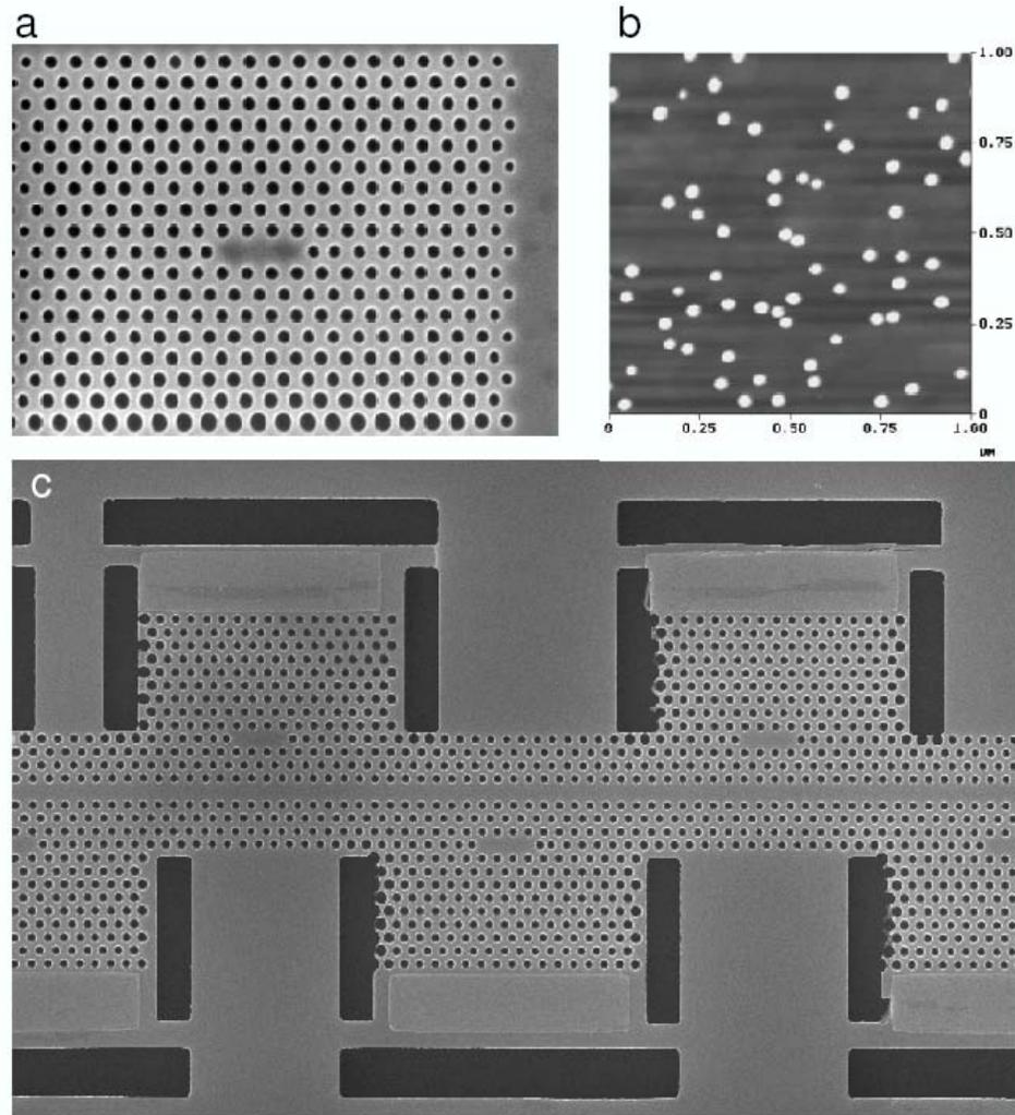
Figure 1.1: (a) Scanning electron microscope image of the fabricated photonic crystal cavity, (b) Atomic Force Microscopy (AFM) image of a  $1\mu m^2$  array of self-assembled InAs/GaAs QDs (courtesy of Bingyang Zhang, Stanford University). (c) Scanning electron micro-graph of a hypothetical integrated nano-photonic structure made of photonic crystal cavities and wave-guides.
