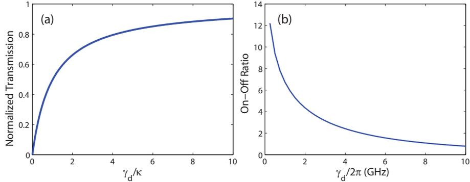
Figure 2.17: (a) Normalized steady state transmission of the laser resonant with the dot (i.e.,  $\Delta\omega_a = 0$ ) with pure dephasing rate  $\gamma_d/2\pi$ . Parameters used are:  $g/2\pi = \kappa/2\pi = 20$  GHz;  $\gamma = \kappa/80$ ; (b) On-off ratio of the modulated signal as a function of the dephasing rate, for  $\kappa/2\pi = g/2\pi = 20$  GHz. The modulation frequency  $\omega_e/2\pi = 5$  GHz and the amplitude of the change in resonance frequency  $\Delta\omega_0/2\pi = 10$  GHz.
