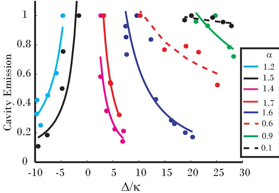
Figure 7.5: Experimentally observed off-resonant cavity emission as a function of the detuning  $\Delta$  between the resonantly driven QD and the cavity. Data are fit with a model  $\Delta^{-\alpha}$ . Extracted values of  $\alpha$  for the different curves are shown.
