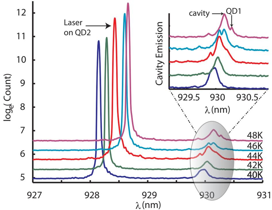
Figure 7.22: Measurement of the emission from the off-resonant cavity and QD1, under resonant excitation of QD2. We observe anti-crossing between QD1 and the cavity when the temperature of the system is changed. Natural log of the count from the spectrometer CCD is plotted. Inset zooms into the cavity emission showing the anti-crossing between the QD1 and the cavity. The plots are vertically offset for clarity.
