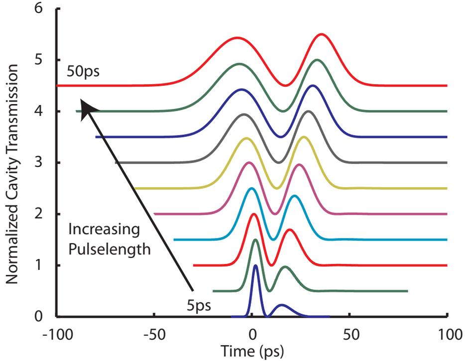
Figure 3.2: The normalized cavity transmission for different pulse duration. The pulse duration is changed from 5 ps to 50 ps. We observe oscillation in the cavity output, although the oscillation frequency decreases with increasing pulse-width. This can be explained by the reduced overlap between the pulse and the coupled dot-cavity system in frequency domain.
