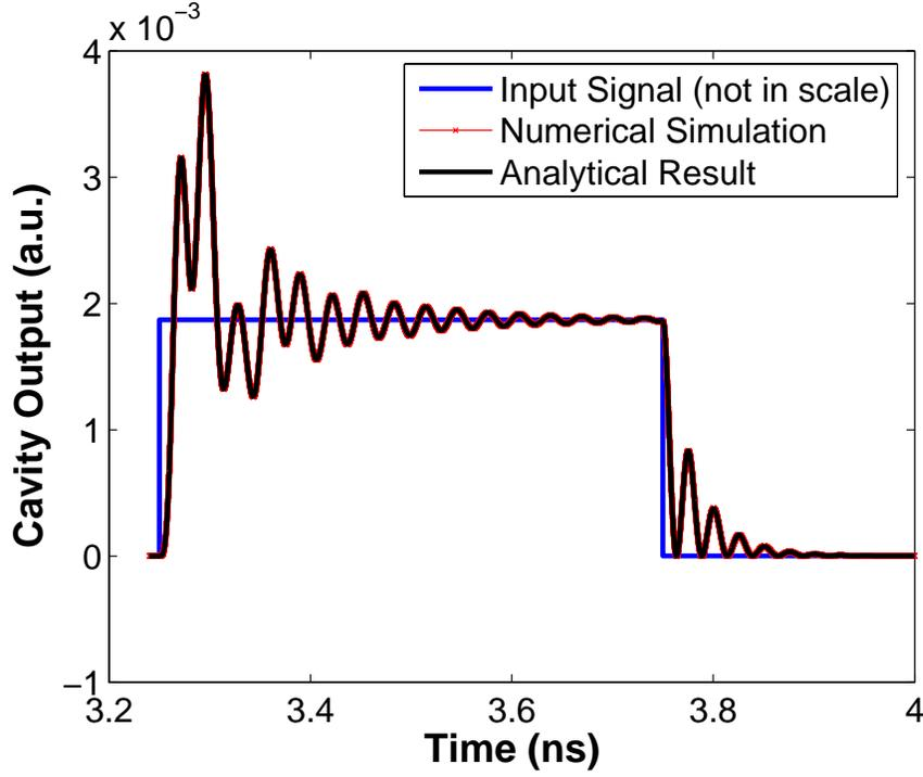
Figure 2.15: Step response of the single QD electro-optic modulator. The parameters used for the simulation are:  $\kappa/2\pi = 5$  GHz;  $g/2\pi = 20$  GHz;  $\Delta\omega_0/2\pi = 20$  GHz;  $\Omega = 1$  GHz.
