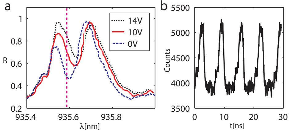
Figure 4.4: Fast electrical switching of a continuous wave laser beam (a) CW reflectivity for bias voltages of 0V, 10V and 14V. During the time-domain switching experiment the laser was set at the wavelength marked by the vertical dashed line and a 0-10V signal was applied. (b) Switching of the coupled laser at the electrical QD driving frequency of 150MHz.
