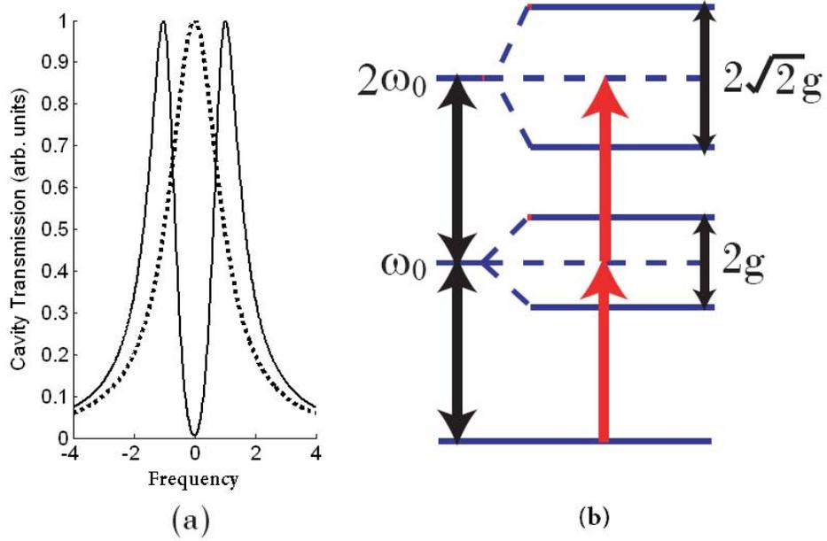
Figure 2.1: (a) The transmission spectrum of a strongly coupled QD-cavity system (split resonance) and an empty cavity (single Lorentzian line); (b) The anharmonic dressed state ladder structure.
