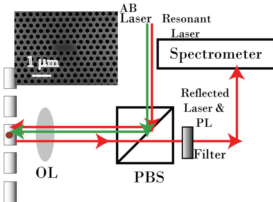
Figure 8.1: The cross-polarized confocal microscopy setup used to probe the coupled QD-cavity system. The inset shows a scanning electron micrograph of the fabricated PC cavity. OL and PBS stand for objective lens and polarizing beam splitter, respectively.
