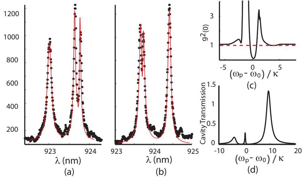
Figure 6.4: QD-photonic molecule spectrum, (a) when the QD is resonant with super-mode sm2 and (b) when the QD is resonant with super-mode sm1. From the fit we extract the system parameters (see text). Numerically simulated (c) second order autocorrelation  $g^2(0)$  and (d) transmission from cavity  $b$ , as a function of laser frequency, with the experimental system parameters that were extracted from the fits.
