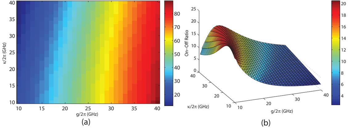
Figure 2.12: (a) Cut-off frequency of the modulator as a function of  $g$  and  $\kappa$ . In the color scheme, the maximum cutoff frequency of  $\sim 90$  GHz is red and the minimum cut-off frequency of  $\sim 10$  GHz is blue; (b) On-off ratio of the modulator at a modulating frequency of  $\omega_e/2\pi = 5$  GHz as a function of  $g$  and  $\kappa$ . For both plots  $\Delta\omega_0/2\pi = 5$  GHz;  $\gamma_d/2\pi = 0.1$  GHz;  $\Omega = 1$  GHz.
