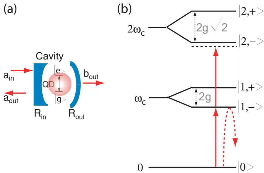
Figure 5.1: (a) Schematic representation of a single emitter coupled to an optical resonator. The optical resonator has mirrors with different reflection coefficients ( $R_{in} \gg R_{out}$ ) such that most of the field coupled into the cavity is emitted at the output port. (b) Schematic representation of the energy eigenstates for a strongly coupled cavity-emitter system.
