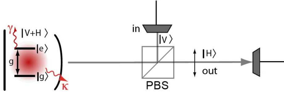
Figure 3.1: Cross-polarized reflectivity setup: the cavity is kept at a  $45^\circ$  angle. The probe light is vertically polarized, but we collect only the horizontal light at the output. Thus we collect only the light which interacted with the cavity, and get rid of the background.
