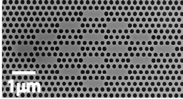
Figure 9.1: SEM of a coupled cavity array in photonic crystal. This particular structure contains 16 cavities.
