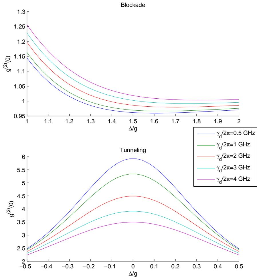
Figure 5.12: The effect of pure QD dephasing on the tunneling and blockade regime: (a) In the blockade regime  $g^{(2)}(0)$  remains lower than 1, but increases with increasing dephasing rate. (b) In the tunneling regime,  $g^{(2)}(0)$  remains higher than 1, but decreases with increasing dephasing rate.
