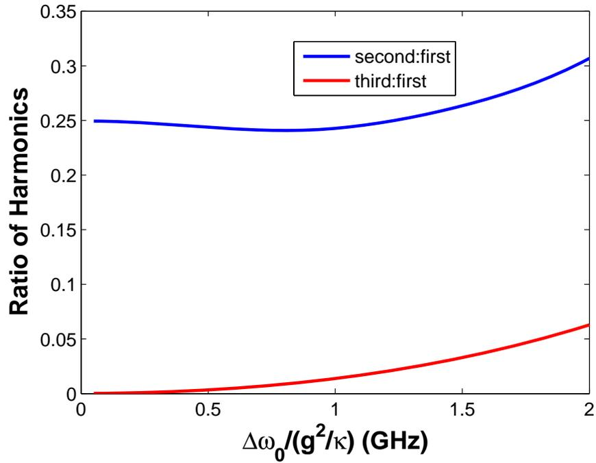
Figure 2.14: Ratio of the second and third harmonic to the first harmonic of the modulated signal, as a function of the maximum frequency shift of the QD, scaled by a factor of  $g^2/\kappa$ . The first harmonic is proportional to the actual signal. For the simulation we assumed that the modulation is working in the passband ( $\omega_e/2\pi = 20$  GHz);  $\kappa/2\pi = g/2\pi = 20$  GHz and the dephasing rate  $\gamma_d/2\pi = 0$ .
