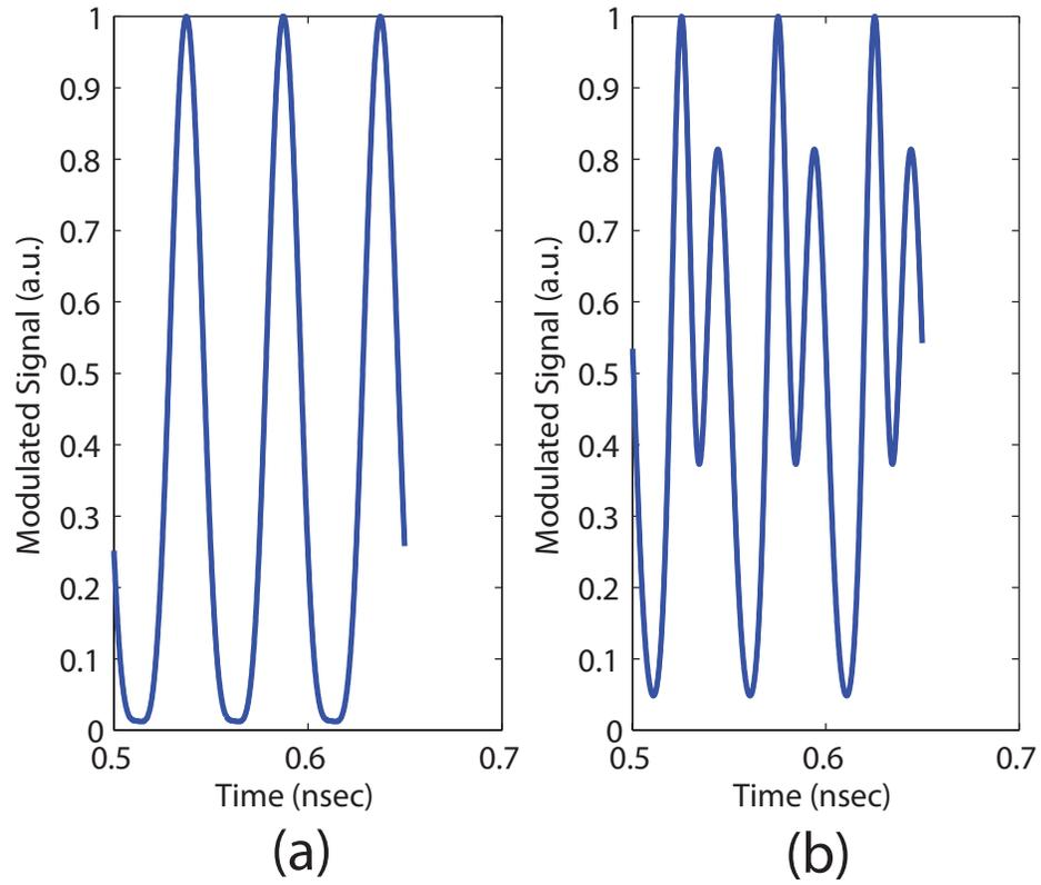
Figure 2.13: Normalized output signal for two different maximal QD detunings  $\Delta\omega_0$ . (a)  $\Delta\omega_0/2\pi = 2$  GHz. (b)  $\Delta\omega_0/2\pi = 40$  GHz. For both simulations the frequency of the electrical signal is  $\omega_e/2\pi = 20$  GHz,  $\kappa/2\pi = g/2\pi = 20$  GHz and  $\Omega = 1$  GHz.
