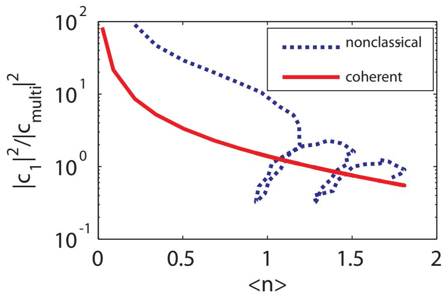
Figure 5.4: Ratio of single photon to multi-photon probability in the output field of the non-classical source with  $\kappa/2\pi = 1\text{GHz}$   $g/2\pi = 40\text{GHz}$  as a function of mean photon number per pulse. The results are compared with a coherent pulsed laser source of the same brightness.
