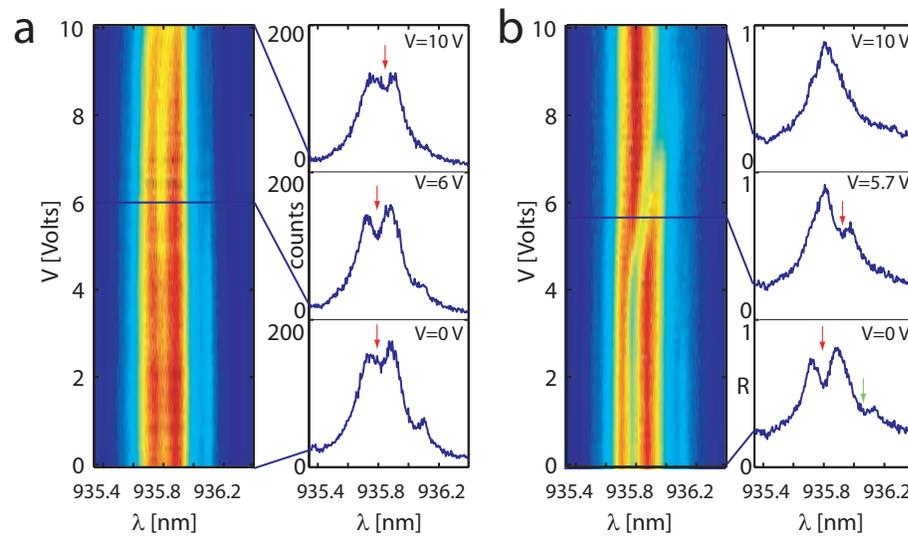
Figure 4.2: (a) Photoluminescence spectra as a function of increasing control voltage ( $V$ ) from 0V to 10V. At 0V the quantum dot was tuned on resonance with the cavity ( $T=48$ K). The PL intensity decreases and the QD red shifts for  $V > 8$ V. The shift is much smaller than the one observed in broadband reflectivity because of the screening induced by free carriers. (b) Broadband reflectivity spectra while changing  $V$  from 0V to 10V ( $T=48$ K). The QD red shifts for  $V > 4$ V.
