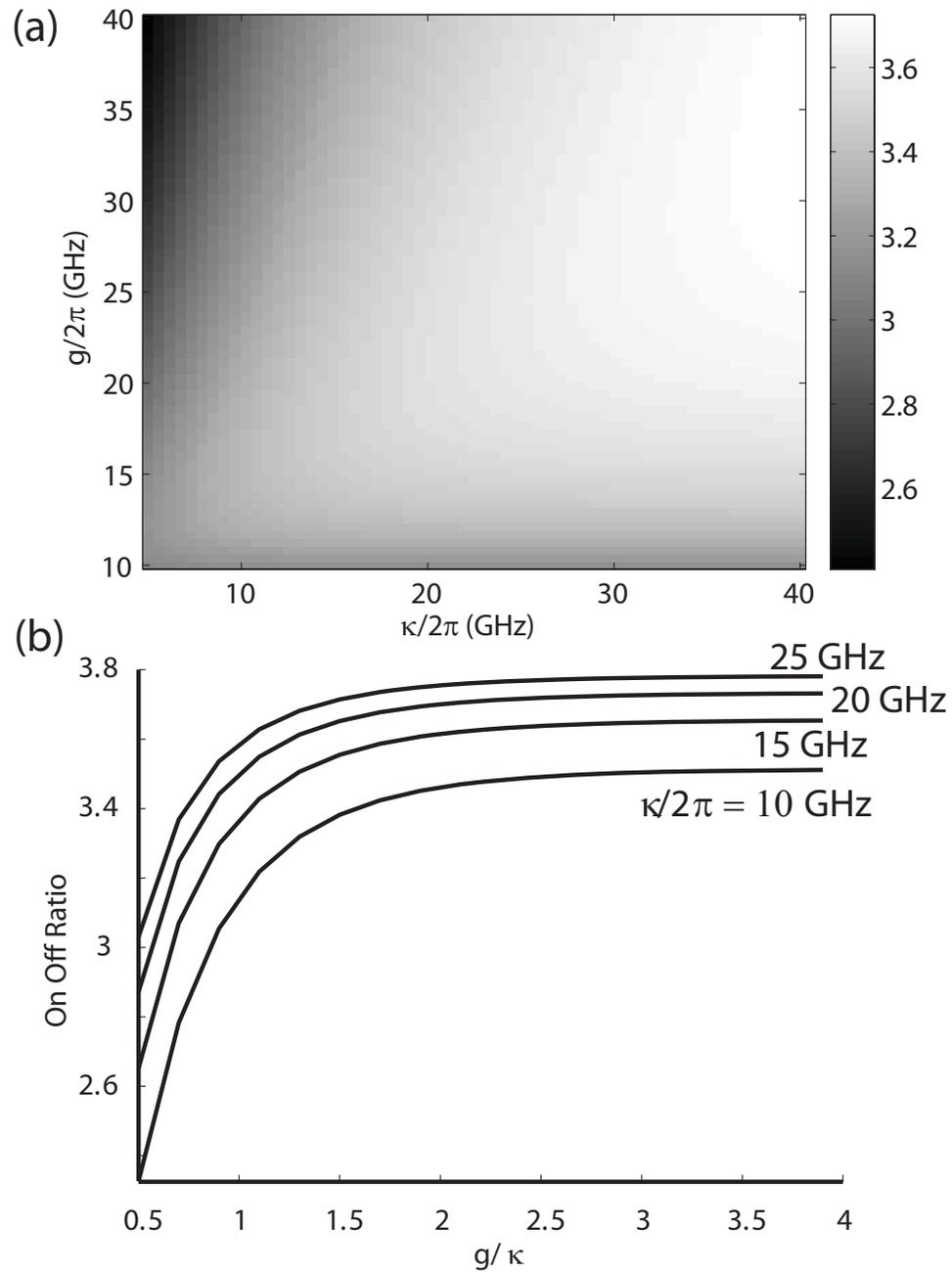
Figure 2.7: (a) Figure showing the on-off ratio (as defined in the text) under CW driving, as a function of  $g$  and  $\kappa$ . (b) On-off ratio as a function of the ratio  $g/\kappa$  for different  $\kappa$ . An increase in on-off ratio is observed with increase in both  $g$  and  $\kappa$ . For, this simulation  $\mathcal{E}/2\pi = 0.1$  GHz.
