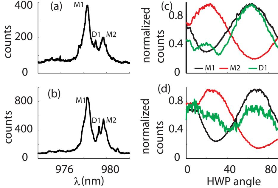
Figure 5.20: (a), (b) PL spectrum of the bimodal (H2) cavity and a coupled QD at two different temperatures 20K (a) and 30K (b). The two modes are denoted as M1 and M2 and the QD is denoted as D1. (c),(d) Polarization dependence of the cavity modes (red and black plots) and the QD (green plot) at two different temperatures: 20K (a) and 30K (b).
