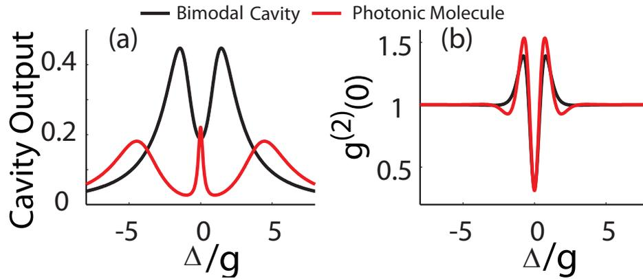
Figure 6.5: (a) Cavity transmission for two cases: bimodal cavity and photonic molecule. (b) Second order autocorrelation  $g^{(2)}(0)$  for these two cases. Parameters used for the simulations: QD-cavity interaction strengths  $g/2\pi = g_a/2\pi = g_b/2\pi = 10$  GHz; cavity field decay rates  $\kappa_a/2\pi = \kappa_b/2\pi = 20$  GHz; coupling strength for the photonic molecule  $J/2\pi = 40$  GHz; dipole decay rate  $\gamma/2\pi = 1$  GHz.
