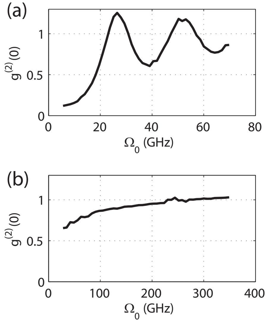
Figure 5.3: (a) Second order correlation correlation function of the output field, for the case  $\kappa/2\pi = 1\text{GHz}$ ,  $g/2\pi = 40\text{GHz}$ . (b) Second order correlation correlation function for  $\kappa/2\pi = 5\text{GHz}$ ,  $g/2\pi = 30\text{GHz}$ .
