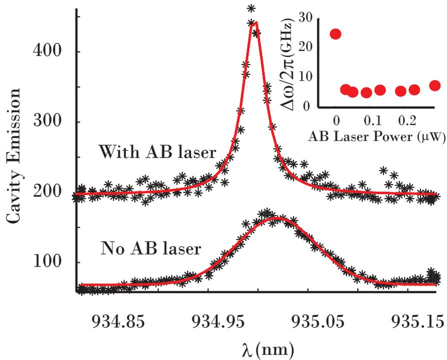
Figure 8.4: Effect of the AB laser on the QD spectrum as measured through off-resonant cavity emission. In the absence of the AB laser, we observe a broad QD linewidth. However, in the presence of this laser, a significant linewidth narrowing is observed. The increased background with the AB laser on is caused by the PL generated by the AB laser. The inset shows the QD linewidth measured as a function of the AB laser power.
