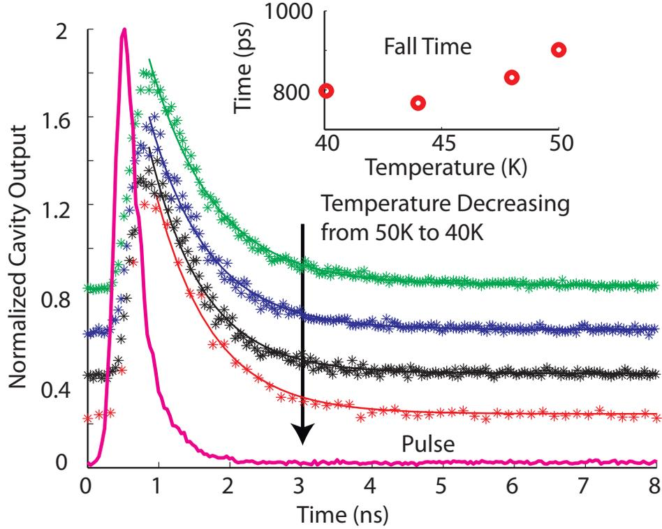
Figure 7.19: Time resolved measurement of the off-resonant cavity emission. The QD is resonantly excited with a 40 ps pulse, and the time-resolved measurement of the higher energy off-resonant cavity emission is performed. The inset plots the fall times of the cavity emission (extracted from the exponential fits) against the system’s temperature.
