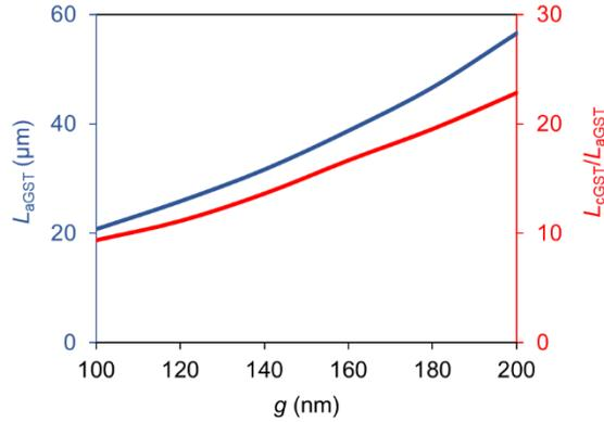
Figure 4.7. Trade-off between  $L_{\text{aGST}}$  and  $L_{\text{cGST}}/L_{\text{aGST}}$  by varying the gap.
