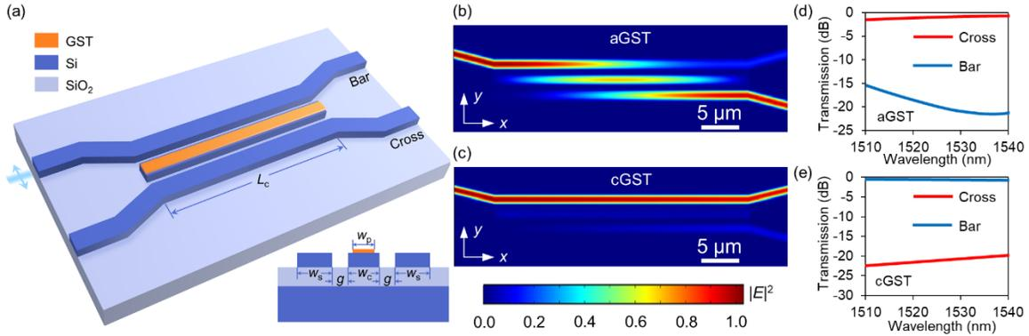
Figure 4.5. Simulation of the  $2 \times 2$  DC switch. (a) Schematic of the switch. (b,c) Normalized optical field intensity distribution in the device for (b) aGST and (c) cGST simulated at 1550 nm. (d,e) Calculated transmission spectra at the cross and bar ports for (d) aGST and (e) cGST.
