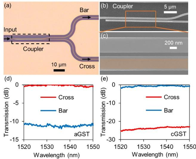
Figure 4.4. Experimental results of the  $1 \times 2$  DC switch. (a) Optical microscope image of the fabricated switch. (b) SEM image of the switch. (c) An enlarged view of the coupling region highlighted by the orange rectangle in (b) with the GST false-colored. (d-e) Measured transmission at the cross and bar ports with the GST in the (d) amorphous and (e) crystalline states.
