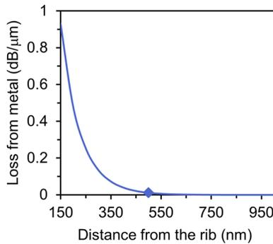
Figure 5.4. Additional loss introduced from metal contacts as a function of the distance between the edges of the electrodes and the rib waveguide. The marked dot corresponds to the adopted distance in the main text.
