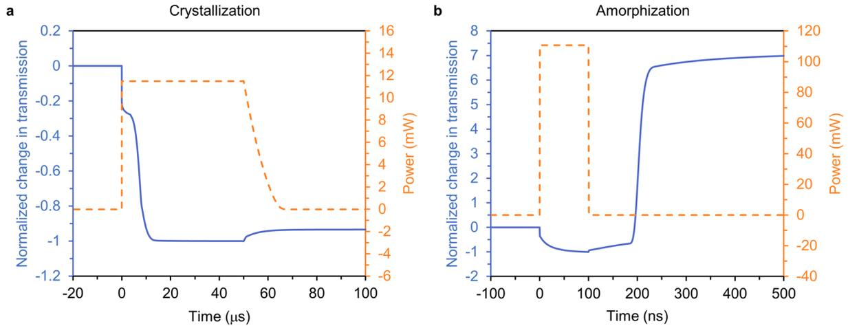
Figure 6.4. Real-time optical transmission during Set and Reset processes. (a,b) real-time power of the applied electrical pulse (dashed line, same as in Figure 6.3) and corresponding normalized change in optical transmission of the simulated switching unit at 1550 nm (solid line) for crystallization (Set, a) and amorphization (Reset, b). Here, the length of the switching unit is  $5\ \mu\text{m}$  and the thickness of the GST is 10 nm.
