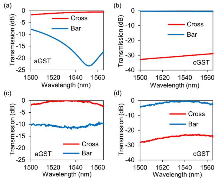
Figure 4.9. Full wavelength range transmission spectra of the  $1 \times 2$  DC switch at the cross and bar ports for (a,b) simulations and (c,d) experiments.
