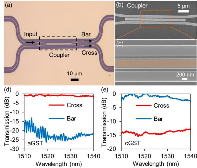
Figure 4.8. Experimental results of the  $2 \times 2$  DC switch. (a) Optical microscope image of the fabricated switch. (b) SEM image of the switch. (c) An enlarged view of the coupling region highlighted by the orange rectangle in (b) with the GST false-colored. (d,e) Measured transmission at the cross and bar ports with the GST in the (d) amorphous and (e) crystalline states.
