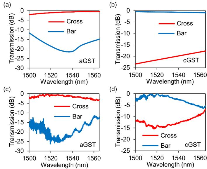
Figure 4.10. Full wavelength range transmission spectra of the  $2 \times 2$  DC switch at the cross and bar ports for (a,b) simulations and (c,d) experiments.
