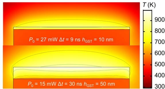
Figure 5.7. Temperature distribution at the end of a pulse indicating re-amorphization during the crystallization process due to much too high power (upper panel,  $P_0 = 27$  mW,  $\Delta t = 9$  ns,  $h_{\text{GST}} = 10$  nm) and large GST thickness (lower panel,  $P_0 = 15$  mW,  $\Delta t = 30$  ns,  $h_{\text{GST}} = 50$  nm). The red (green) lines denote the contour of  $T = 723$  K ( $T = 883$  K) for the crystallization (re-amorphization) boundary.
