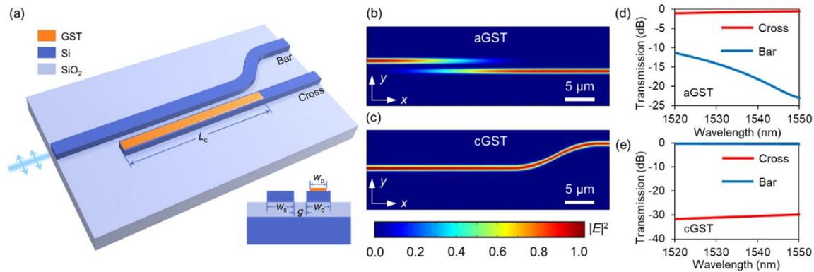
Figure 4.1. Simulation of the  $1 \times 2$  DC switch. (a) Schematic of the switch. (b,c) Normalized optical field intensity distribution of the switch for (b) aGST and (c) cGST simulated at 1550 nm. (d,e) Calculated transmission spectra at the cross and bar ports for (d) aGST and (e) cGST.
