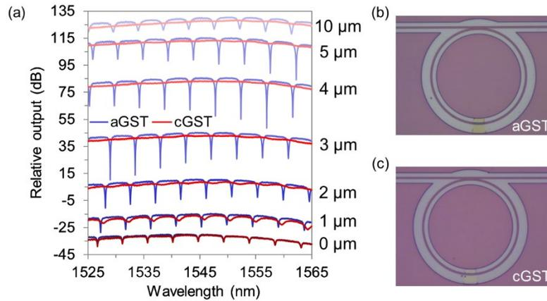
Figure 2.3. Transmission measurement of the microrings with GST. (a) Representative output spectra of microrings with different length of GST for amorphous and crystalline states. For each length of GST, the cGST and aGST spectra are in scale, while each set of spectra for a different length of GST is offset vertically for clarity. (b,c) Microscope images of a microring with 5  $\mu\text{m}$  (b) aGST and (c) cGST.
