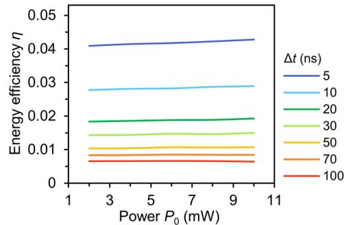
Figure 5.12. Power-dependent energy efficiency for different pulse widths. The pulse power is selected to be low enough in order to heat the aGST without inducing any phase transition.
