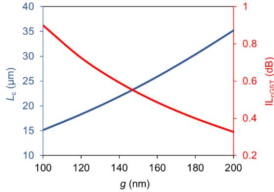
Figure 4.3. Trade-off between the coupling length for the maximum transmission in the amorphous state and insertion loss in the crystalline state by varying the gap.
