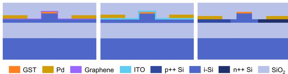
Figure 5.13. Cross-section schematics of the PINCs with graphene, ITO, and PIN diode heaters. p++ (n++), heavily doped p (n)-type silicon region. i, intrinsic silicon region.
