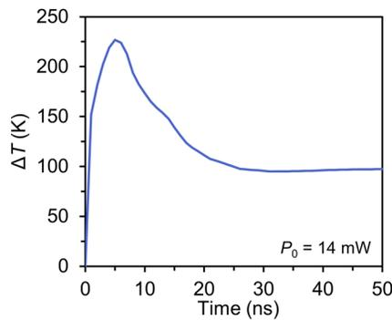
Figure 5.6. Real-time temperature gradient during the crystallization process ( $P_0 = 14$  mW,  $\Delta t = 50$  ns).
