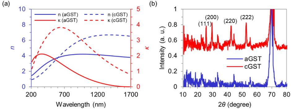
Figure 2.1. GST characterization. (a) Complex refractive index of aGST and cGST as a function of wavelength. (b) XRD data of aGST and cGST. The curve of cGST is offset vertically for clarity.
