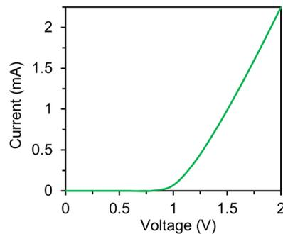
Figure 5.14. Current-voltage (I-V) curve of the silicon PIN diode.
