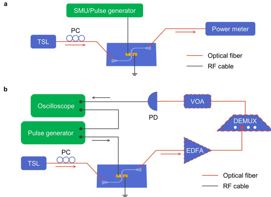
Figure 6.2. Experimental setups. (a) Setup for static measurement. (b) Setup for transient response measurement. The tools framed with dashed red lines were used for measuring the pulse width modulation (PWM) effects. TSL, tunable laser. PC, polarization controller. SMU, source meter unit. EDFA, erbium-doped fiber amplifier. DEMUX, optical demultiplexer. VOA, variable optical attenuator. PD, photodiode.
