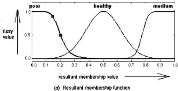
Figure 3. Membership functions for fuzzy calculation.
