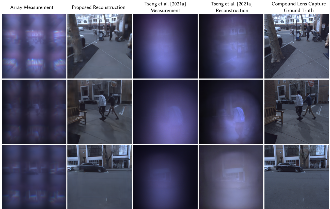
Fig. 11. Experimental evaluation of the proposed thin nanophotonic camera on broadband outdoor scenes. The proposed nanophotonic array optic with the probabilistic deconvolution method reconstructs the underlying latent image robustly in broadband lit environments, outperforming Tseng et al. [2021a] significantly in outdoor scenes. See Supplemental Material for lab captures acquired of a narrow-band screen where the proposed design and Tseng et. al both function adequately.
